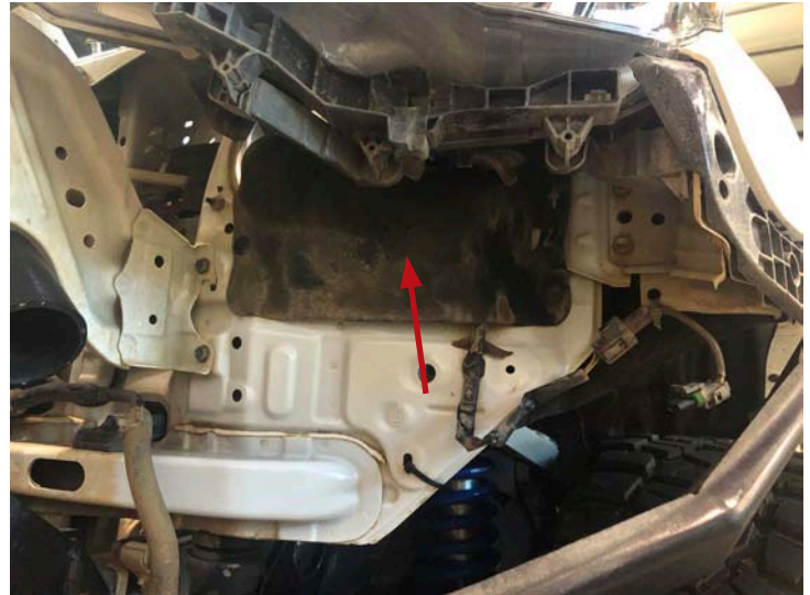
Remove Rubber Panel
