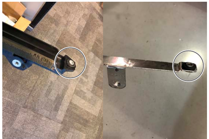
Radiator Bracket Isolator
