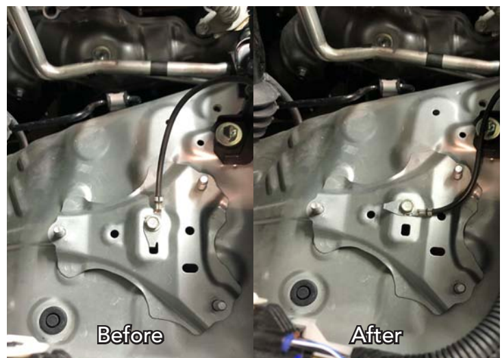
Ground Wire Rotated
