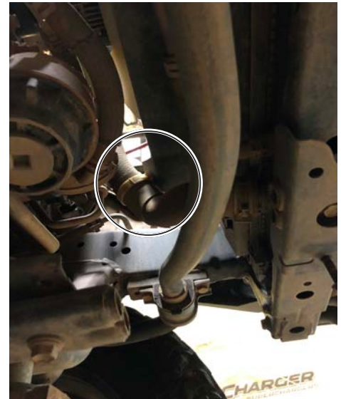
Unhook Retaining Clip
