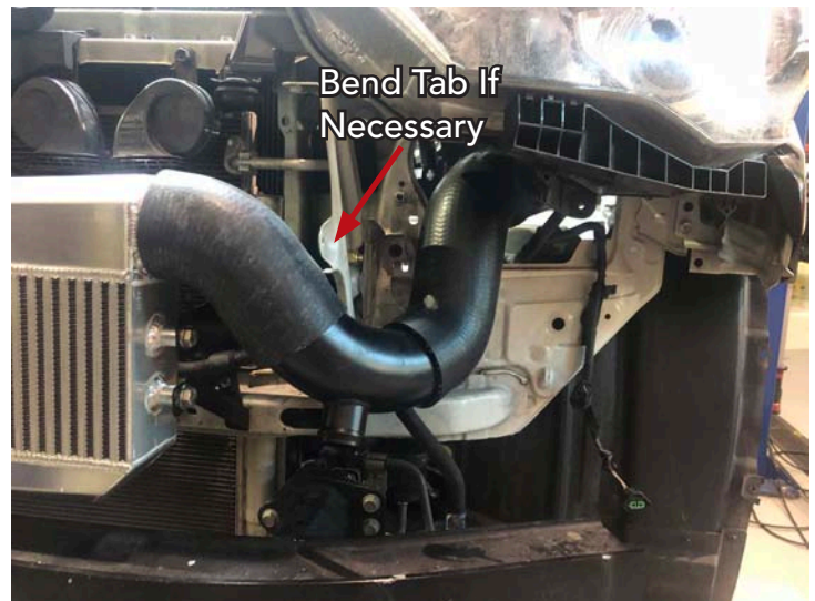
Tubing To Intercooler
