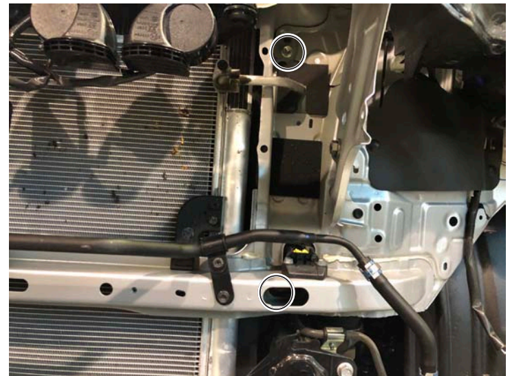
Radiator Bracket Front Bolts
