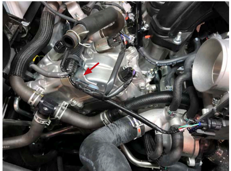
Remove Metal Bracket
