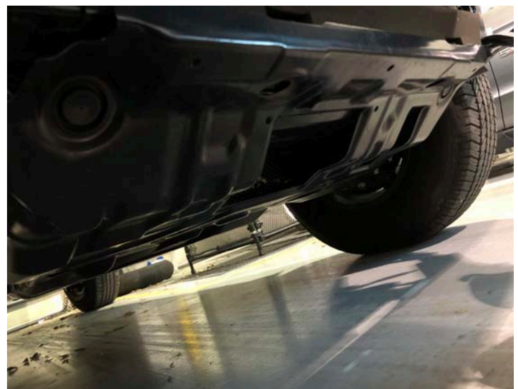
Remove Skid Plate
