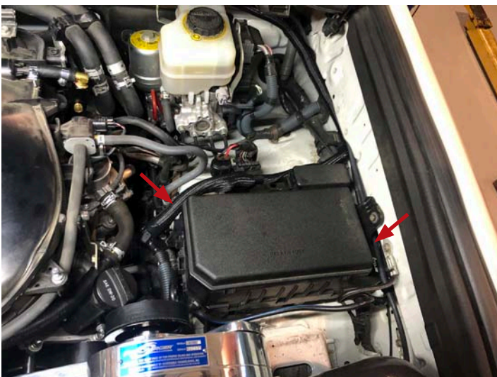
Route Cables Behind Fuse Box
