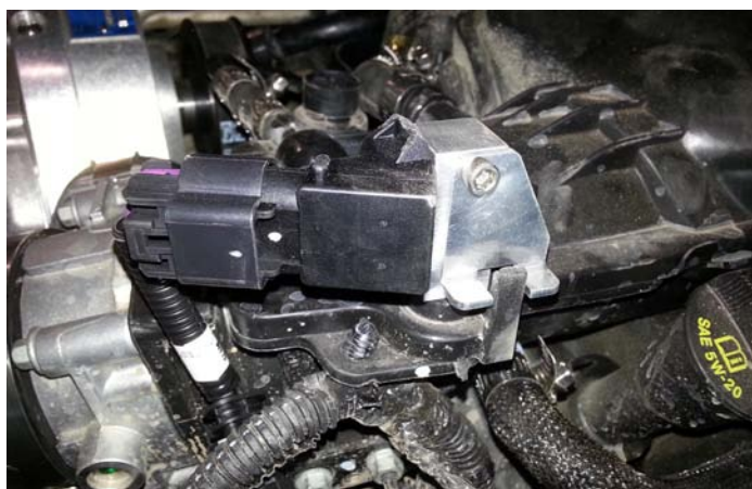
MAP sensor Installed
