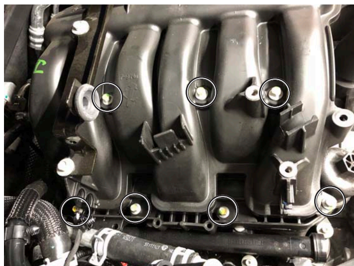
Remove Bolts (7 of 8 Shown)
