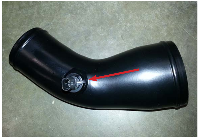
IAT Sensor Lock Tab Direction
