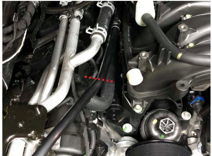
Cut PCV Line At The Dotted Line
