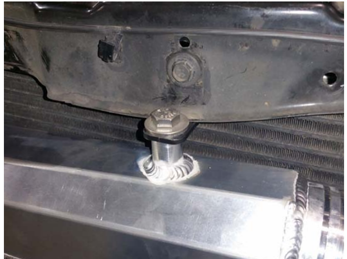
Driver's Side Intercooler Mounted
