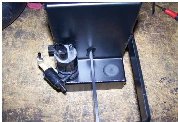
Washer Tank With Pump And Plug 2012-13 (Shown Without the Pump Hold down)
