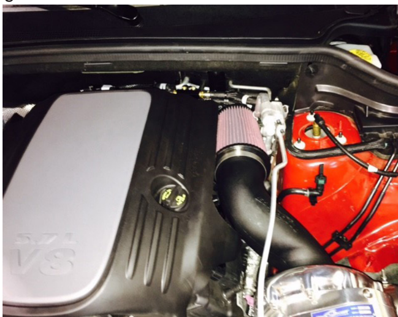
Air Inlet Installed
