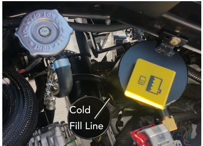
Coolant Tank Installed
