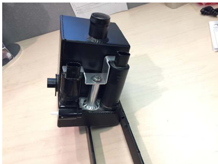
Washer Tank With Pumps And Hold Down Installed 2014+
