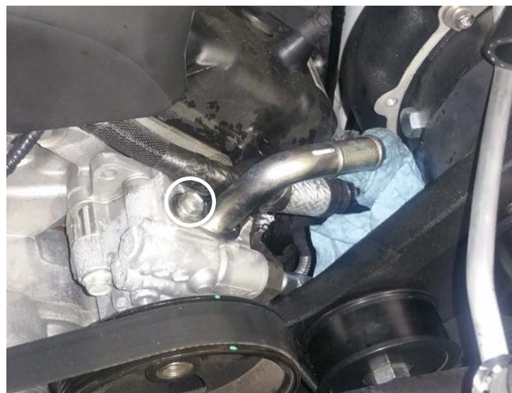
Power Steering Line Removal
