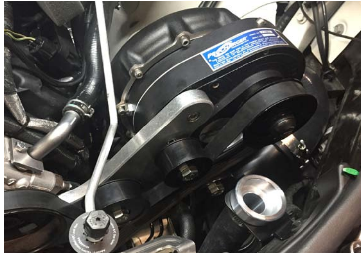
Procharger Head Unit Installed
