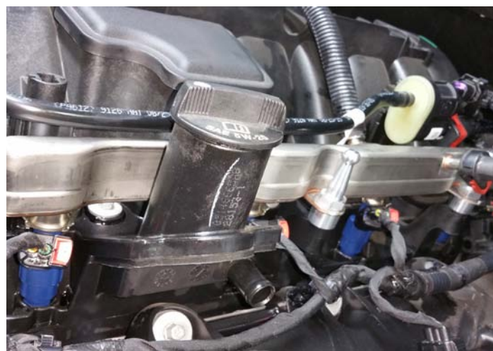
Fuel Rails Installed
