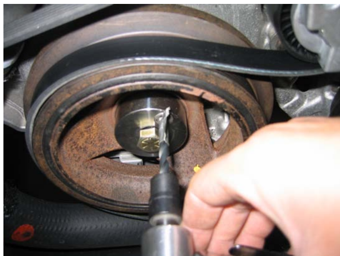
Drilling the Crank
