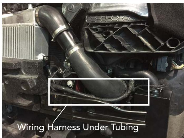
Tubing To Intercooler Installed
