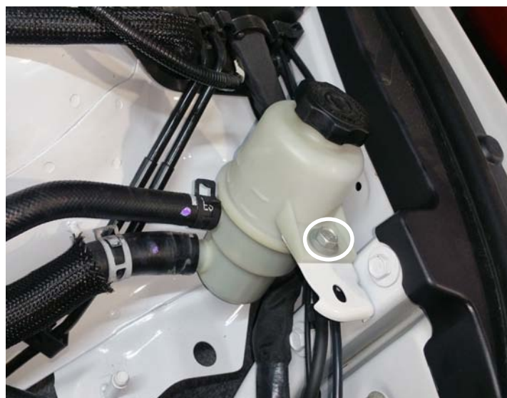
Remove Power Steering Reservoir
