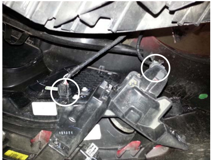
Fog Light & Turn Signal Connectors (Drivers)
