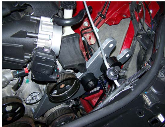
Main Bracket Installed
