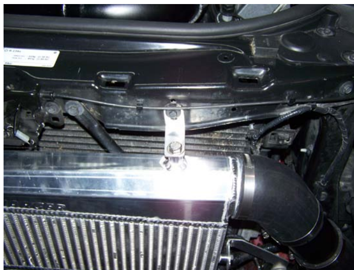
Driver's Side Intercooler Mounted
