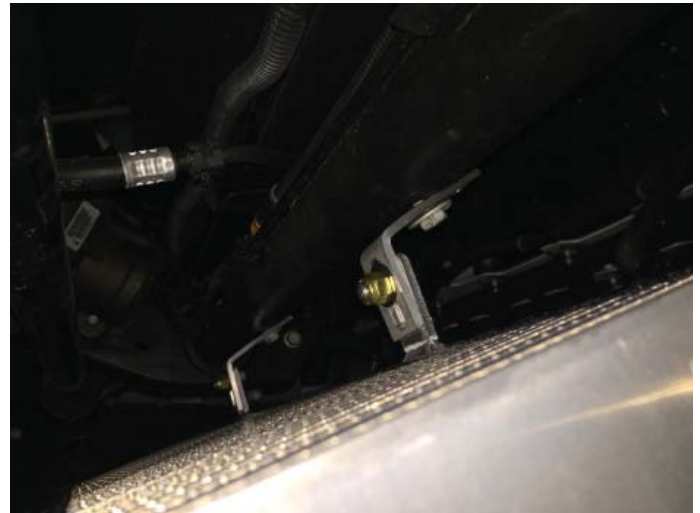
Front Of Intercooler Mounted
