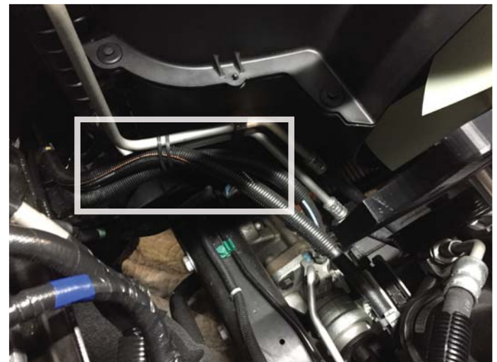
Power Steering Lines Moved
