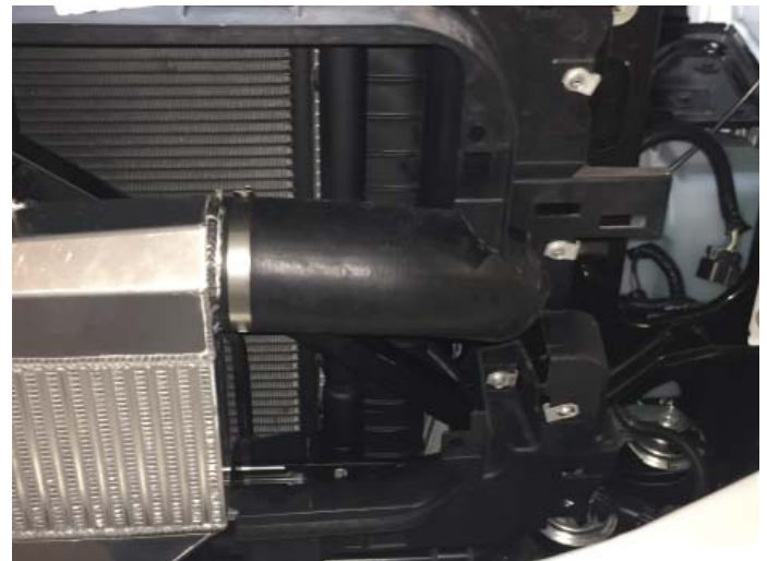
Tubing To Intercooler
