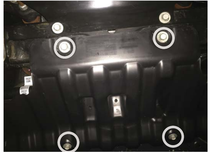
Remove Plastic Skid Guard
