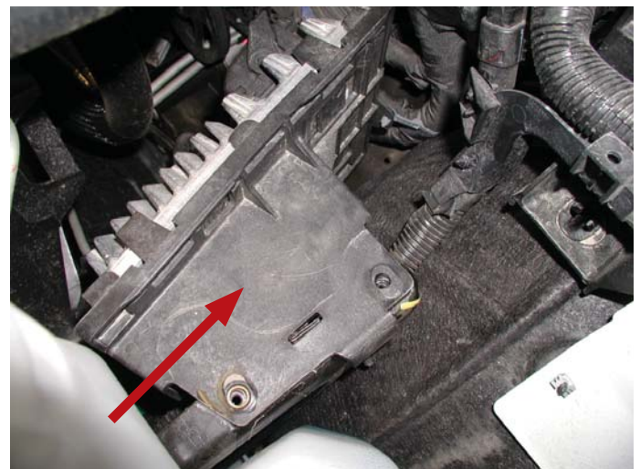
ECU Bracket Removal
