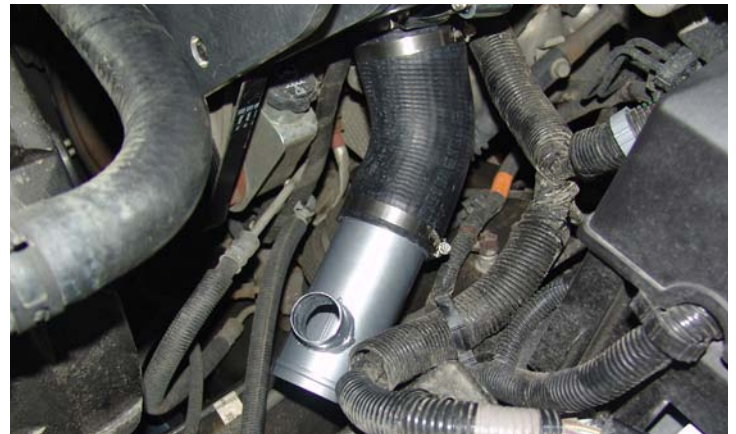
Rubber 45° Elbow With Bypass Tube
