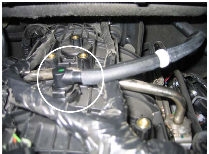
Intake Manifold PCV Line O-Ring Seal
