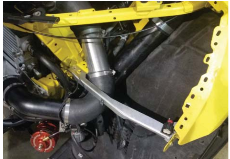
Install New Fender Brace
