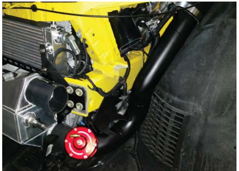
Blower Outlet Tube Installed
