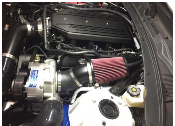
F1A-94 Air Inlet Installed
