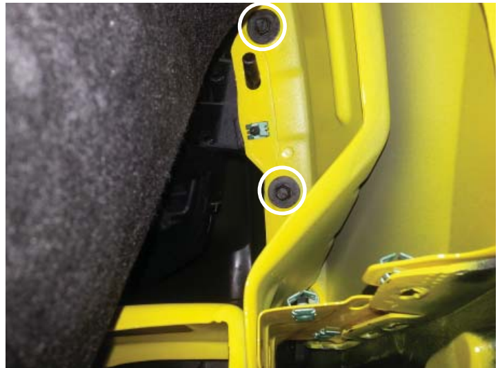
Screws Behind Wheel Liner (Lower Two Shown)
