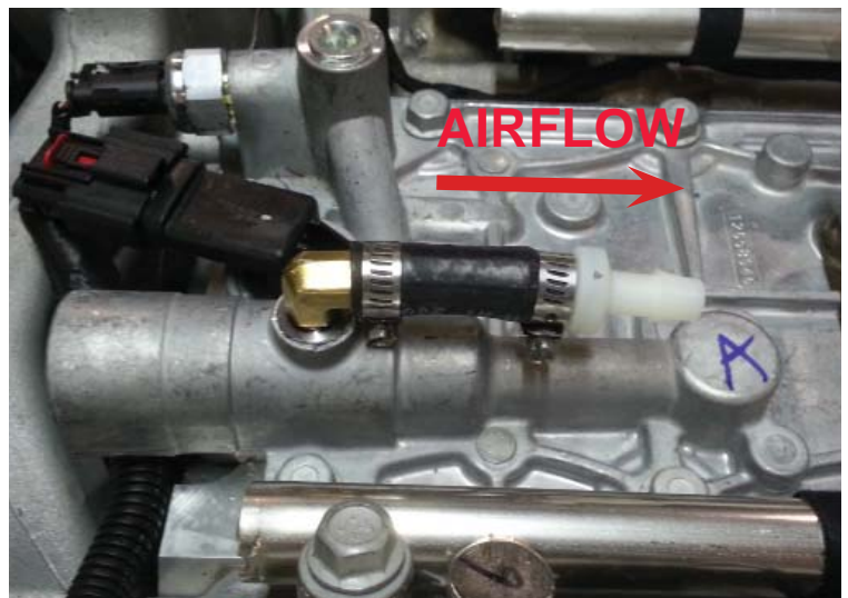
Check Valve Installed
