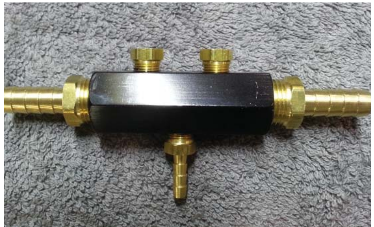
Vacuum Manifold Assembled
