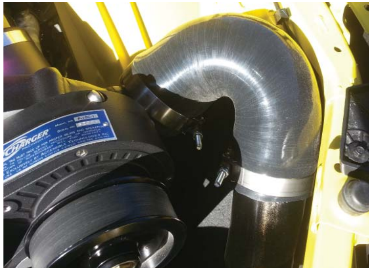
Blower Discharge Tube Installed
