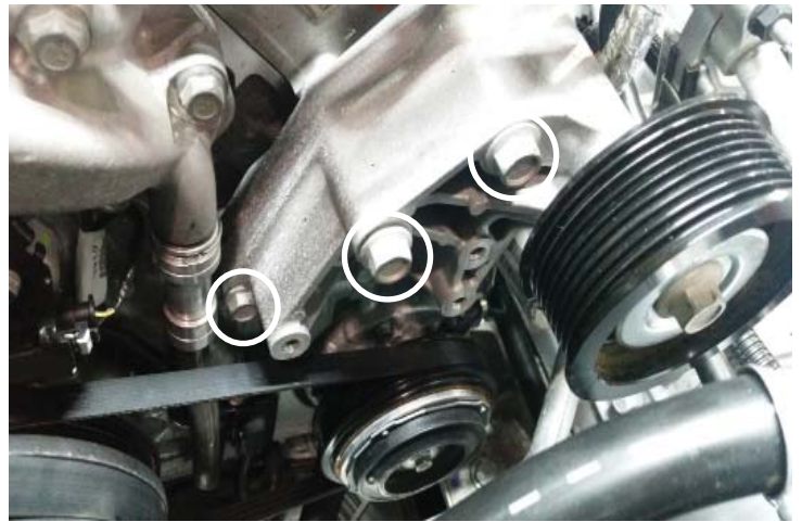
Tensioner Bracket Bolts (3 of 4 shown)
