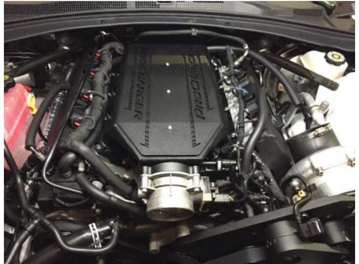
Intake Manifold Installed
