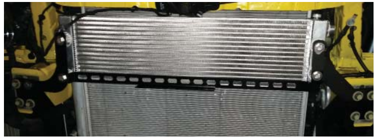
Heat Exchanger Mounted
