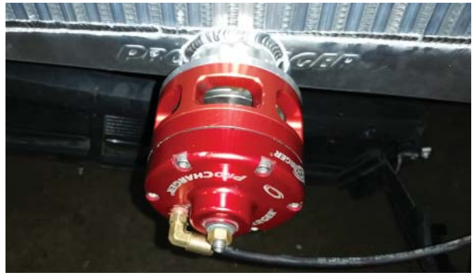
Race Valve Installed
