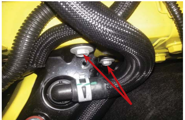
Upper Aux. Heat Exchanger Bolts
