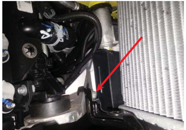
Lower Aux. Heat Exchanger Bracket Bolt
