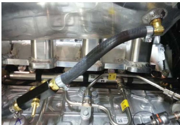
Vacuum Manifold Connected to Intake
