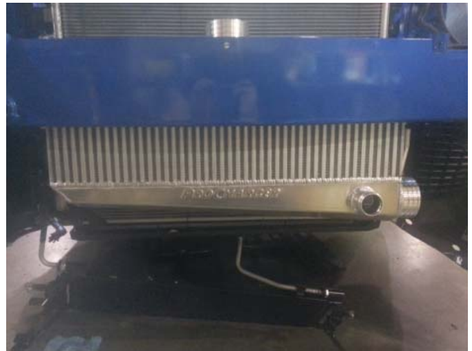
Stage 2 Intercooler Installed
