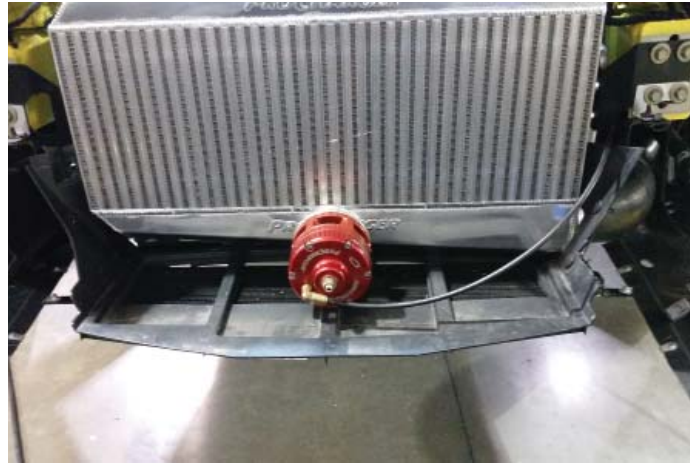
Modified Air Shroud Installed
