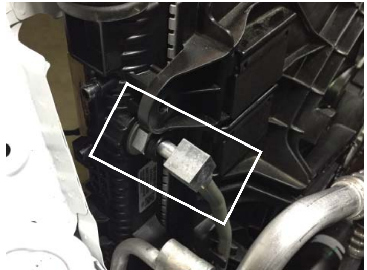
Transmission cooler line.
