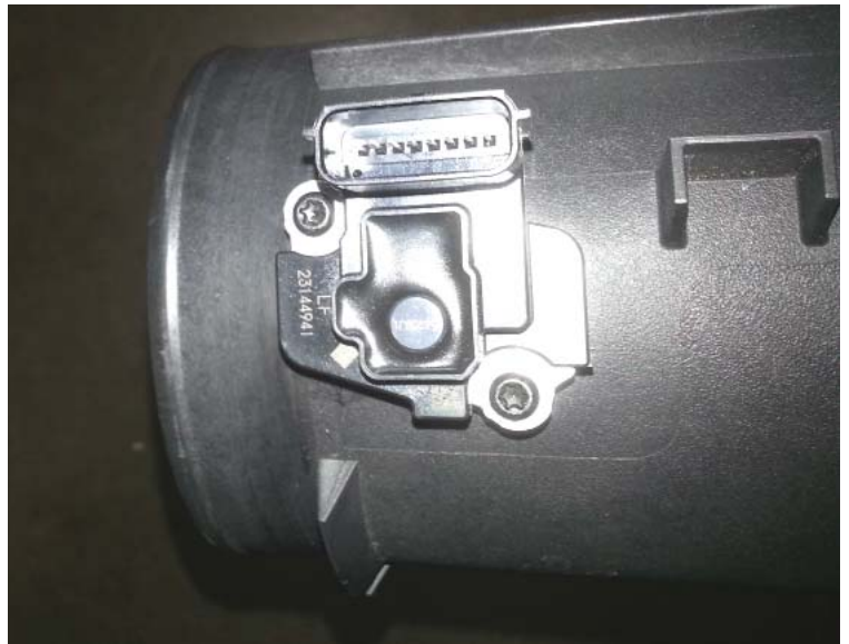
Remove MAF Sensor from Factory Air Box
