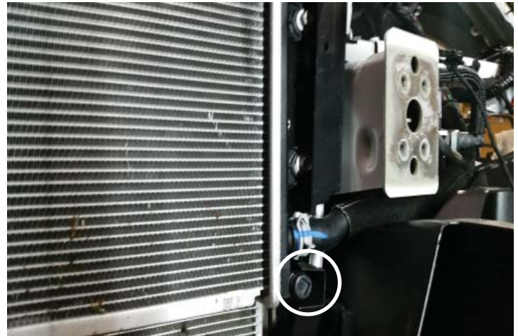
Heat Exchanger Drain
