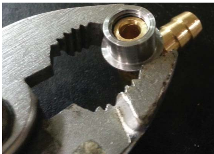
Adapter Fitting Installed on Barb Fitting
