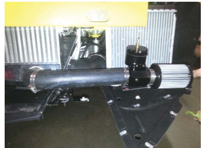
Surge Valve Installed
