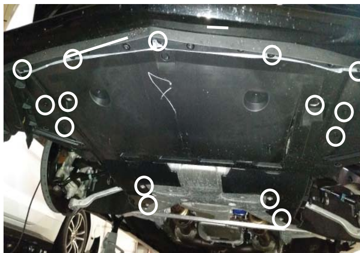
Plastic Splash Panel Screws and Bolts
