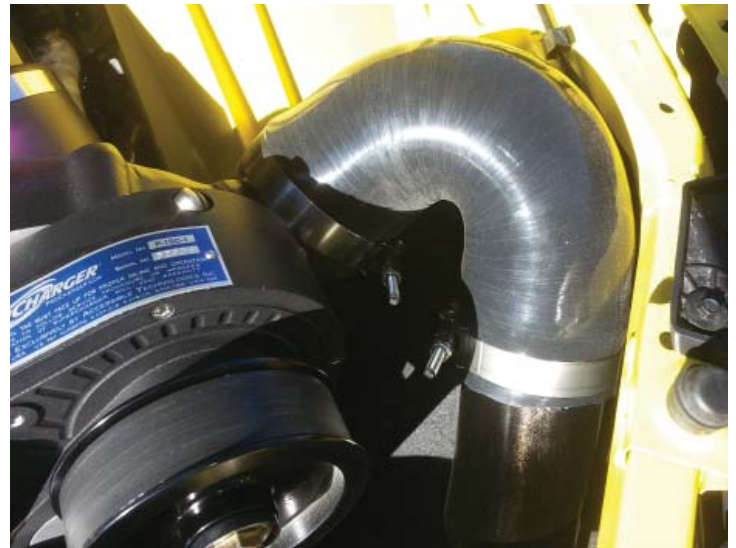
Blower Discharge Tube Installed
