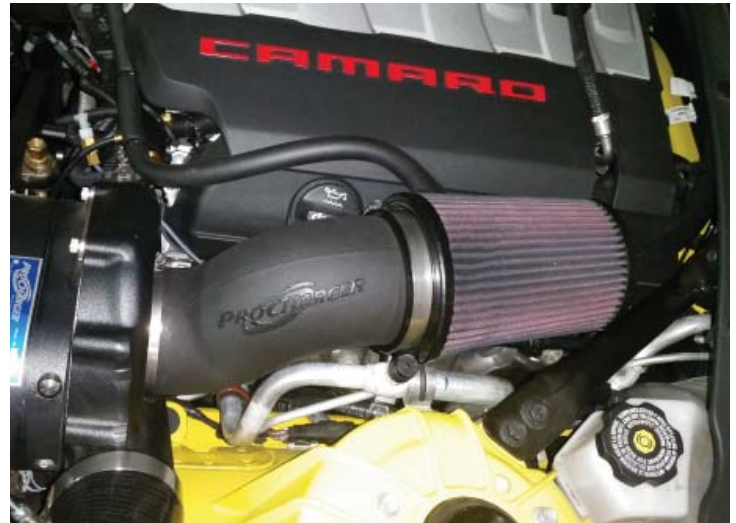
Air Inlet Installed
