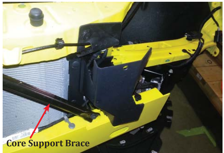
Remove Plastic Covers (Driver's Side)
