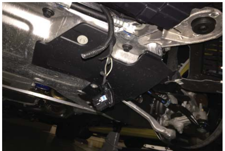
Intercooler Pump Wiring
