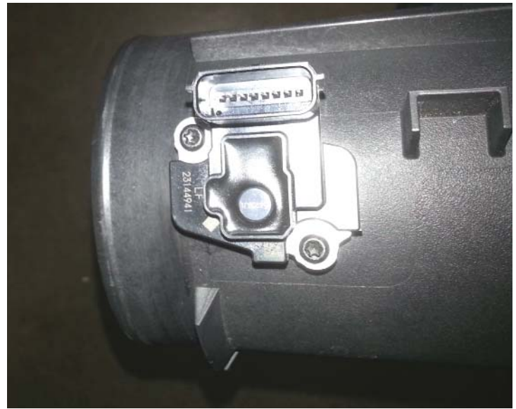
Remove MAF Sensor from Factory Air Box
