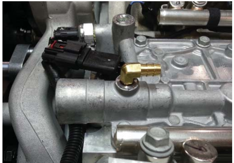
Barb Fitting Installed In Valley Cover
