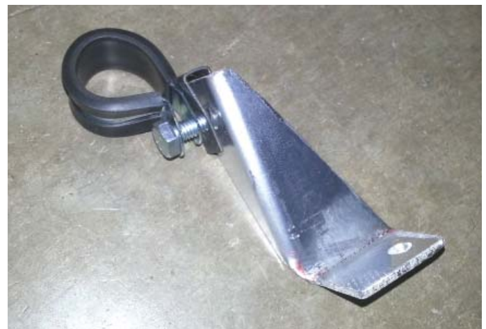
Assembled A/C Line Bracket
