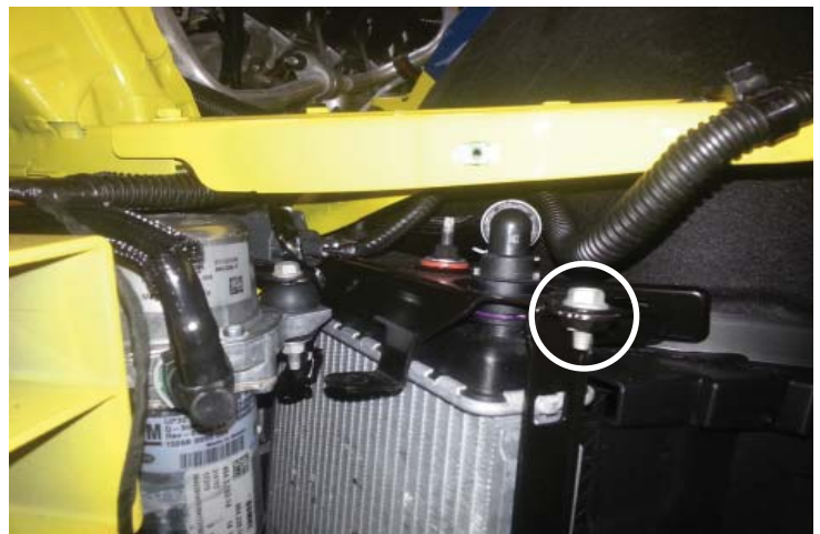
Aux. Heat Exchanger Bracket Bolts
