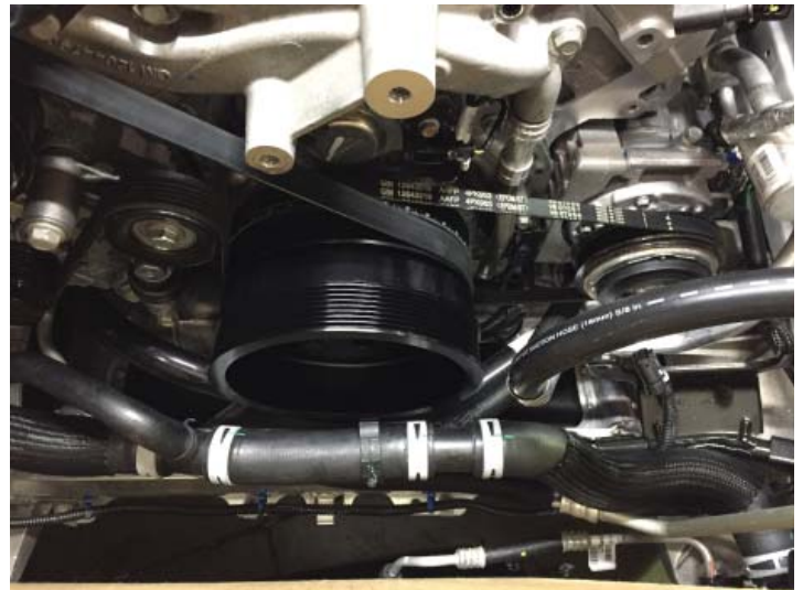
Crank Pulley Installed
