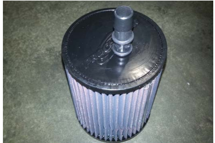
Plastic Fitting Installed in Air Filter
