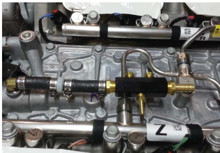
Vacuum Manifold Installed
