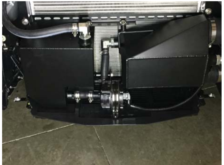
Modified Air Shroud Installed
