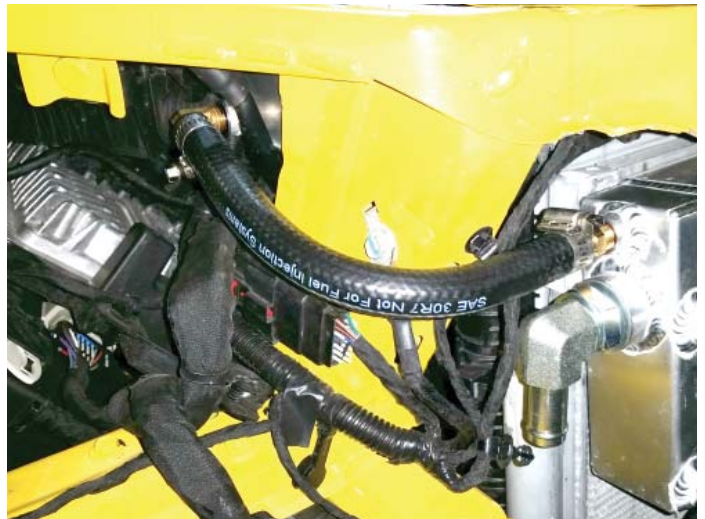
Fill Tank Hose Connected
