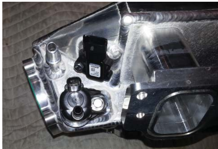
EVAP, MAP and Throttle Body O-ring Installed
