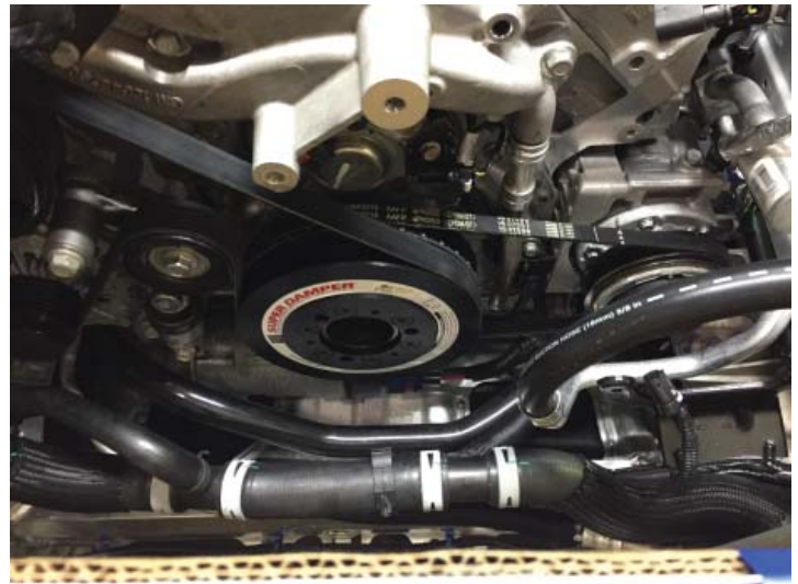
ATI Balancer Installed
