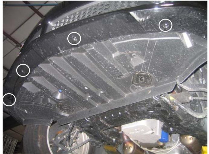
Remove (4) Bolts With 7mm Socket
