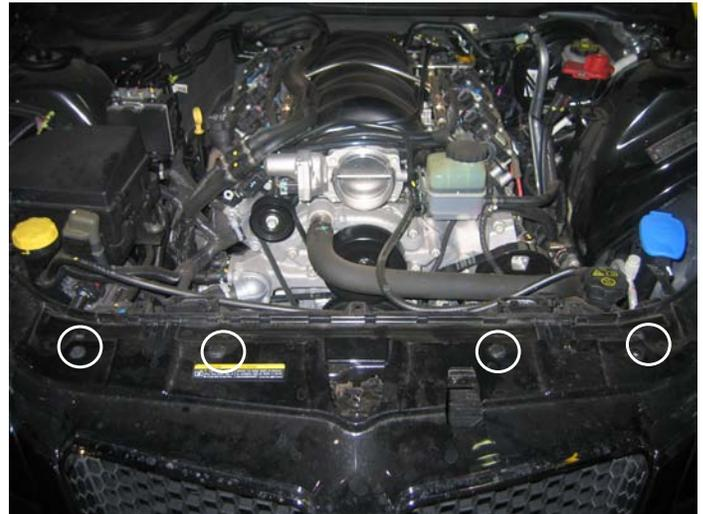
Remove (2) Bolts With 10mm Socket and (2) Push Pins
