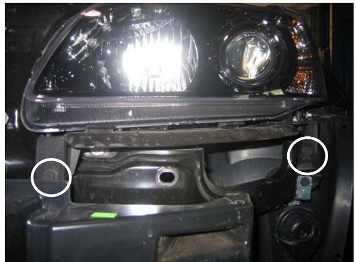
Driver's Side Headlight Shrouding Fasteners
