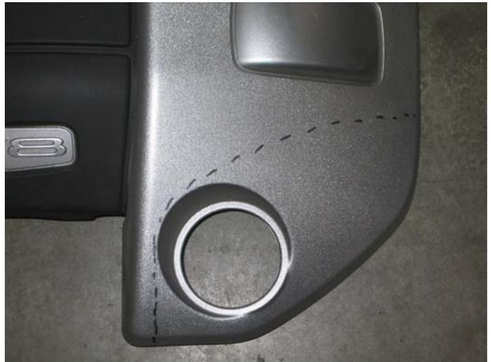
Engine Cover Trimming Guide Lines
