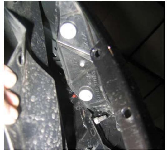
Passenger's Side Fascia to Fender Fasteners
