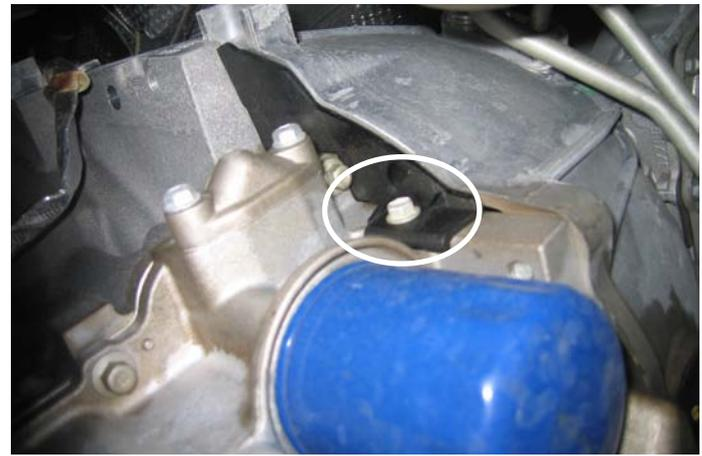
Transmission Access Shield and Hardware
