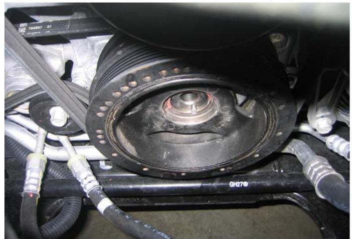
Crank Pulley Bolt Removed
