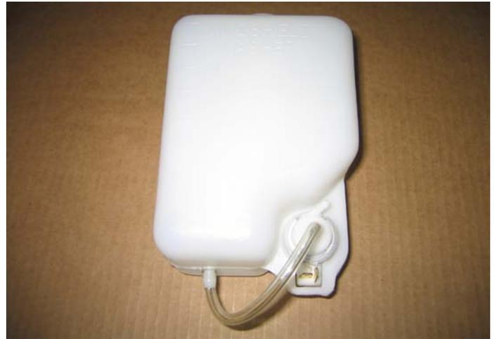
Tube Routing From Reservoir to Washer Motor
