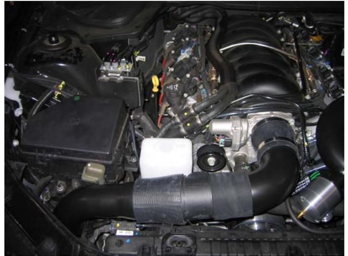
Upper Passenger's Side I/C Tubing Installed
