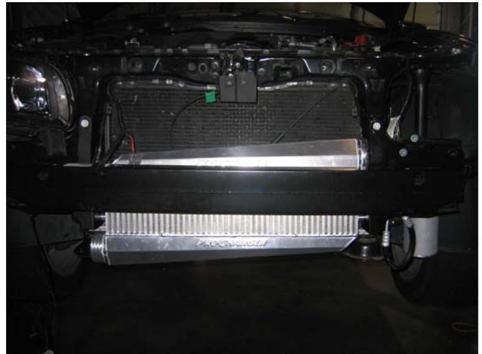
Intercooler Installed (3 Core I/C Shown)
