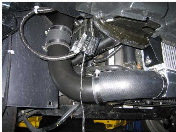
Lower Passenger's Side I/C Tubing Installed
