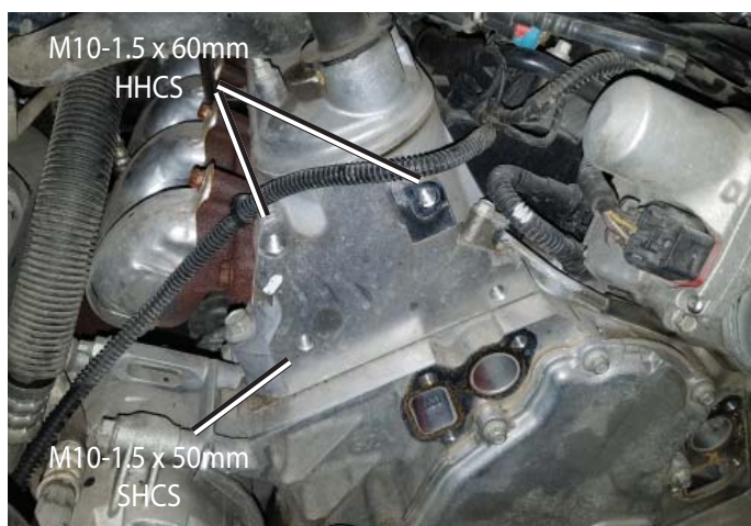
Sub-Bracket Mounting Locations
