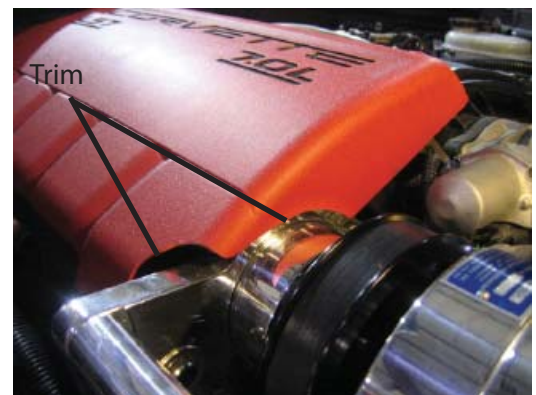
Passenger's Side Engine Cover
