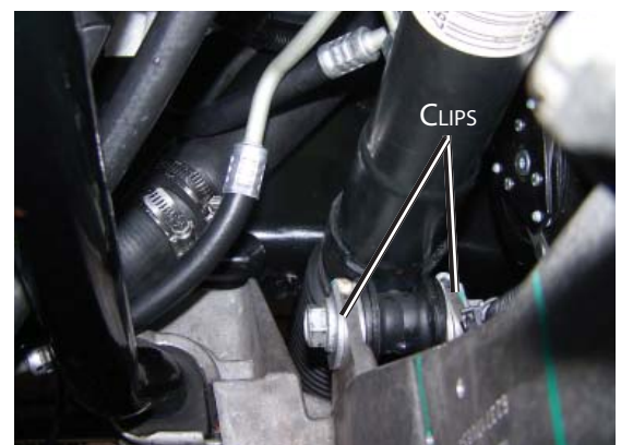
Passenger's Side Rack Mount
