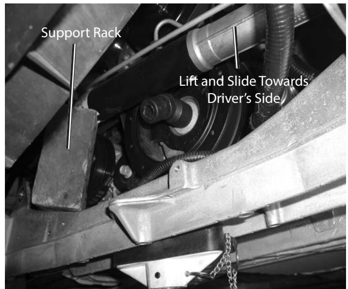
Rack Relocated for Balancer Bolt Removal
