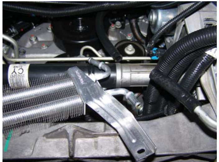
Factory Power Steering Cooler Removal
