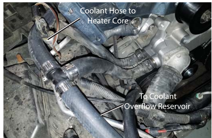
Supplied Tee Installed
