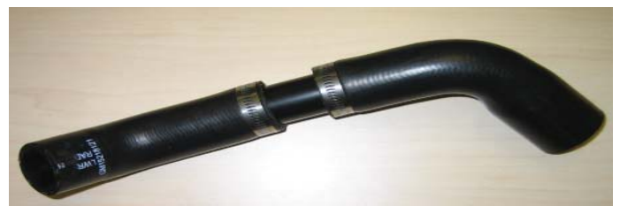
Lower Radiator Hose Modified
