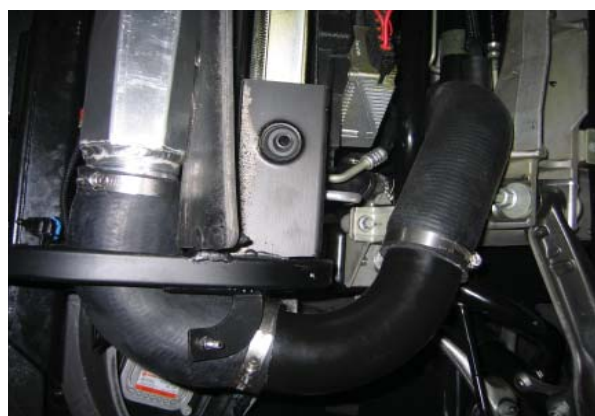
Tubing Between Fan & Engine Cradle
