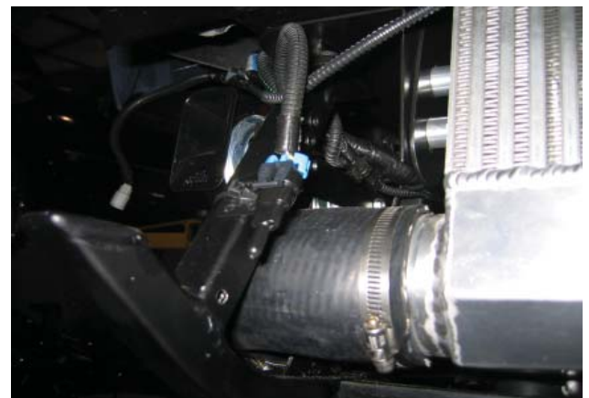
Temperature Sensor Relocation
