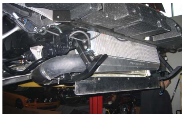
Intercooler and 3" Elbow Installed
