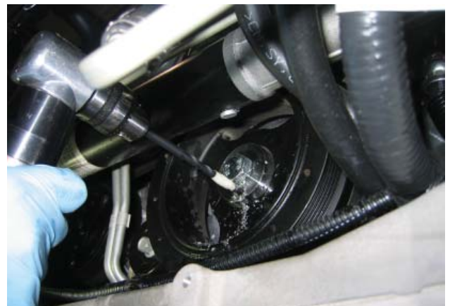
Drilling the Harmonic Balancer
