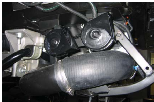
3" Metal 90° Tube Installed
