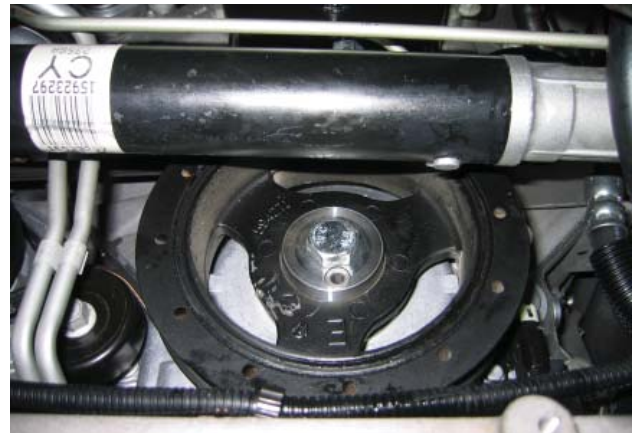
Harmonic Balancer Pinning Tool
