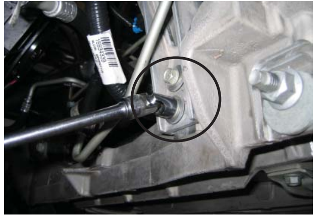
Traction Control Module Bolts
