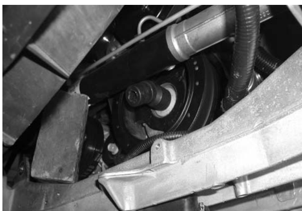
Harmonic Balancer Bolt Removal
