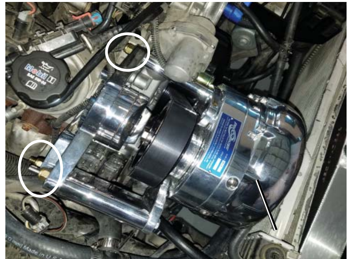
Bolting Supercharger to the Sub Bracket
