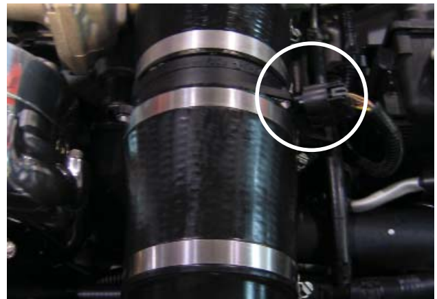
MAF Sensor Installation
