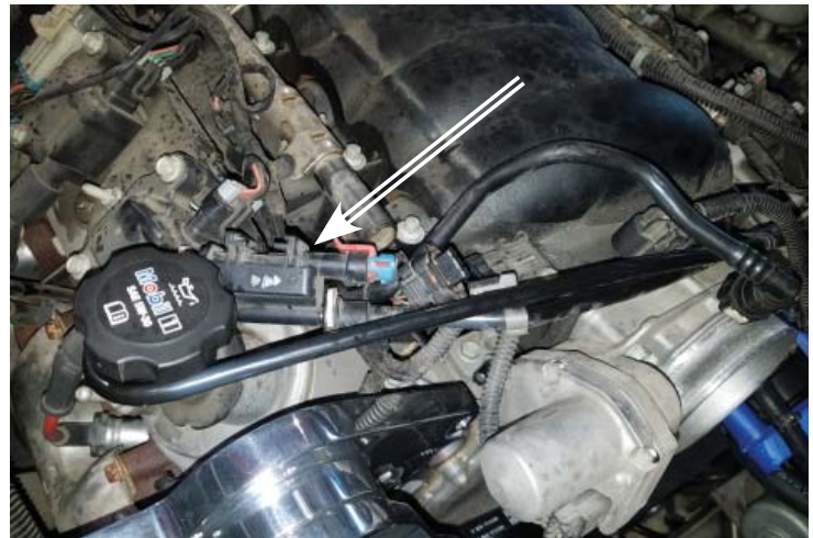
Air Solenoid Relocated
