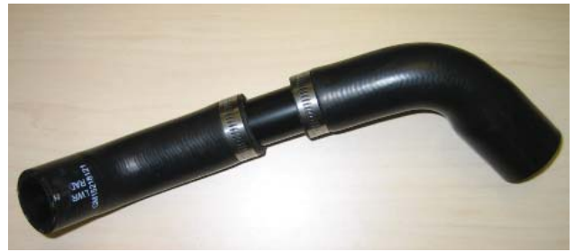
Lower Radiator Hose Modified
