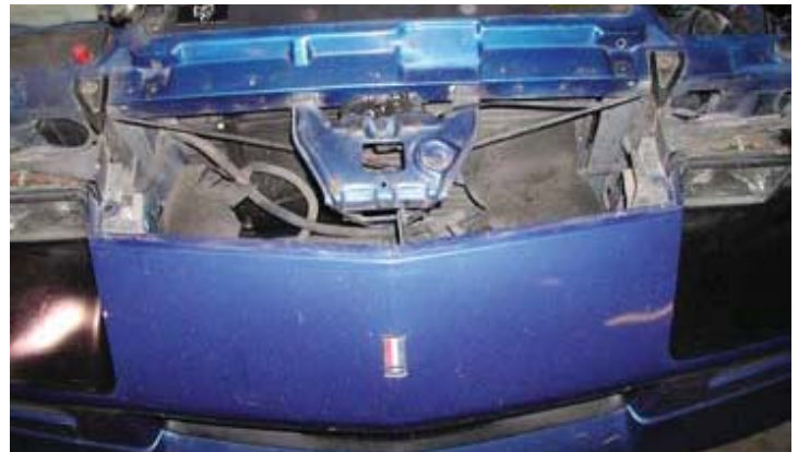
Factory Air Filter Housing Removed
