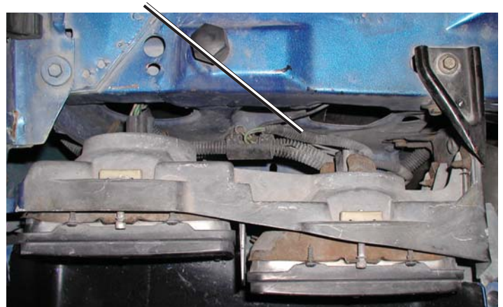
Wiring Harness Relocation (Pass. Side)
