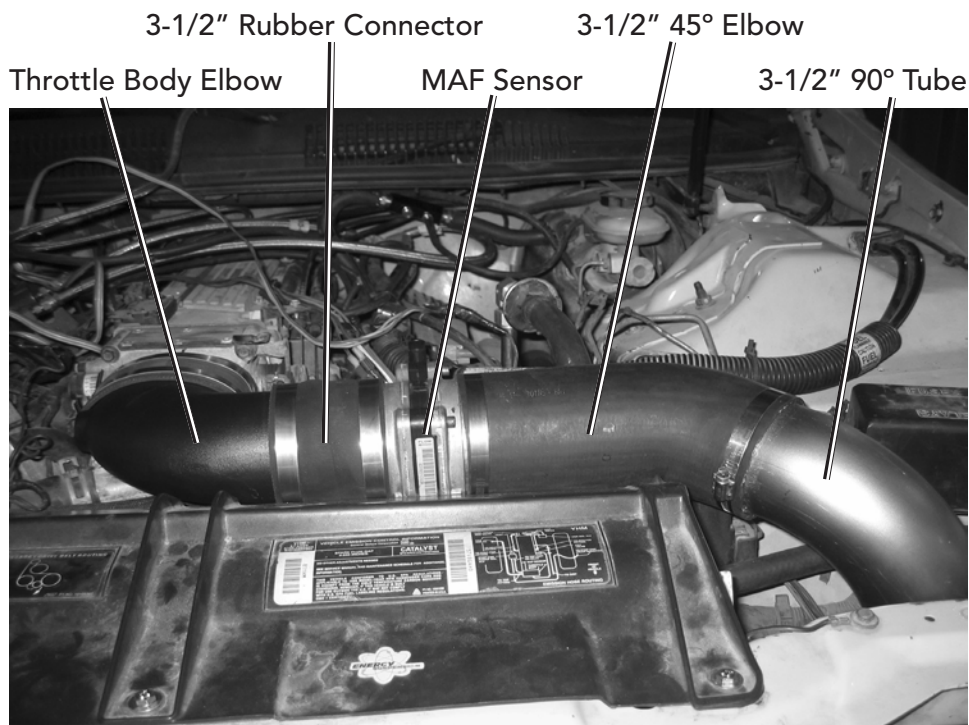
Throttle Body Tubing Installation
