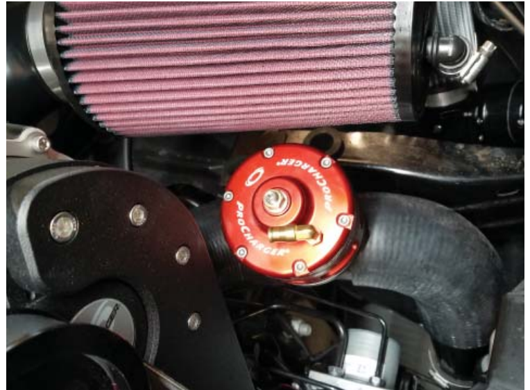
Race Valve Install
