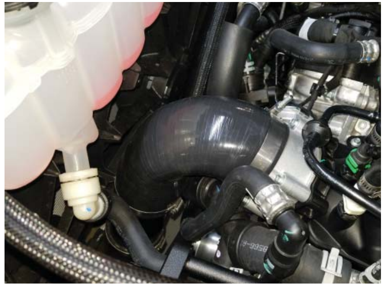
Tubing To Throttle Body Installed
