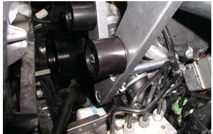
Main Bracket Installed (Lower Spacers)
