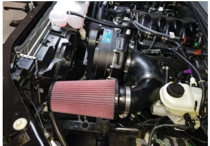
Air Filter Inlet Installed
