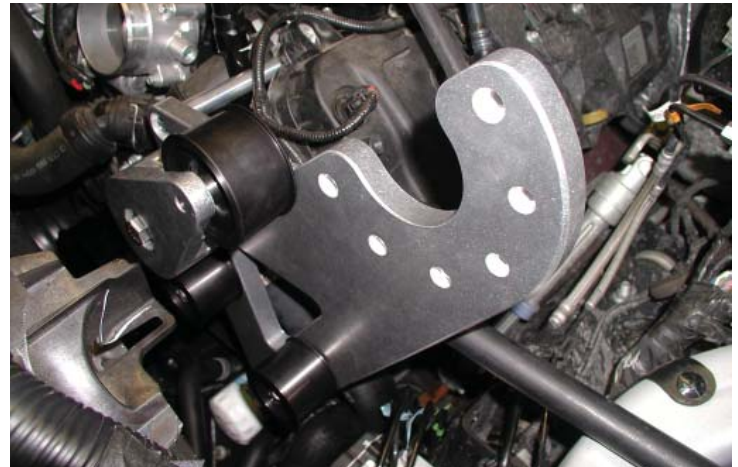
Main Bracket Installed
