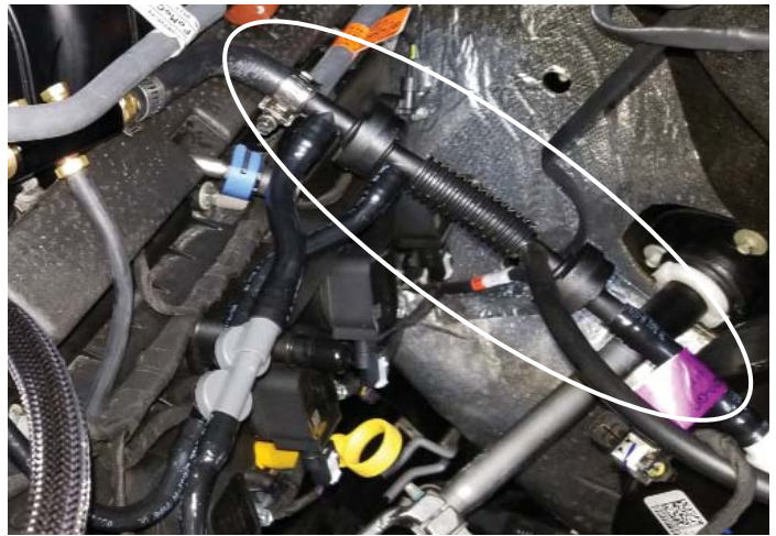
Factory Vacuum Line To Brake Booster
