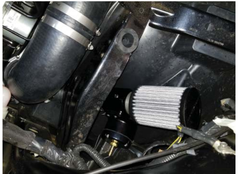
Surge Valve Installed
