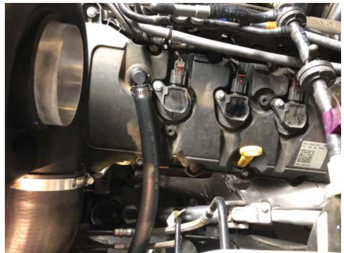
PCV Line Installed
