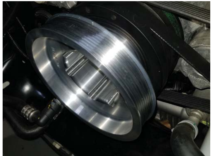
Crank Pulley Installed
