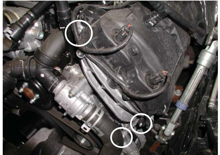
Remove Factory Hardware
