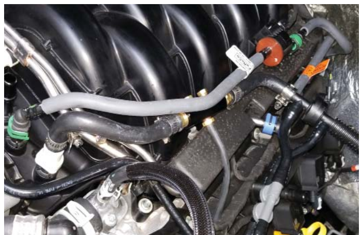
Vacuum Manifold Installed
