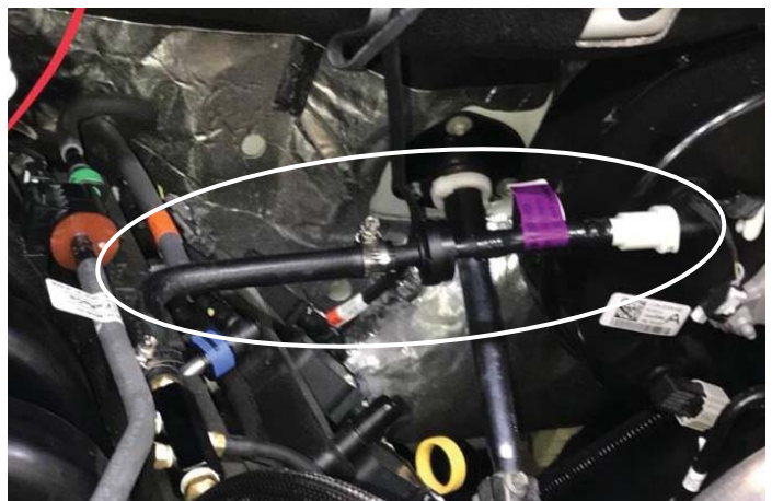
Factory Vacuum Line to Brake Booster
