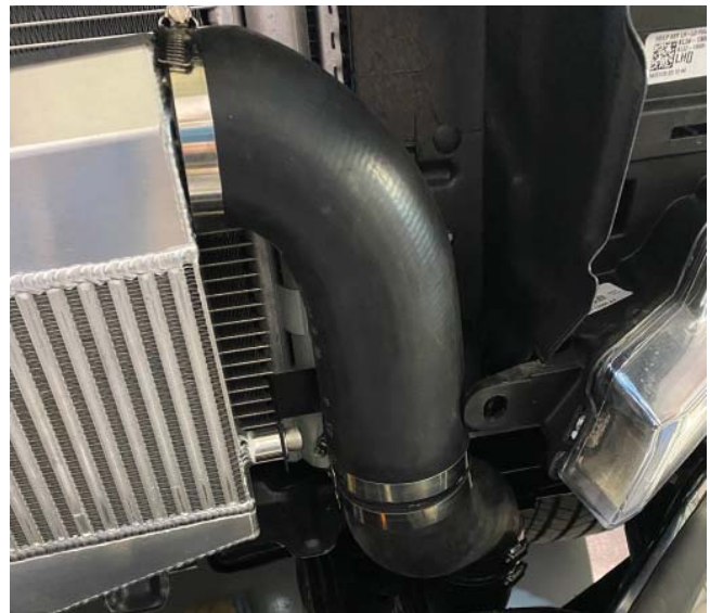
Tubing To Intercooler Installed
