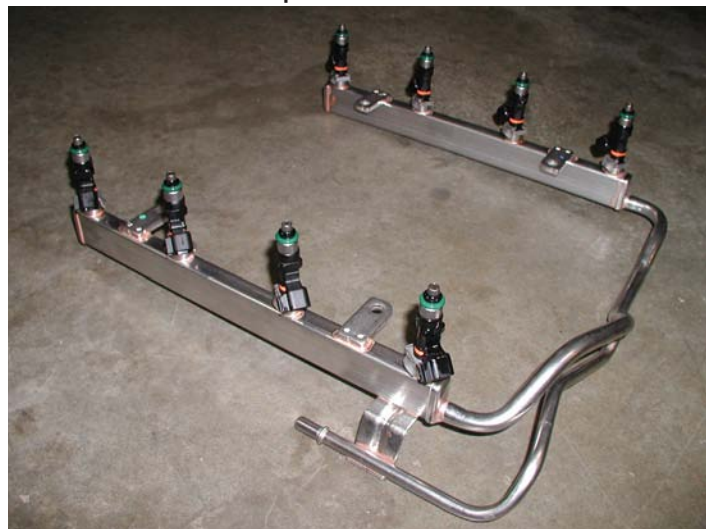
New Fuel Injectors Installed Onto Fuel Rail Assembly
