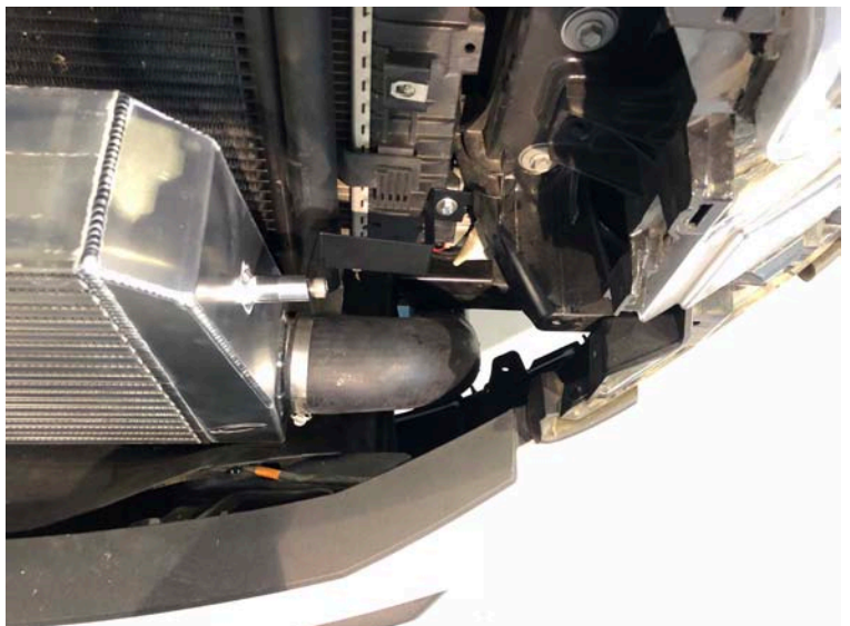
Tubing To Intercooler Installed
