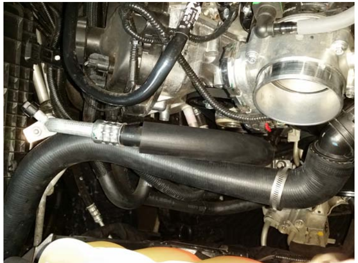
Re-install Fitting and Supplied Radiator Hose
