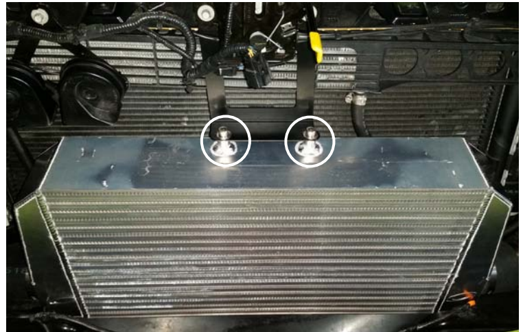
Intercooler Installed to Upper Bracket
