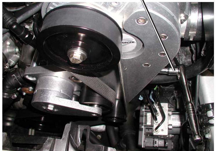
Belt Tensioning (Brass Collar Access)
