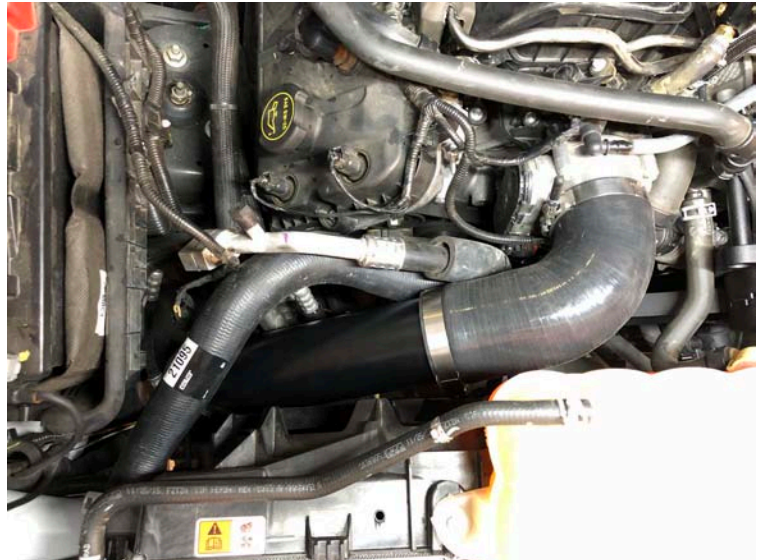
Tubing To Throttle Body Installed
