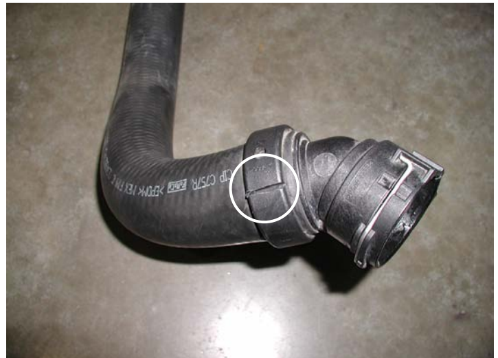
Cut Plastic Ring Clamp to Remove Fitting
