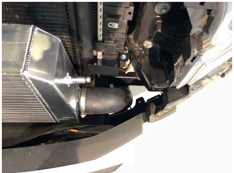
Tubing To Intercooler Installed
