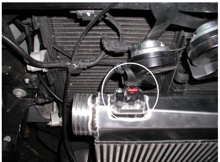
MAF Extension Connected
