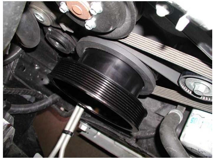
Crank Pulley Installed
