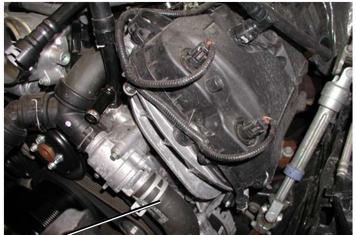
Disconnect Lower Radiator Hose
