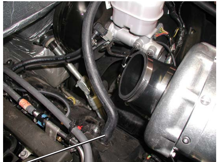
PCV Line and Rear Inlet Coupler Installed
