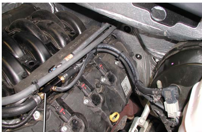
Vacuum Manifold Installed
