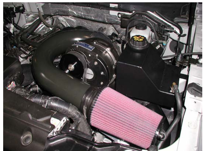
Forward Inlet and Air Filter Installed
