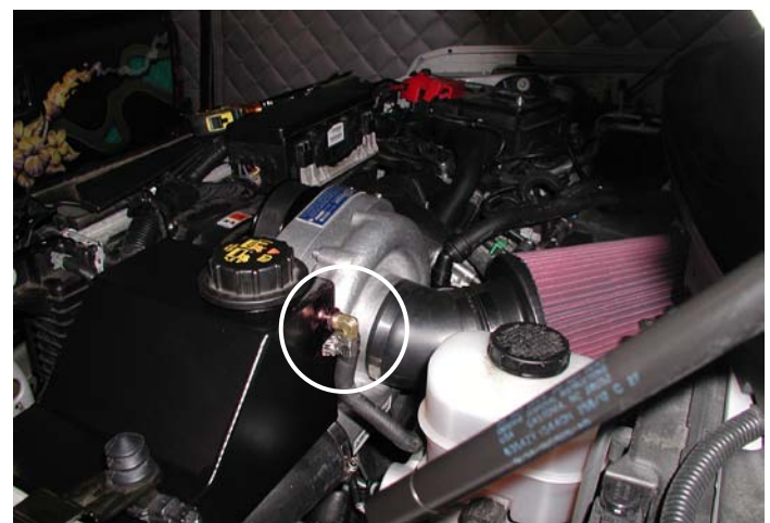
Rear Overflow Line Connected
