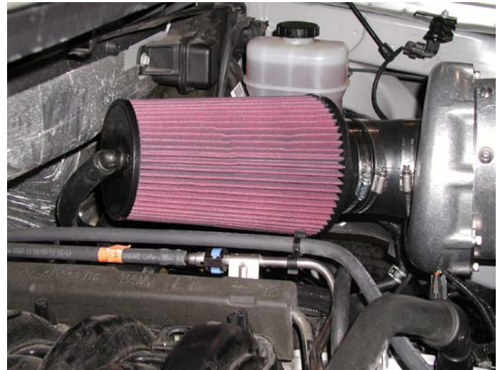
Rear Inlet and Air Filter Installed
