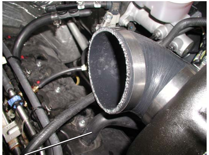
PCV Line and Forward Inlet Coupler Installed
