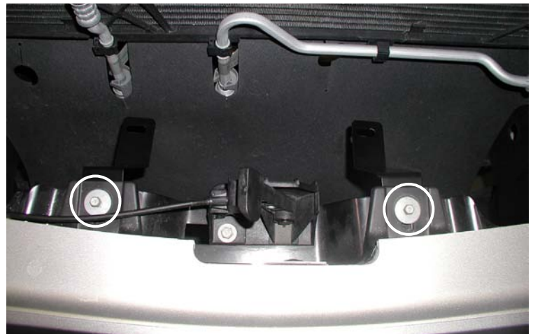
Lower Intercooler Brackets Installed
