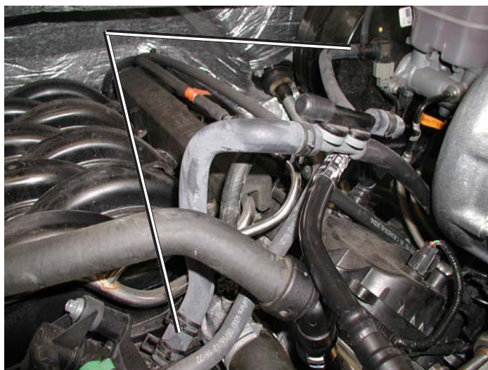
Vacuum Line Removal
