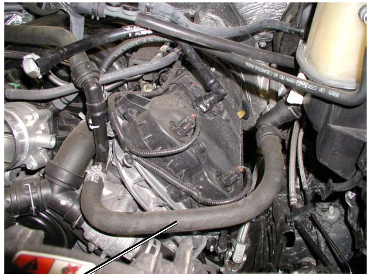
Remove Lower Supply Hose
