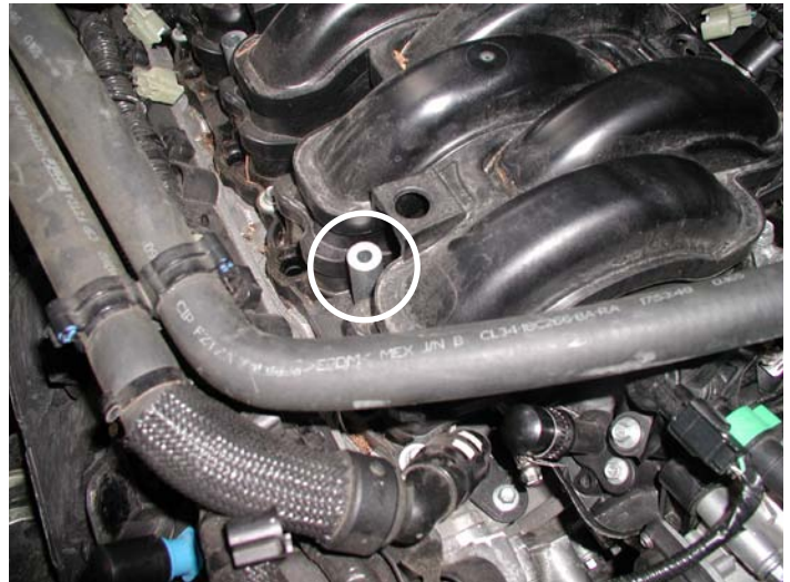
Remove Fuel Rail Spacers (4x)
