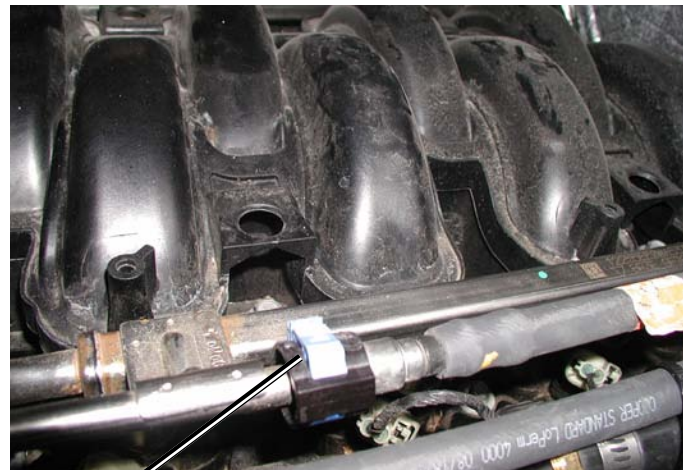
Disconnect Fuel Supply Line
