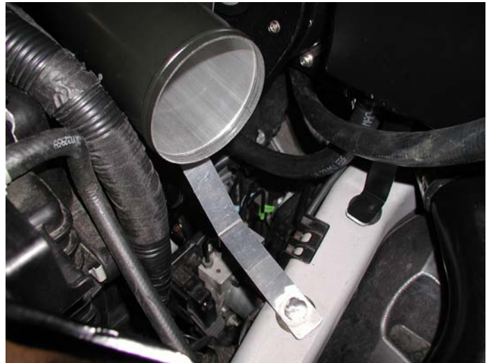
Forward Inlet Tube & Bracket Installed
