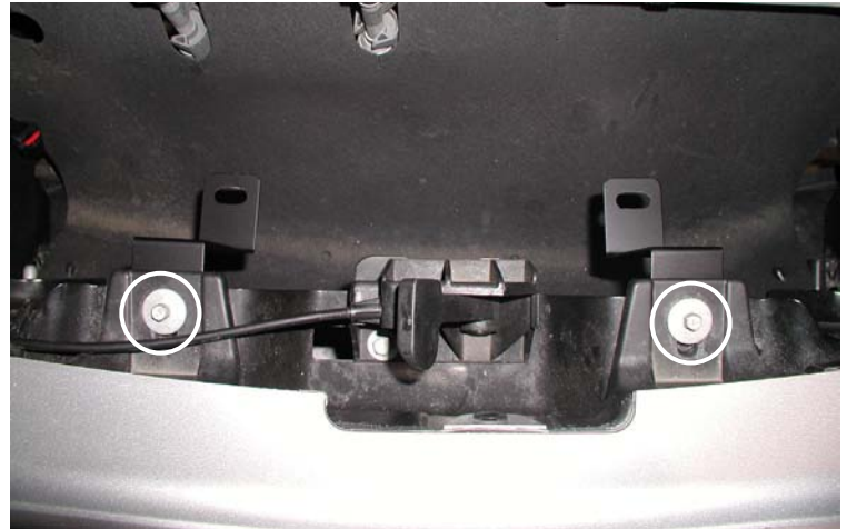
Lower Intercooler Brackets Installed
