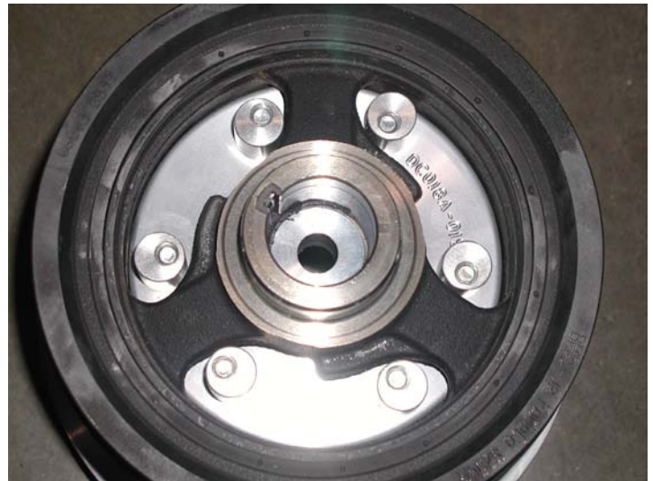
Back View of Crank Pulley and Cam Locks Installed
