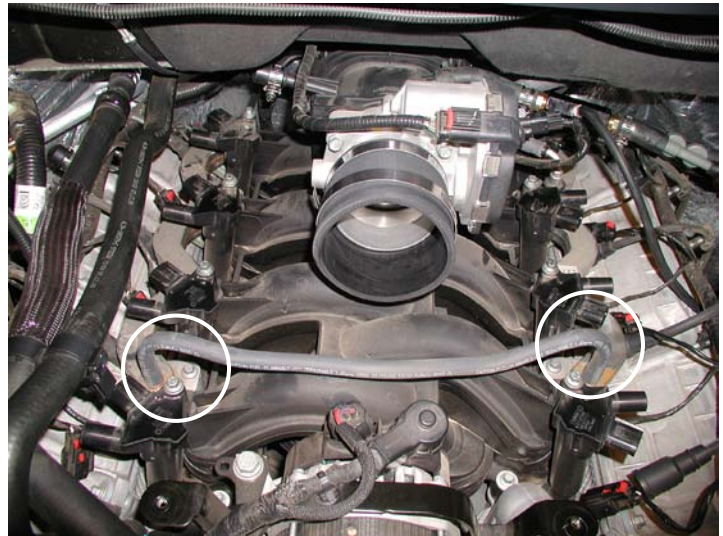
Front Fuel Rail Bolts (4 Total)
