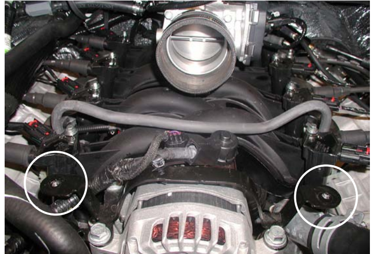
Engine Cover Base Mounting Locations
