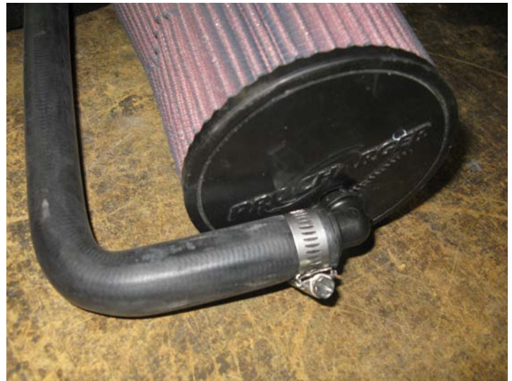
PCV Hose Routed to End of Filter
