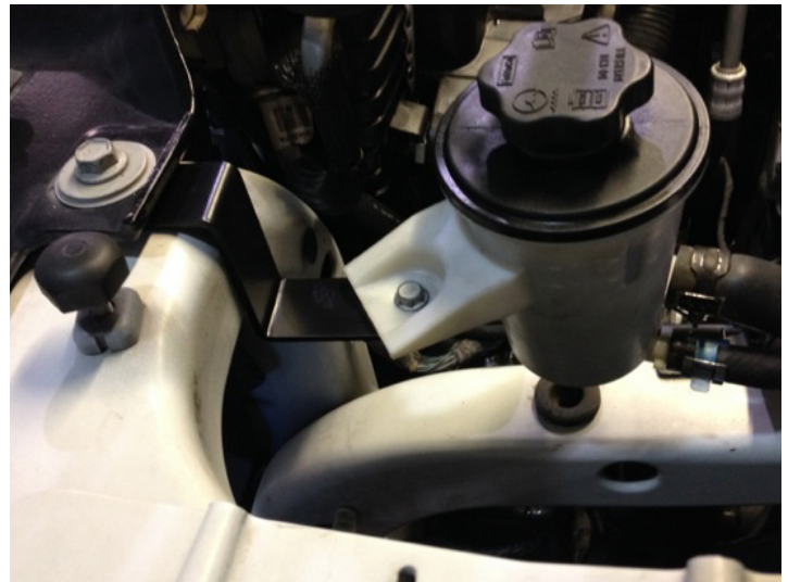
Power Steering Reservoir Mounted
