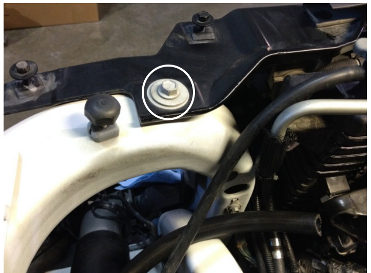
Radiator Support Bolt
