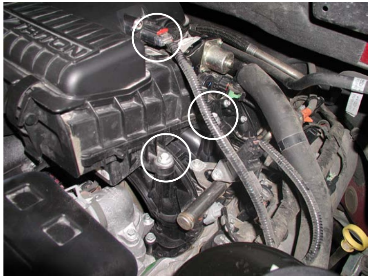
Disconnect MAF Harness & Remove Driver's Side Air Filter Box Bolts
