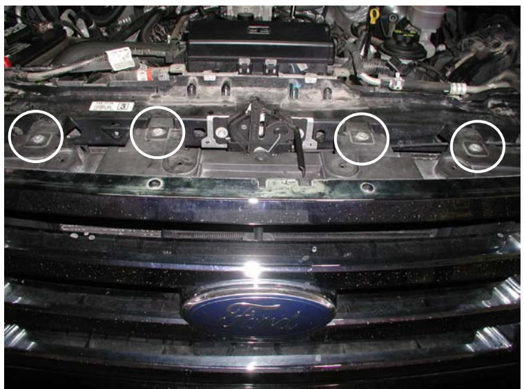
Remove Upper Grill Support Bolts
