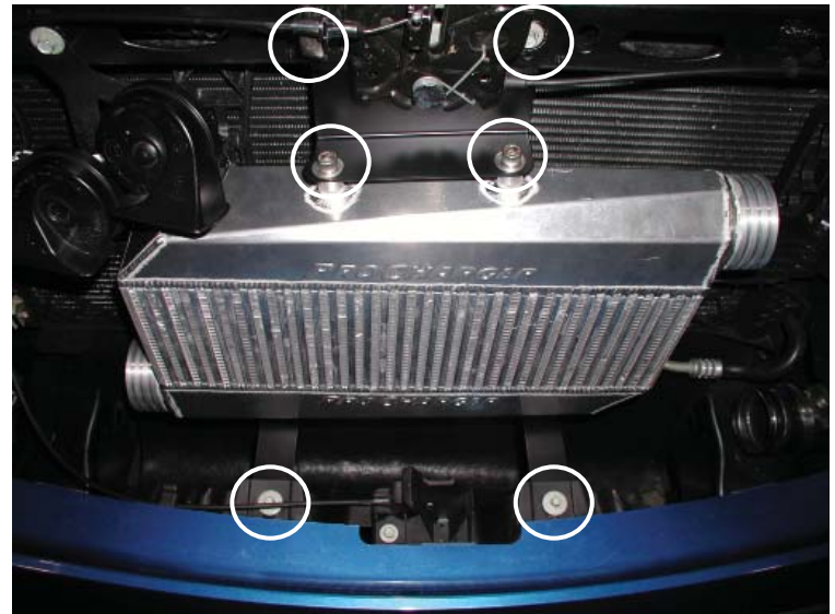
Intercooler & Brackets Installed
