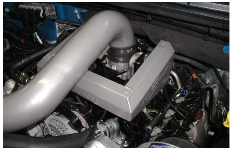
Intake Cover Base Installed
