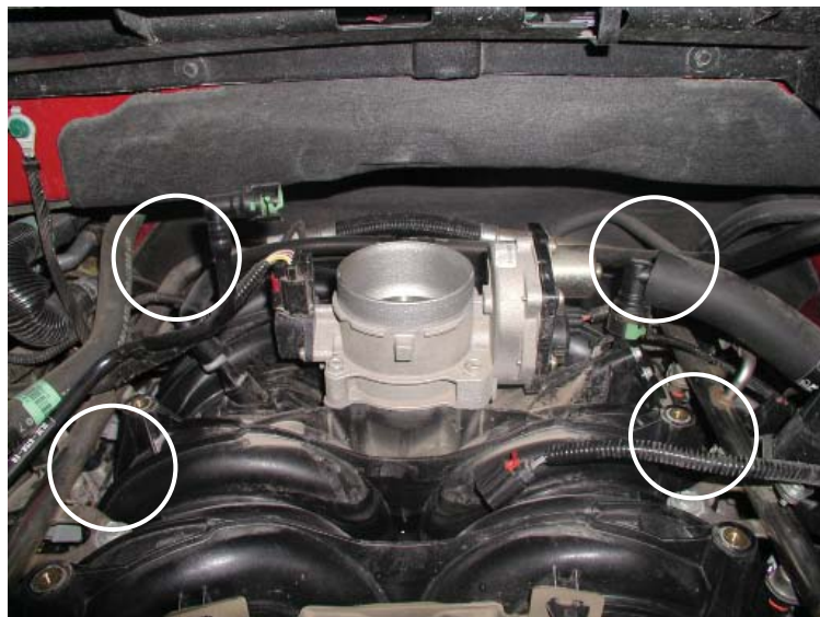
Fuel Rail Retaining Bolts
