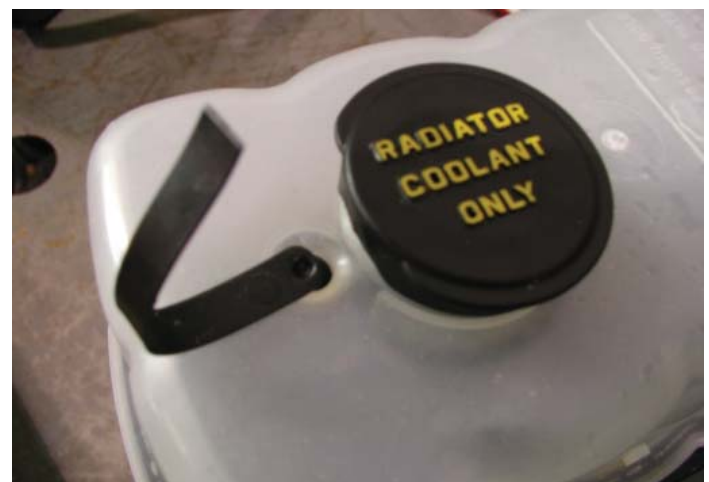
Factory Coolant Tank Cap Removal
