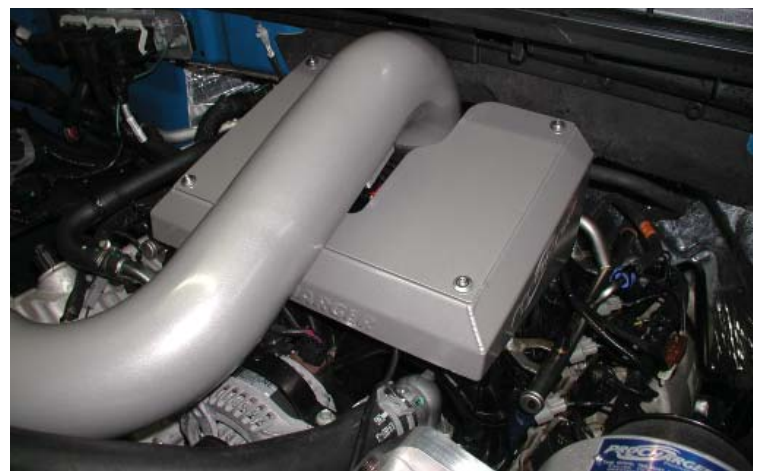
Intake Cover Installed
