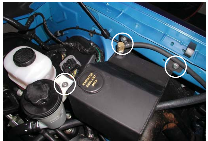
Coolant Tank Installed
