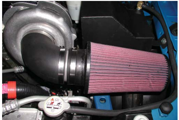
Air Inlet Assembly Installed
