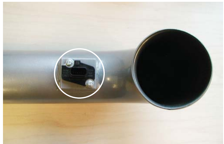
Factory MAF Installed in Intake Tube
