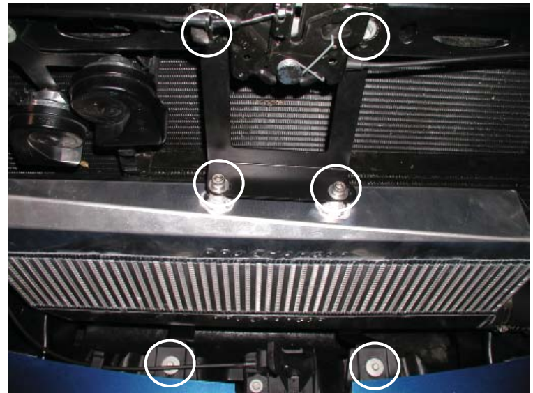
Intercooler & Brackets Installed
