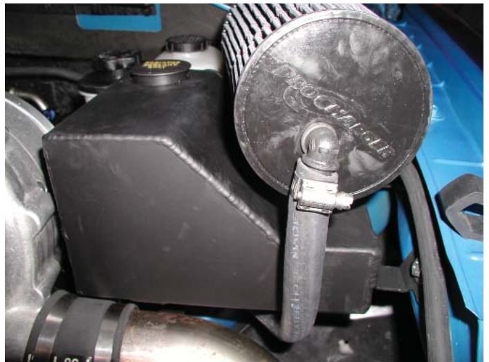
PCV Line Installed in Air Filter
