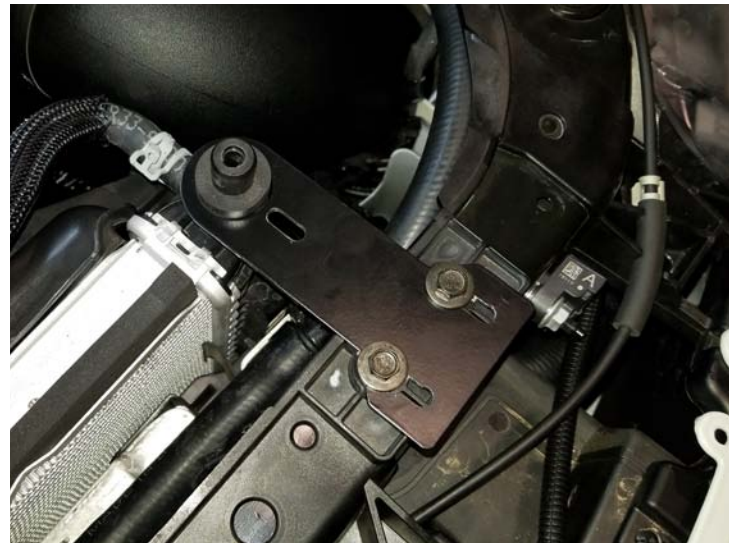
Radiator Bracket Installed
