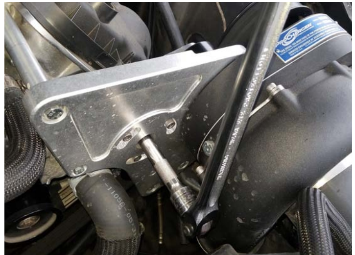
Rotate Tensioner Counter Clockwise
