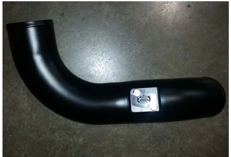
MAF Installed Into Tube #430
