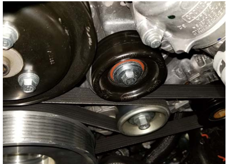
New Idler Shaft Installed
