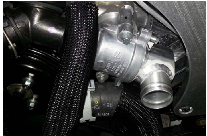
New Thermostat Housing Neck Installed
