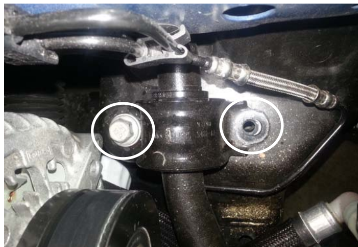
Driver's Front Sway Bar Bolt Removed
