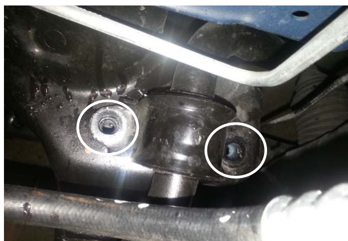
Passenger's Sway Bar Bolts Removed
