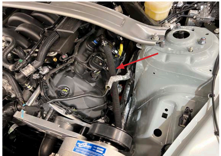
PCV Line Installed
