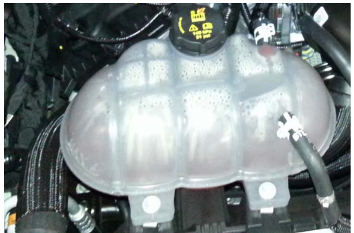
Factory Coolant Reservoir
