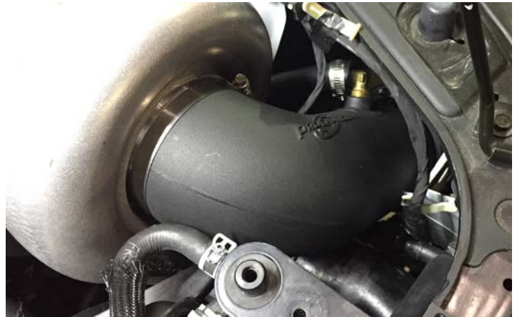
Inlet Elbow Installed
