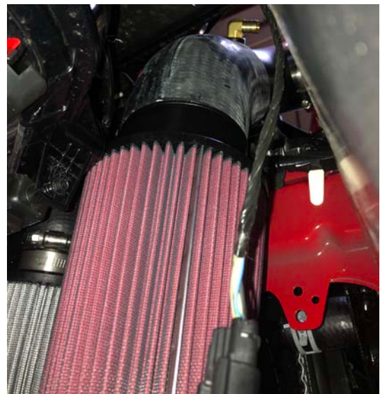
Air Filter Installed
