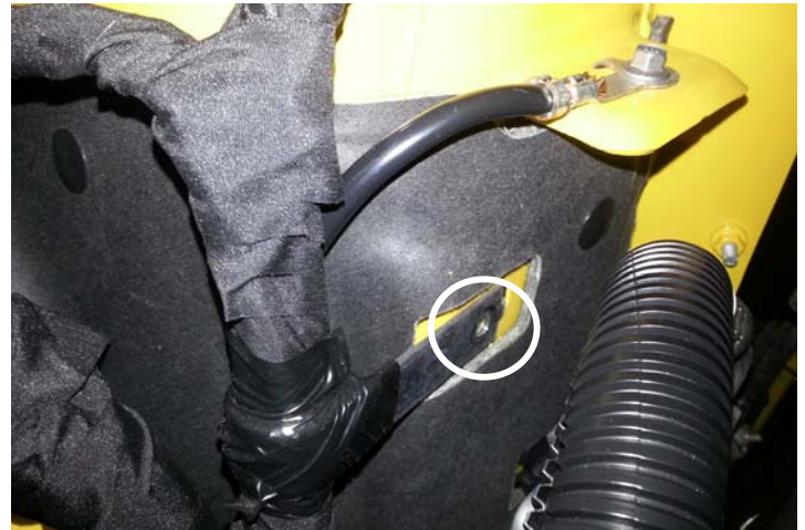
Wiring Harness Screw (Passenger's Side)
