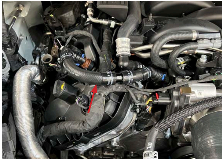
PCV Line Installed
