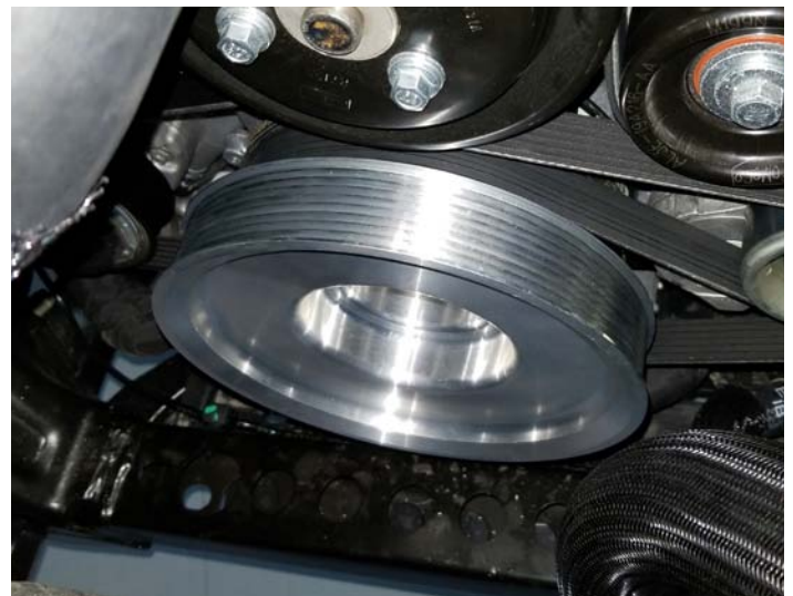
Crank Pulley Installed
