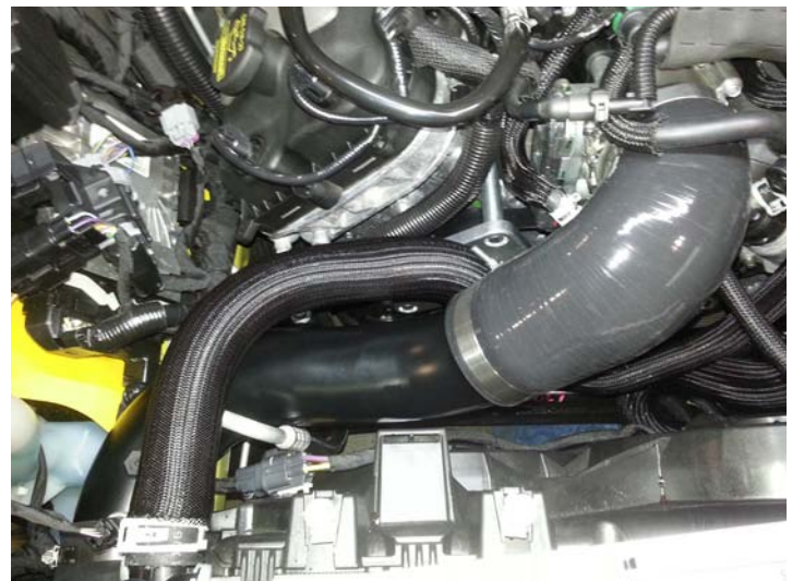
Throttle Body Elbow Installed
