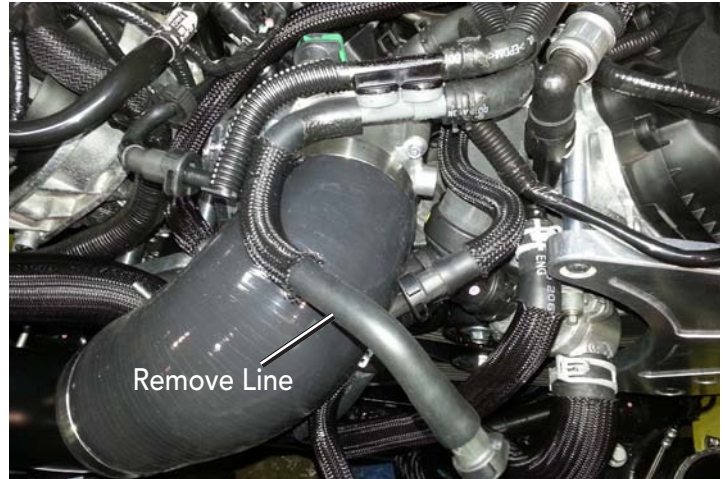
Factory Vacuum Tree
