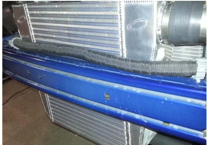
Wiring Harness Relocated
