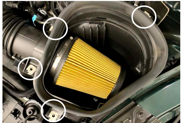
Remove Rubber Hood Seal
