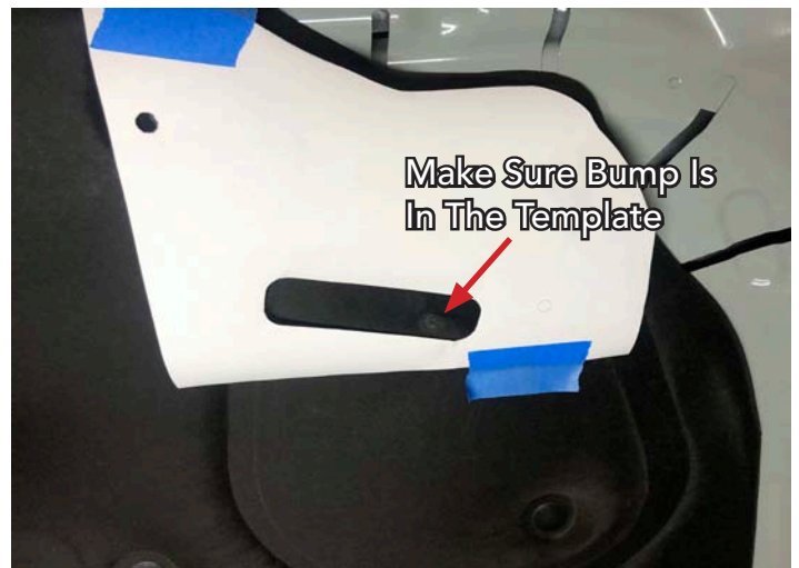
Hood Liner Template Installed (Mach 1)
