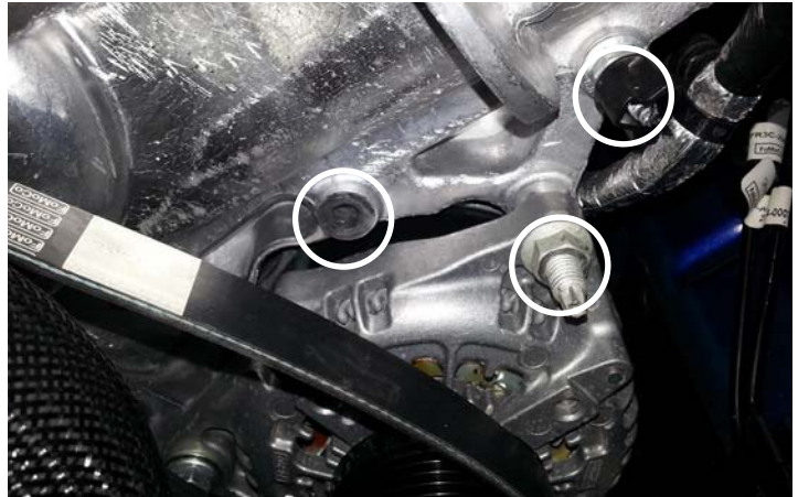
Remove Factory Hardware (Driver's Side)
