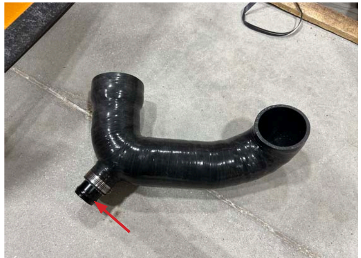
1.5" Connector Tube Installed
