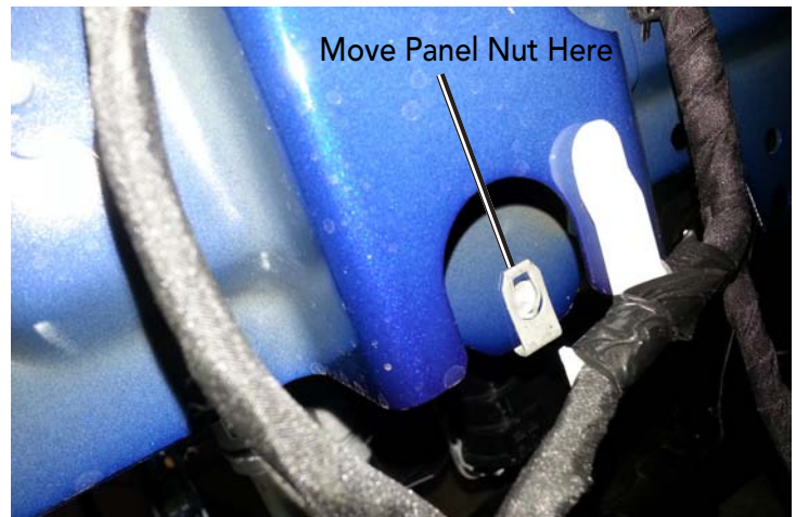
Horn Nut Relocated
