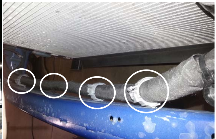
Wiring Harness Retainers
