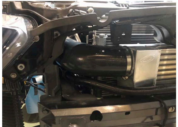
3.5" 90° Silicone Elbow Installed
