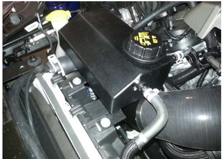
New Coolant Reservoir Mounted
