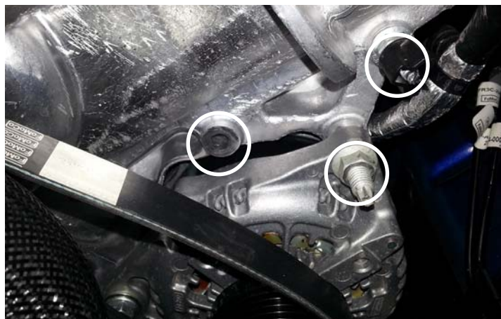
Remove Factory Hardware (Driver's Side)
