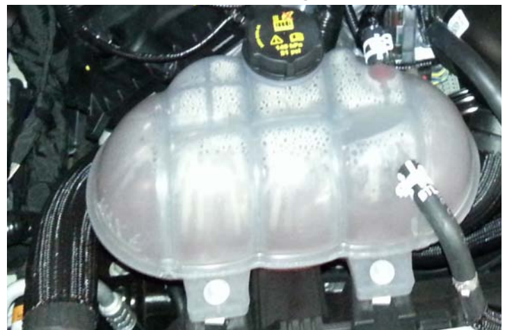
Factory Coolant Reservoir
