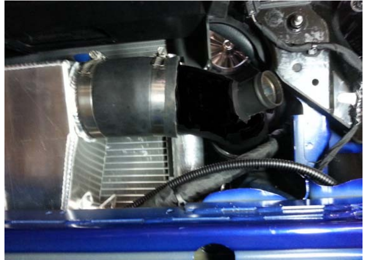
Surge Tube #380 Installed
