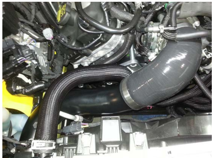
Throttle Body Elbow Installed
