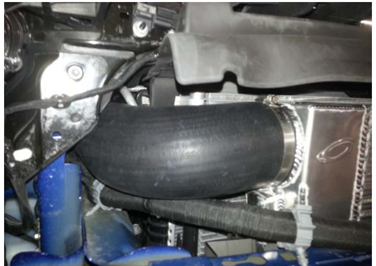
3.5" 90° Rubber Elbow Installed
