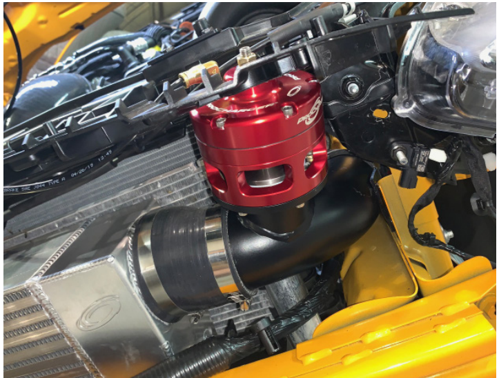
Race Valve Tube Installed
