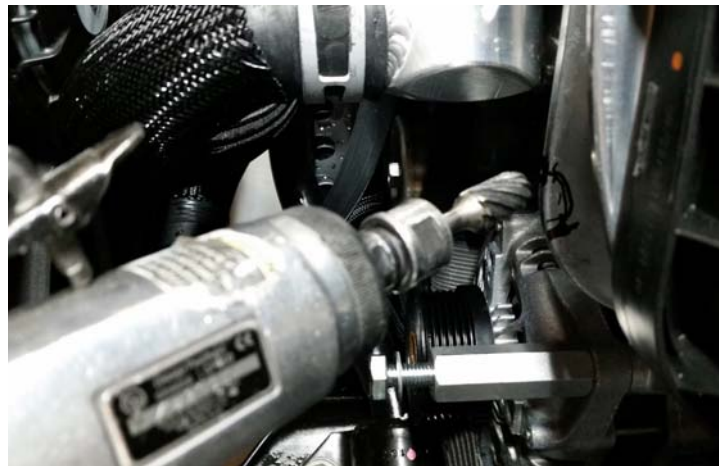
Notch With a Cutting Tool (Die Grinder Shown)
