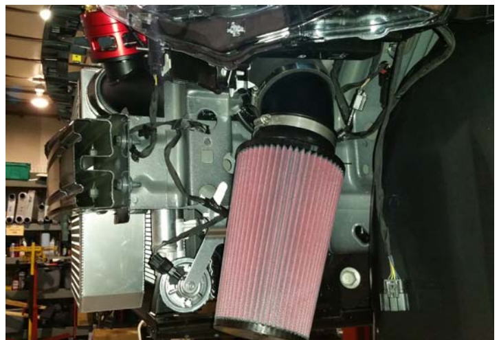
Air Filter Installed
