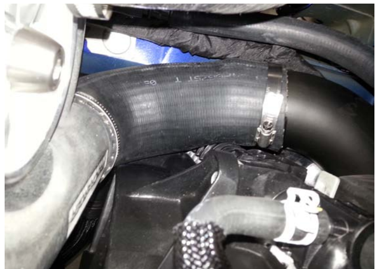
Blower Discharge Tube Installed
