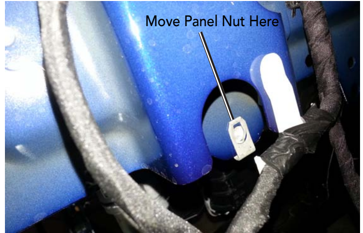
Horn Nut Relocated
