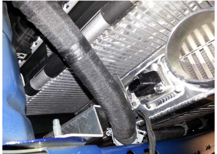
H.O Intercooler Only: MAF Sensor Installed
