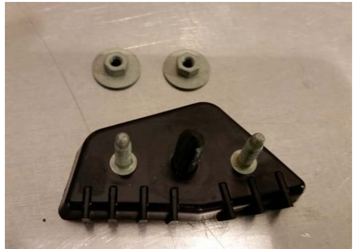
Plastic Stud Housing Removed
