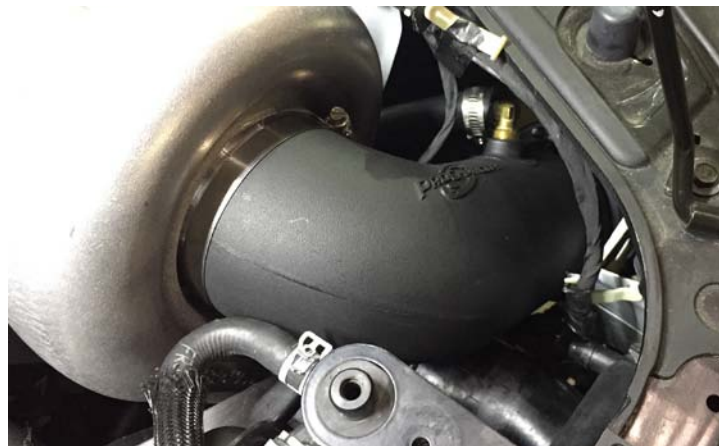
Inlet Elbow Installed
