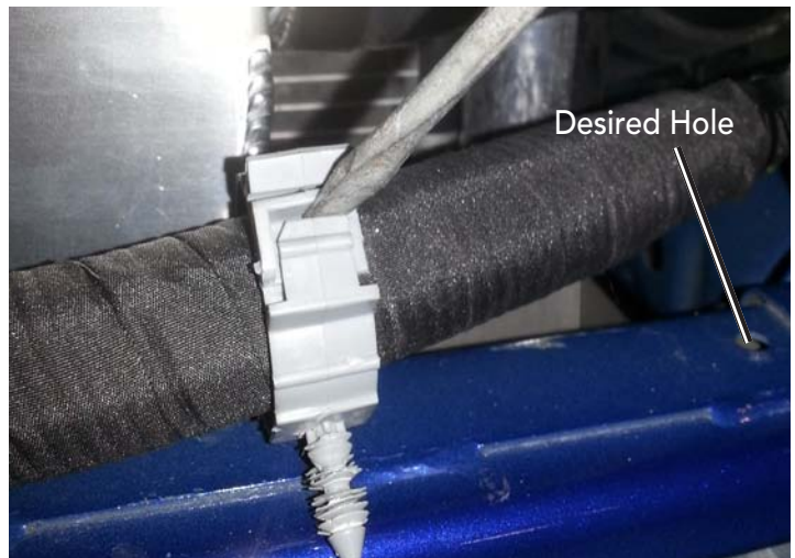
Unclip the Driver's Side Harness Retainer
