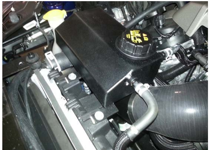
New Coolant Reservoir Mounted
