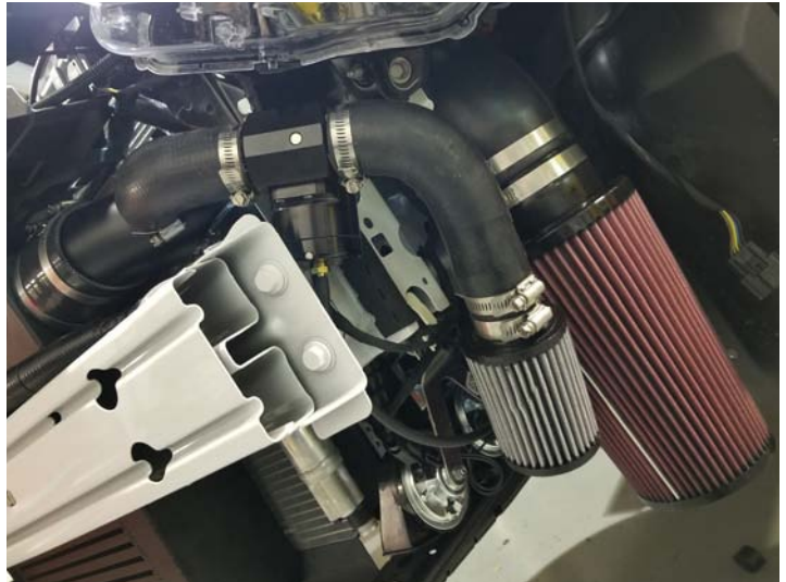
ProFlow Surge Valve Installed
