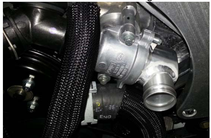
New Thermostat Housing Neck Installed
