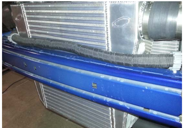
Wiring Harness Relocated
