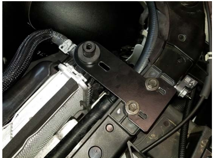
Radiator Bracket Installed
