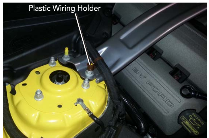
Strut Tower Bar (Passenger's Side)
