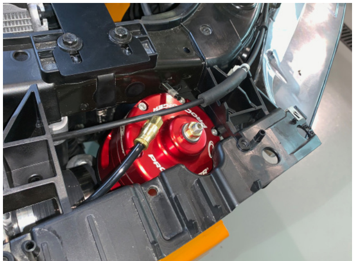
Race Valve Tube Installed
