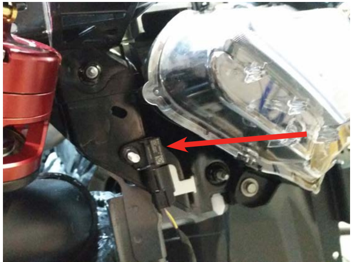
Airbag Sensor Relocated
