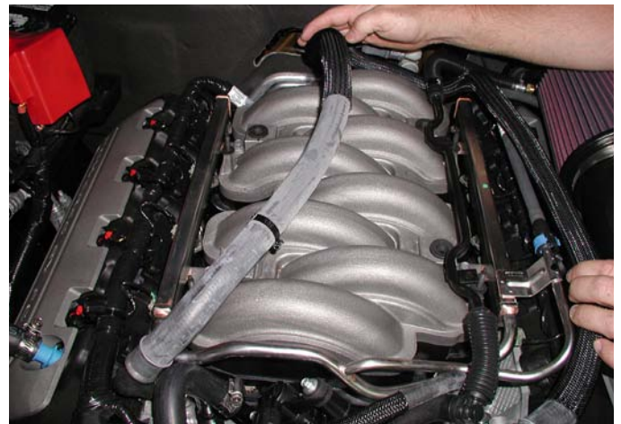
Adjust Coolant Lines For Fuel Rail Removal
