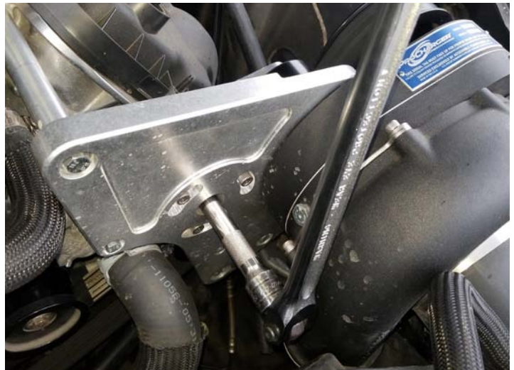
Rotate Tensioner Counter Clockwise
