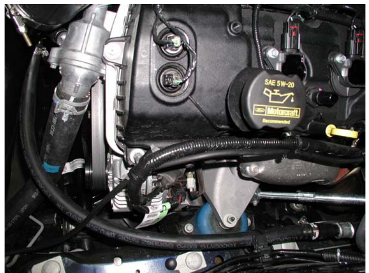
Heater Hose Installed
