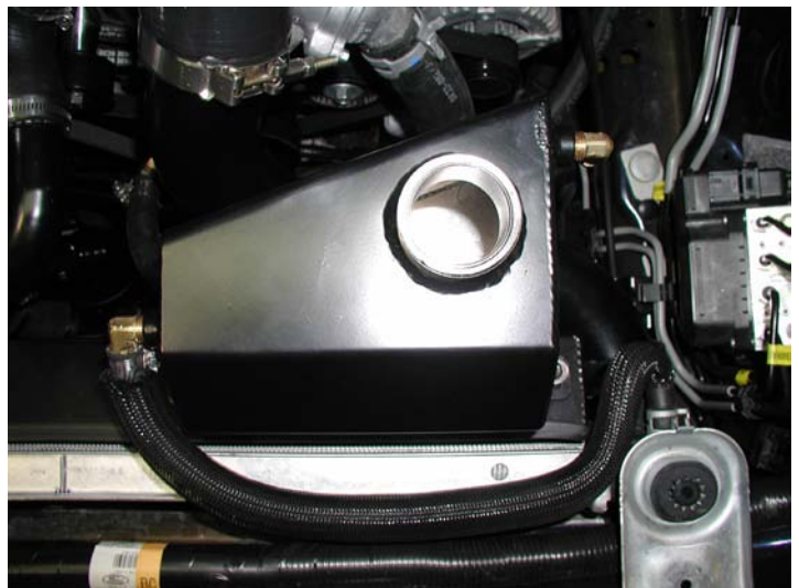
Radiator Overflow Hose Installed
