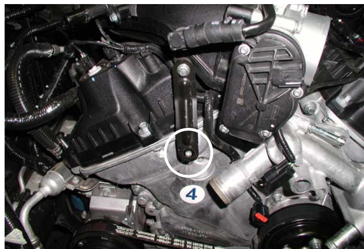
Remove Front Bracket Bolt
