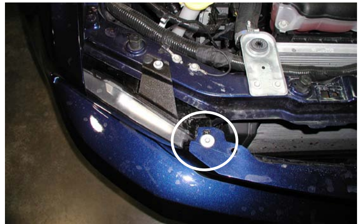
Top Bumper Cover Bolts (Passenger's Side)
