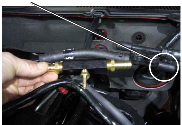
Vacuum Manifold Installation (Automatic)
