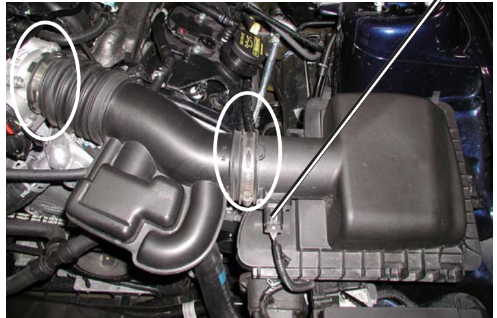
Loosen Air Inlet Connections
