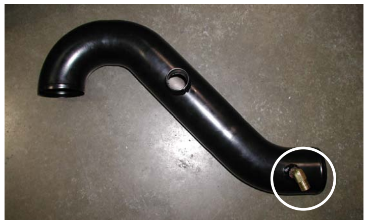
PCV Fitting Installed
