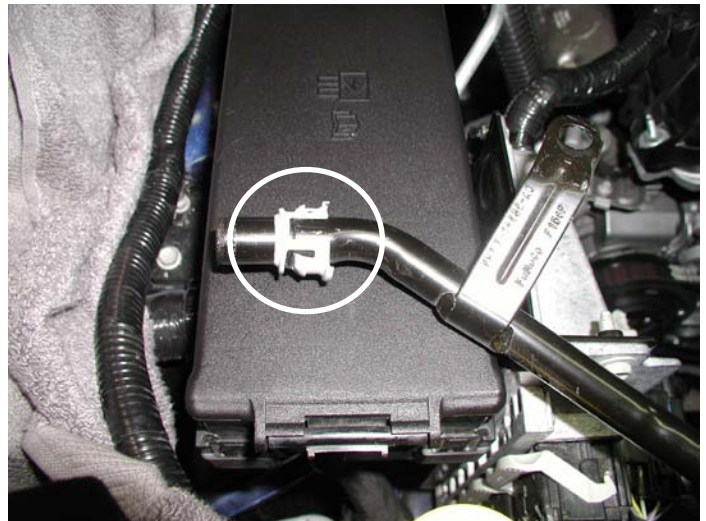
Heater Line Retaining Clip
