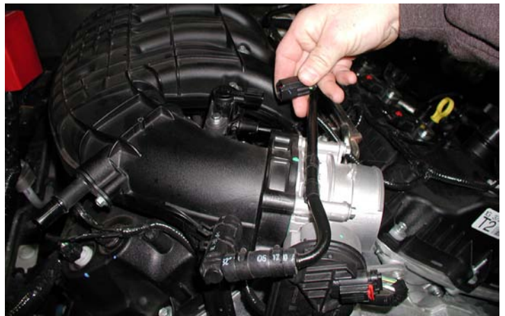
Disconnect Fuel Pressure Wiring Harness
