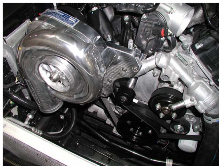
ProCharger Head Unit Installed
