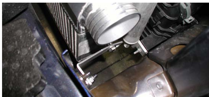
Lower Intercooler Bolt Installed (Driver's Side)
