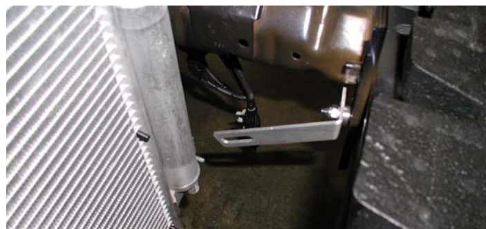
Lower Intercooler Bracket Installed (Driver's Side)
