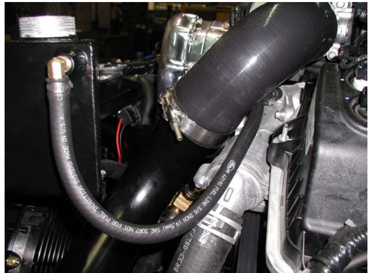
Upper Coolant Hose Installed
