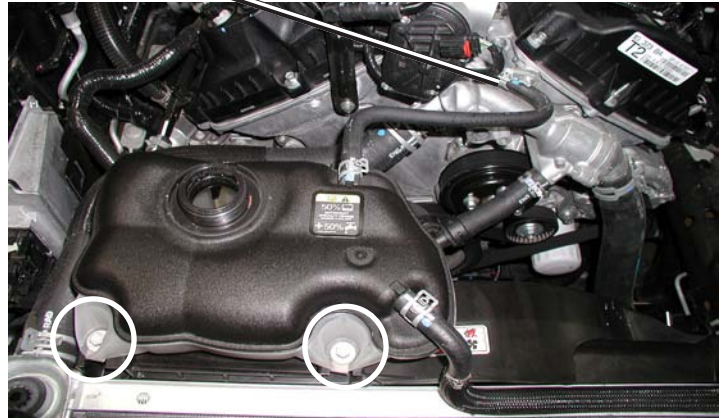
Coolant Tank Bolts
