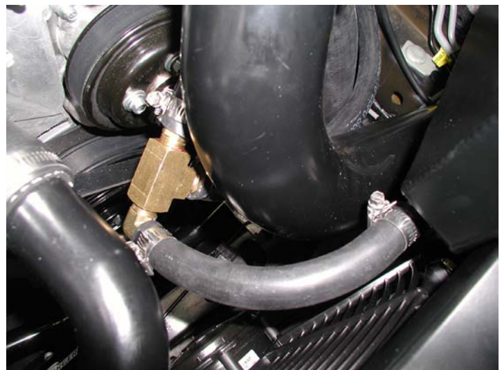
Lower Coolant Line Installed
