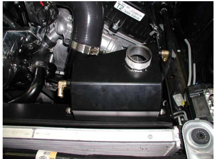
Coolant Reservoir Installed
