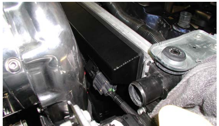
Shroud & Fan Installed (Passenger's Side)
