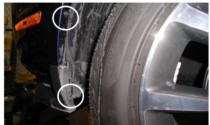
Inner Fender Well Screws (2011-2013 Shown)
