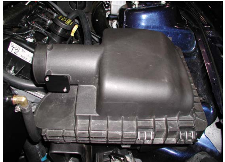
Factory Airbox Cover & MAF Cover Installed
