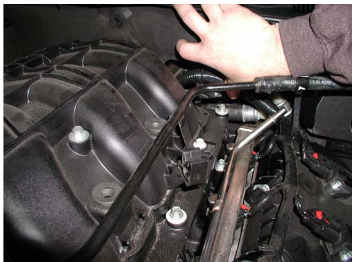
Unclip Wiring Harness From Intake
