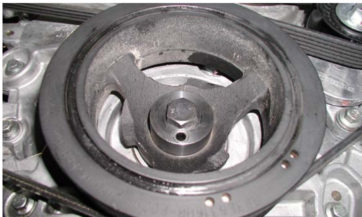
Install Crank Pinning Jig
