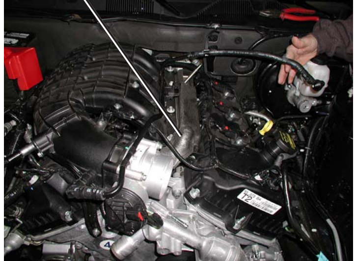
Disconnect Vacuum Line From Brake Booster & Remove Fuel Rail Insulator
