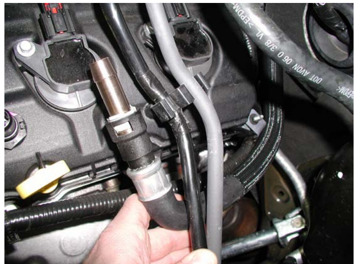
Heater Hose Fitting Installed
