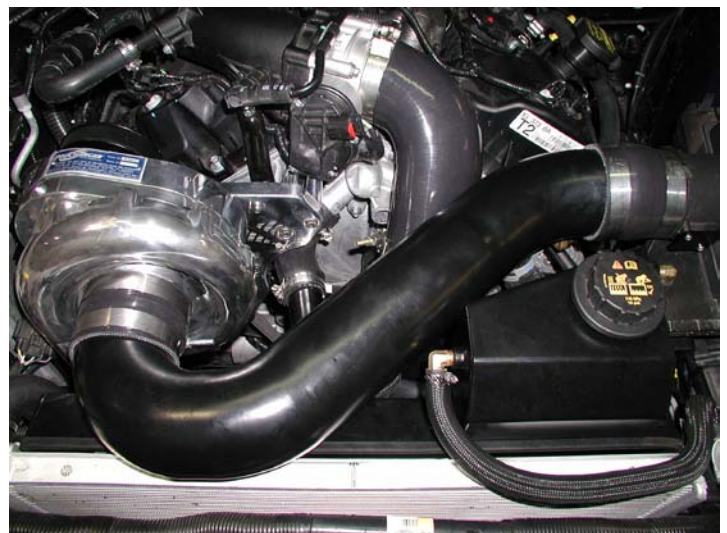
Air Inlet Tube Installed
