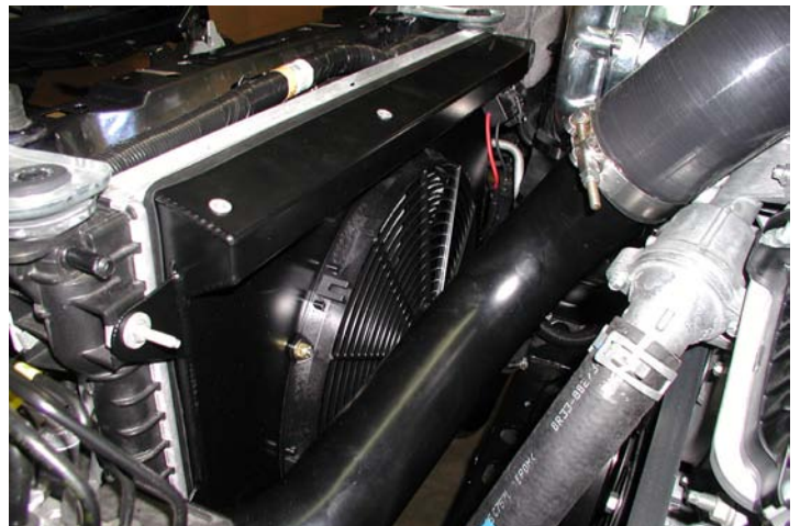
Shroud & Fan Installed (Driver's Side)
