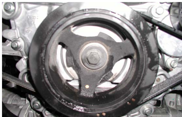
Remove Factory Balancer Bolt
