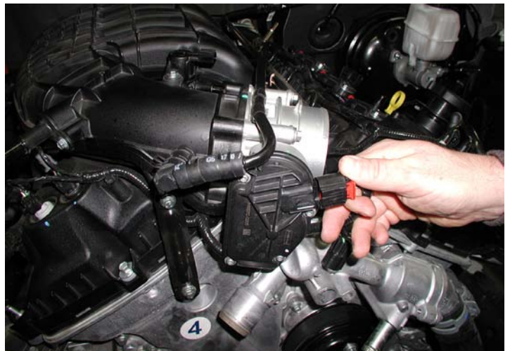
Disconnect Throttle Wiring Harness
