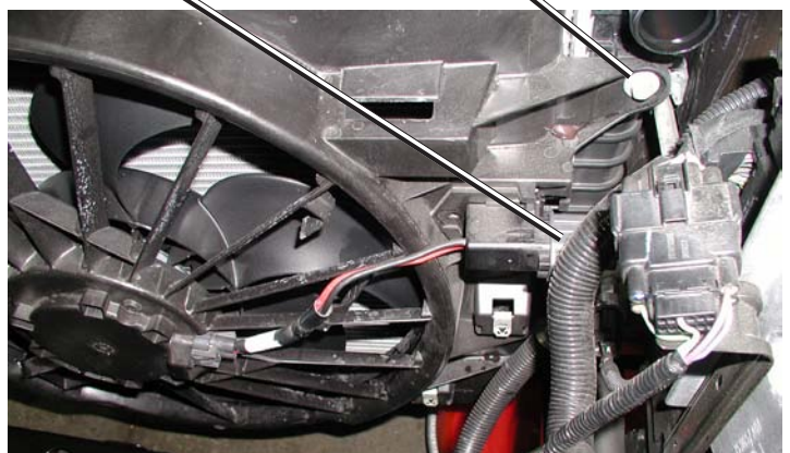
Disconnect Wiring Harness & Remove Bolt
