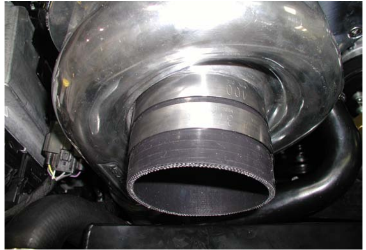
ProCharger Inlet Coupler Installed
