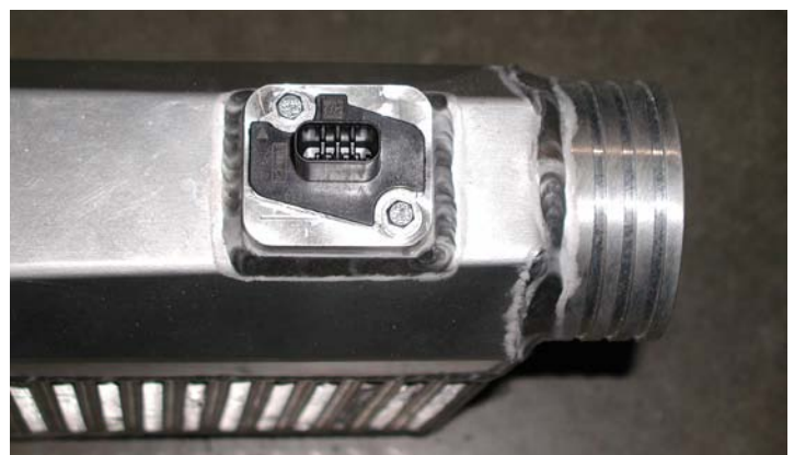
MAF Sensor Installed
