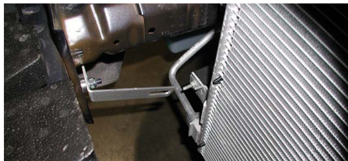
Lower Intercooler Bracket Installed (Passenger's Side)
