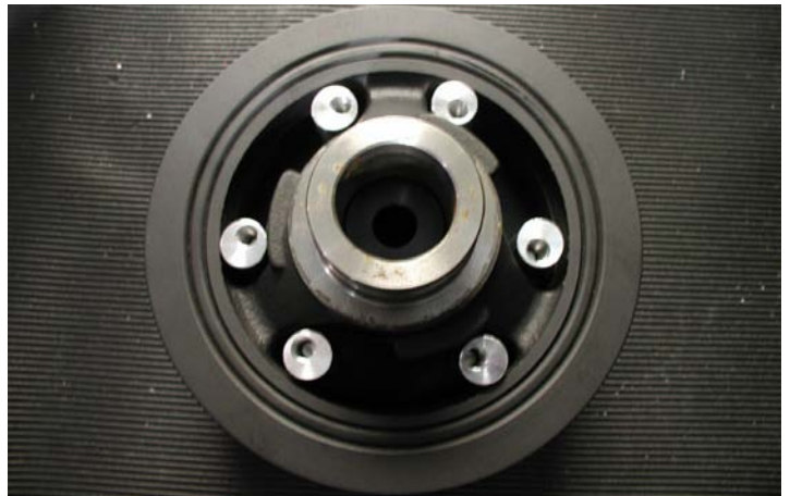
Back View of Crank Pulley and Cam Locks Installed
