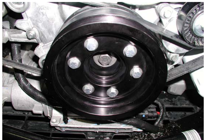
Crank Pulley Installed
