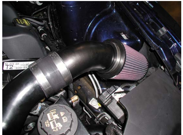
Cold Air Inlet Installed
