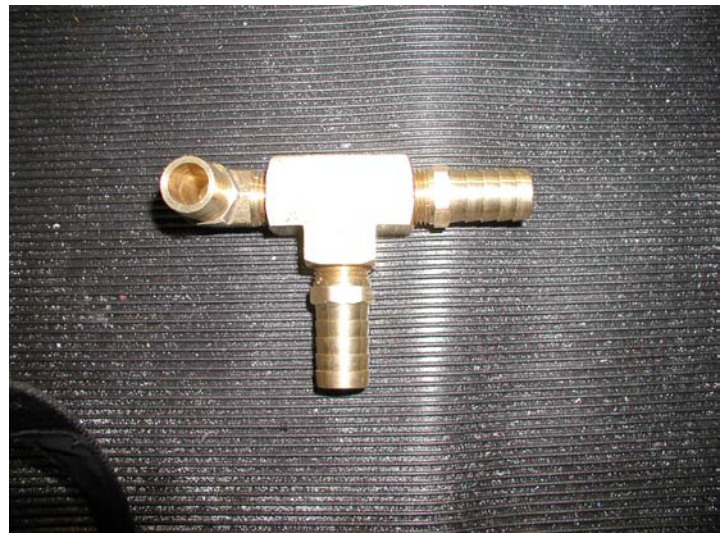
Coolant "T" Fitting Assembled
