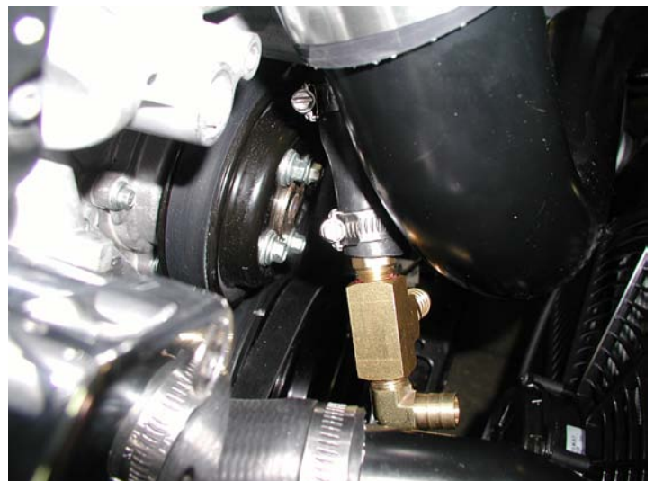
Coolant Fitting Installed
