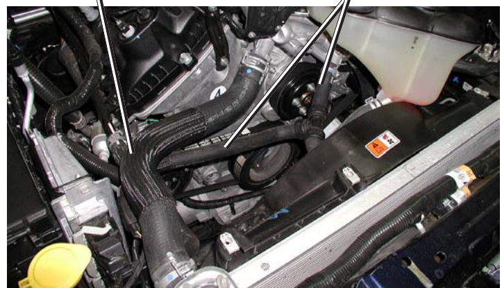
Upper Radiator Hose, Heater Hose & Return Line
