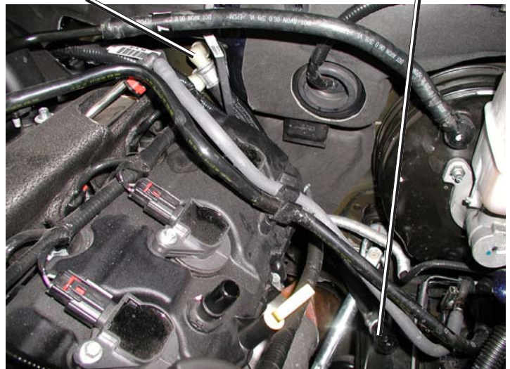
Firewall Heater Hose Rotated
