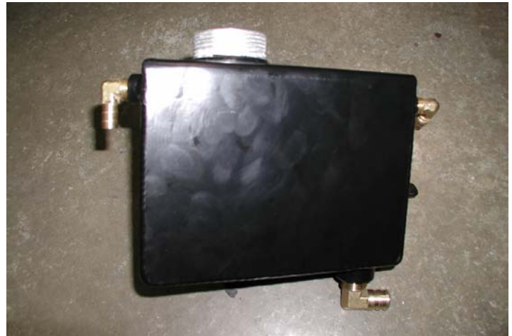
Coolant Reservoir Assembled
