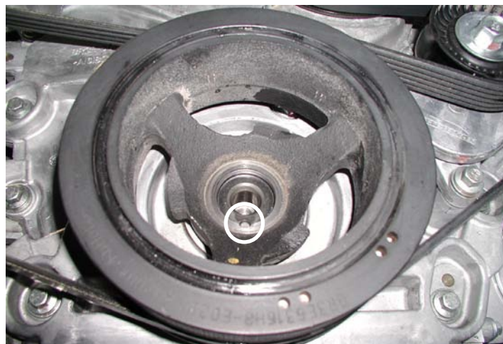
Install Crank Dowel Pin
