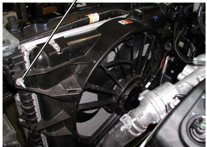
Remove Bolt (Driver's Side)
