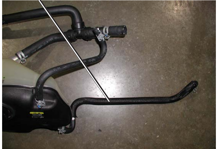
Remove Factory Radiator Overflow Hose
