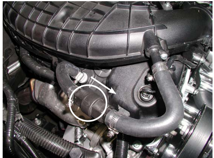
Check Valve Installed
