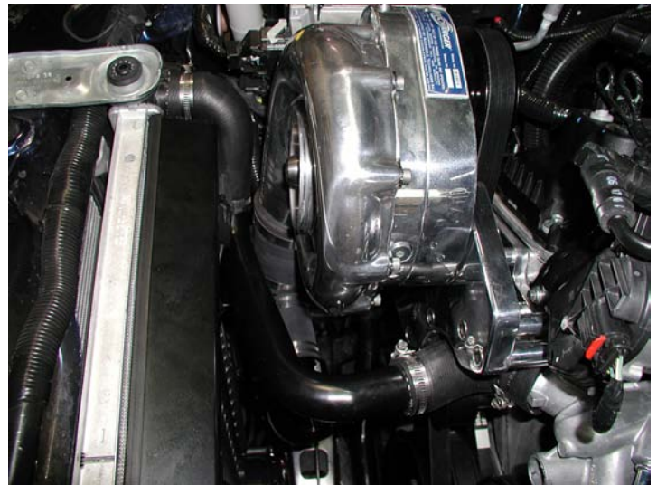
Upper Radiator Tube Installed
