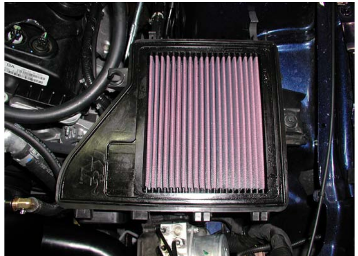
Factory Airbox and Air Filter Installed
