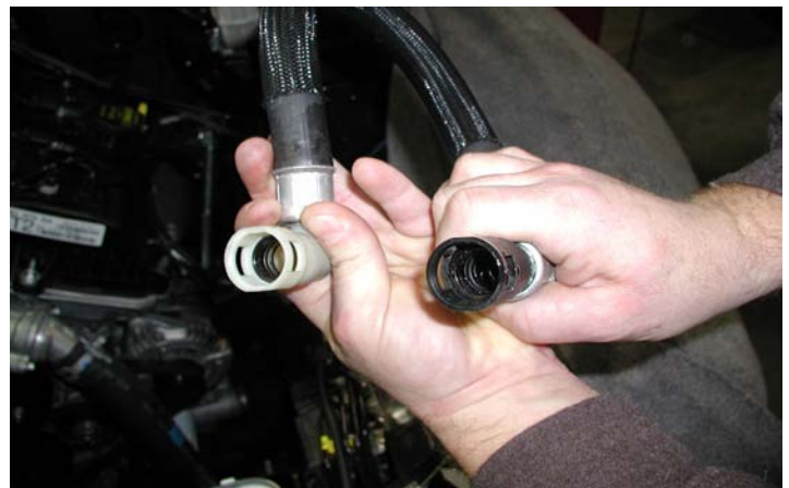
Firewall Heater Hose Connectors
