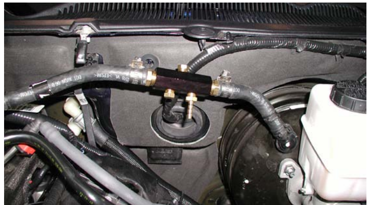
Vacuum Manifold Installation (Manual)
