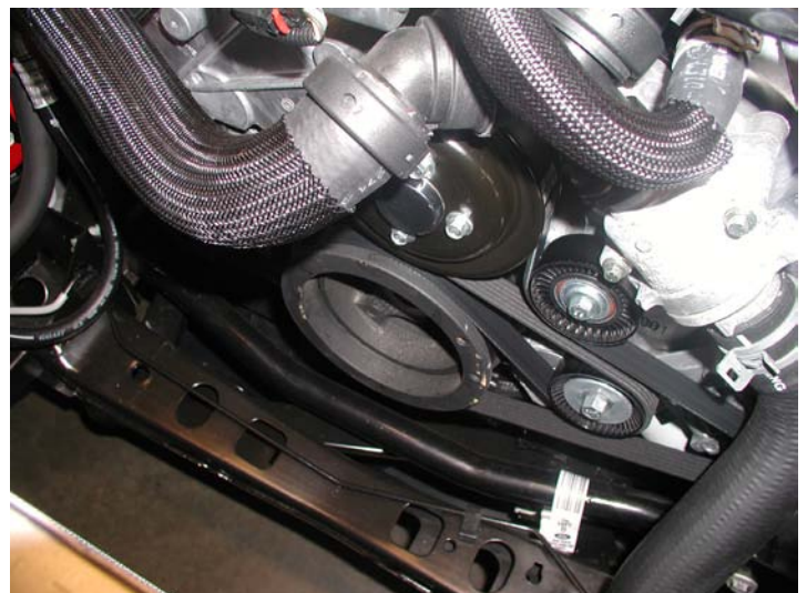
Remove Factory Balancer Bolt
