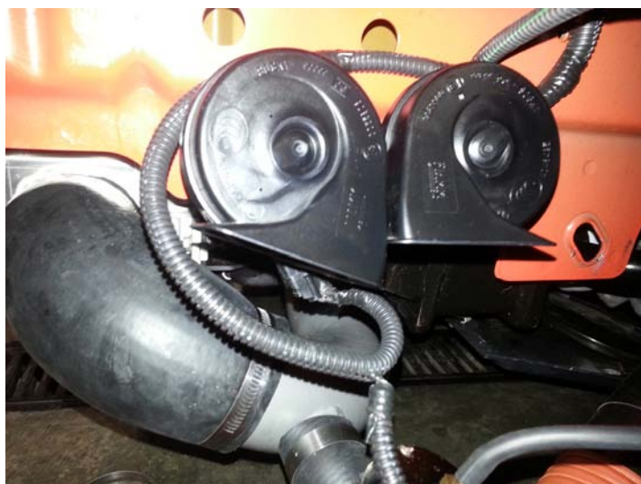
Surge Tube Installed and Horns Relocated
