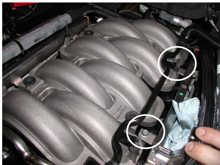
Remove Fuel Rail Mounting Bolts (4x)
