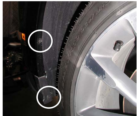
Remove Inner Fender Well Screws (Driver's Side Shown)
