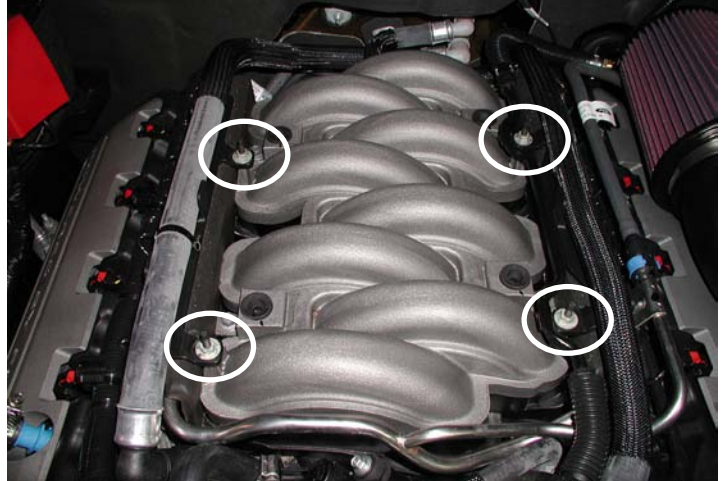
Remove Fuel Rail Insulation Nuts (4x)
