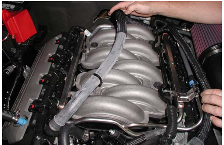
Adjust Coolant Lines For Fuel Rail Removal
