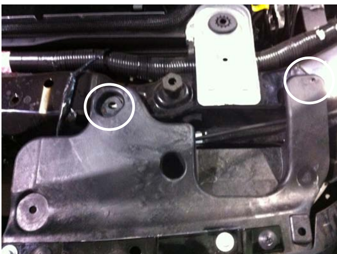
Upper Bumper Cover Bolts (2013-14) (viewed from above the vehicle)
