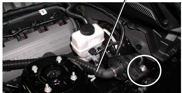
Fastener For Inlet Line Running To Driver's Side Firewall
