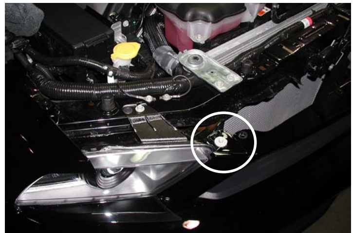
Remove Top Bumper Cover Bolts (Passenger's Side Shown)
