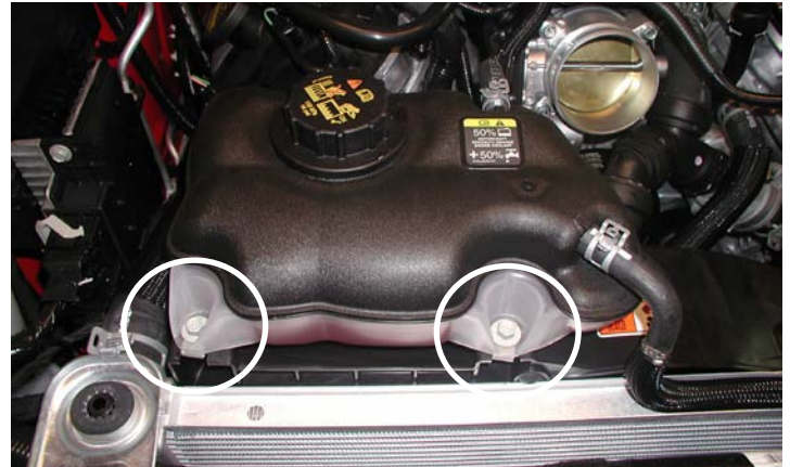
Remove Overflow Tank Bolts (2X)
