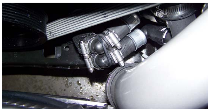
Boss 302 Only Oil Cooler Line Positioning
