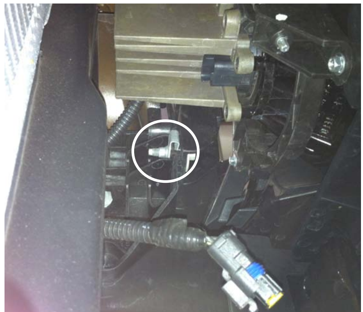
Inner Bumper Cover Bolts (2013-14) (viewed from beneath the vehicle)
