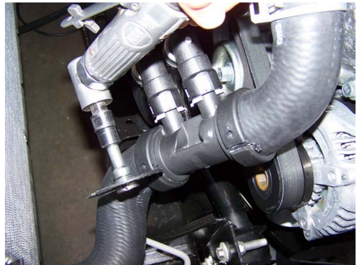
Cut Plastic Ring Clamps on Lower Radiator
