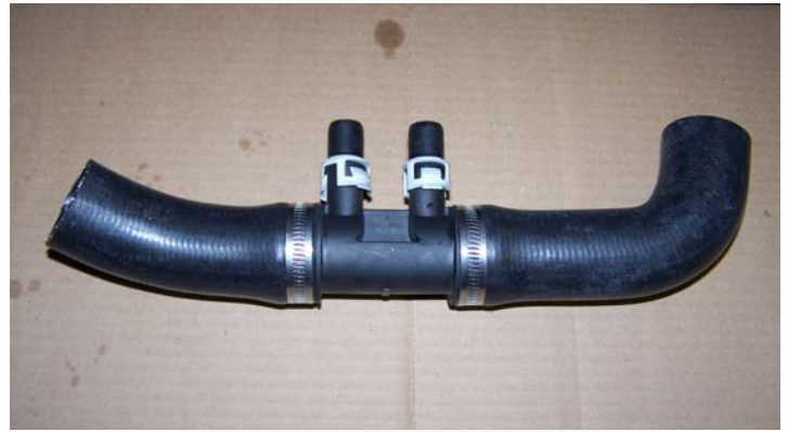
Assemble Lower Radiator Hose
