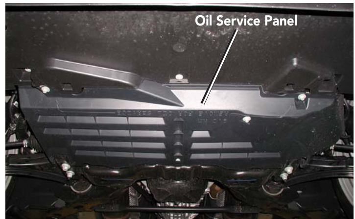
Remove Oil Service Panel Fasteners
