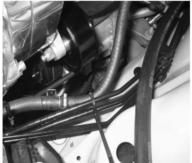
P/S Hose to Idler Clearance
