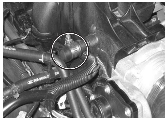
3/8" Vacuum Cap Installation
