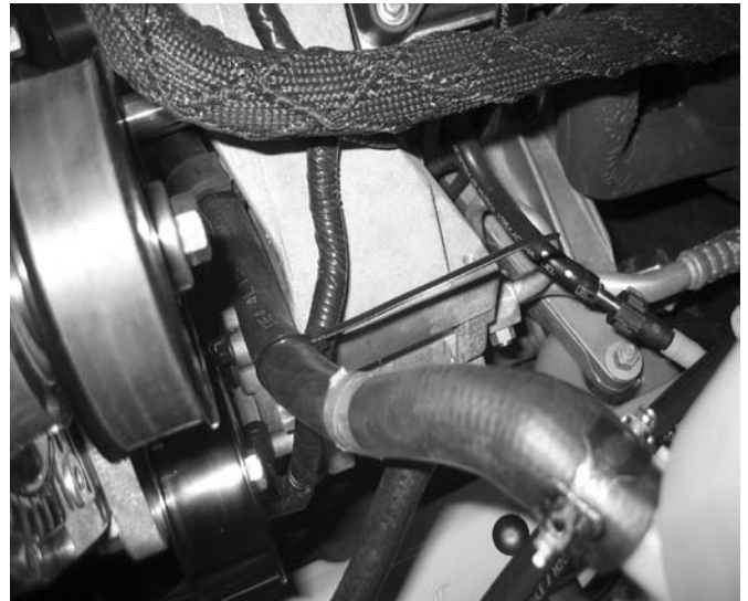
P/S Hose to Idler Clearance
