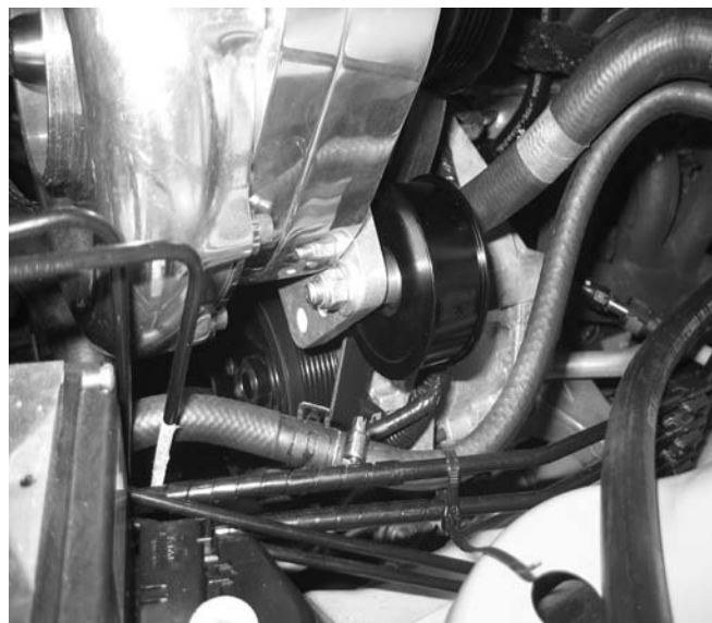
Fixed Idler Installation
