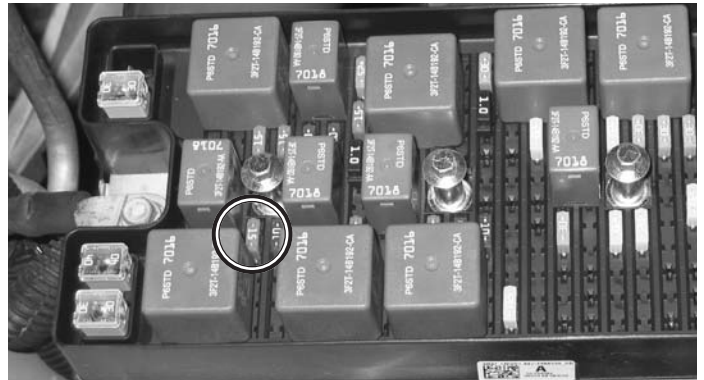
Fuel Pump Fuse Removal #41 Fuel Pump Fuse (Blue 15 Amp Mini Fuse)
