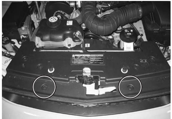
Radiator Cover Removal
