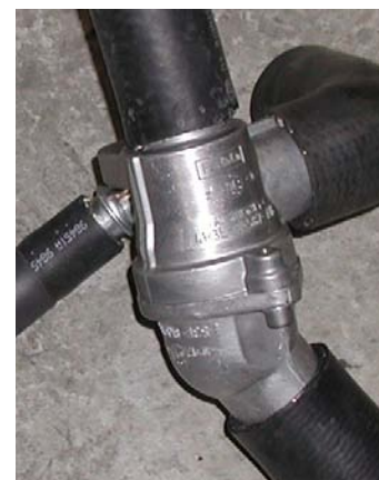
Thermostat Housing Reconfigured
