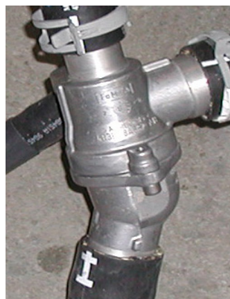
Thermostat Housing Reconfigured
