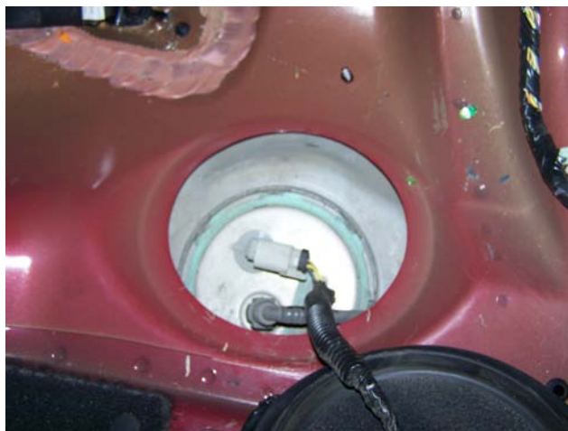
Fuel Pump Module Removal Below the Driver's Side Rear Seat
