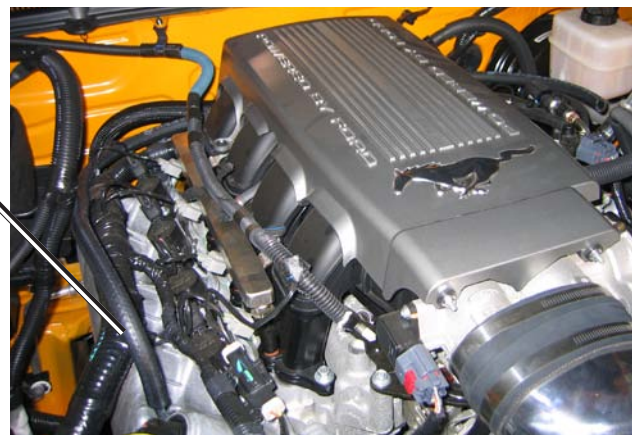
PCV Hose Installed on the Passenger's Side Valve Cover
