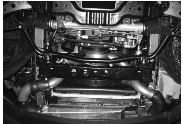
Intercooler & Tubing Viewed From Below
