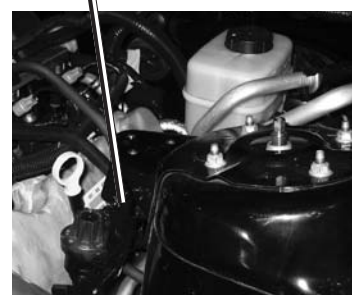
Vapor Control Bracket (Relocated to bottom of Original Mount)
