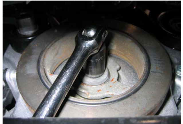
Removing the Crank Pulley Bolt
