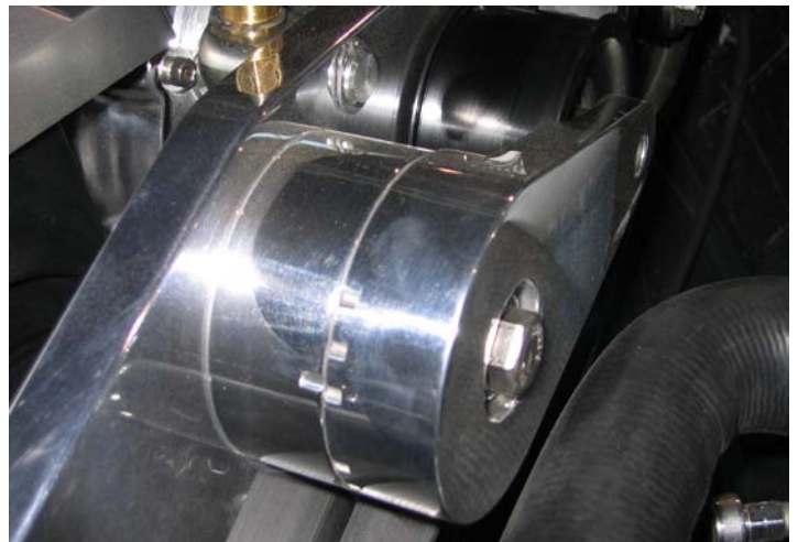
Belt Tensioner Alignment Marks
