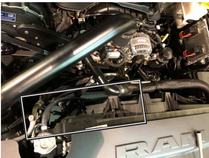
Overflow Hose Installed
