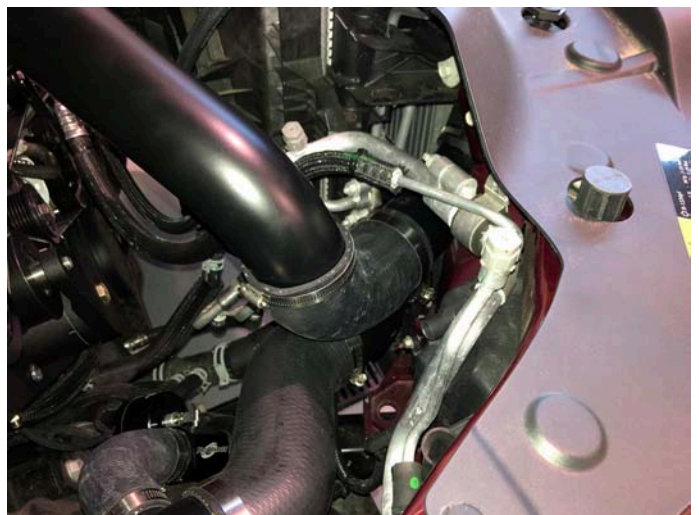
Tube #030 & 90° Rubber Elbow Installed
