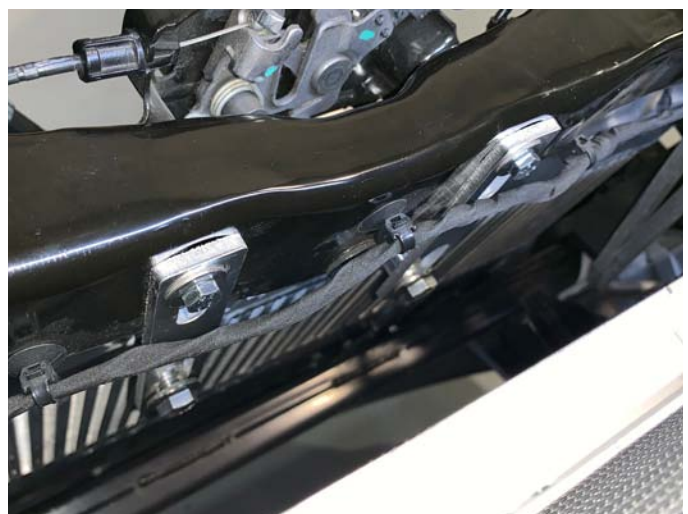
Upper Brackets Installed
