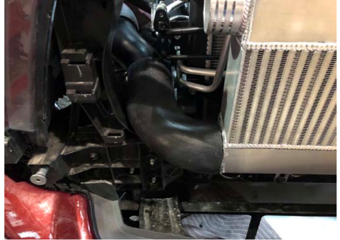
Tubing Into Intercooler
