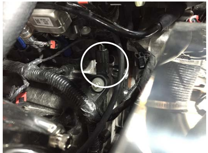
Ground Attached To Valve Cover
