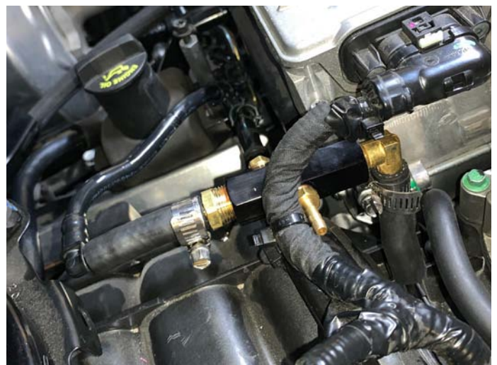
Vacuum Manifold Installed
