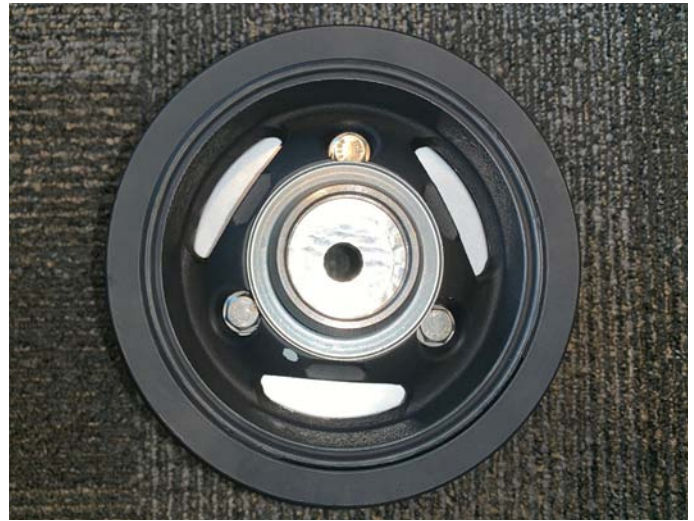
Crank Pulley Installed
