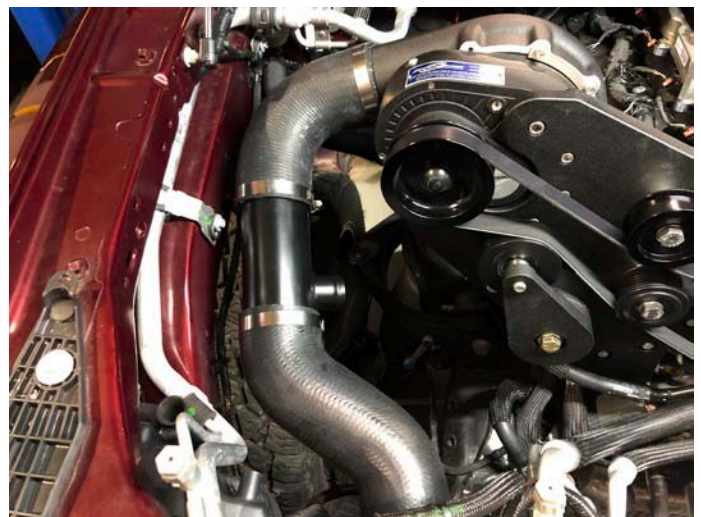
Tubing To Supercharger Installed
