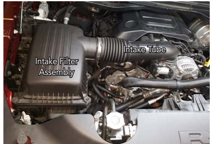
Intake Filter Assembly
