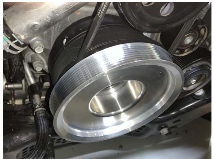
Crank Pulley Installed
