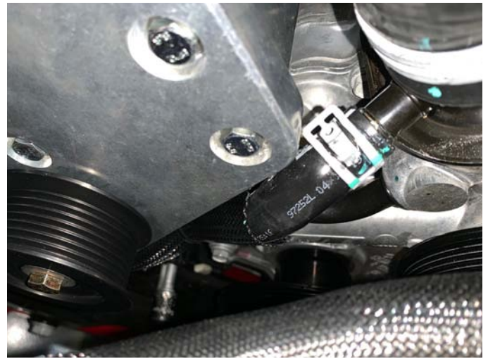
Zip Tie Coolant Hose
