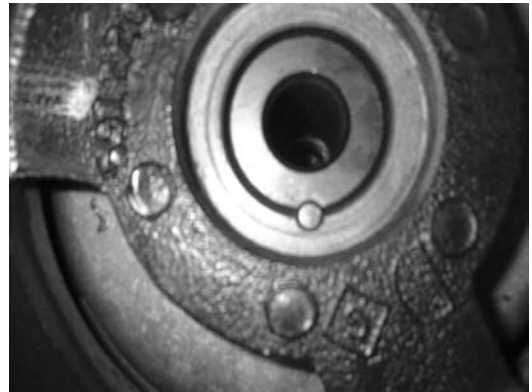
Crank Pulley Pinned to Crankshaft
