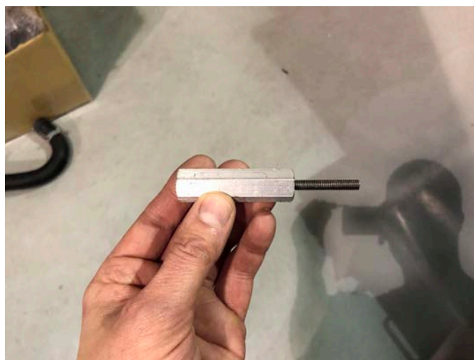
Stud Threaded Into Hex Spacer
