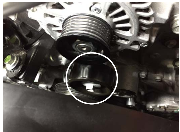
Idler Pulley Replaced
