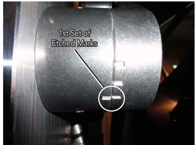
Proper Tensioner Position (View From Below)
