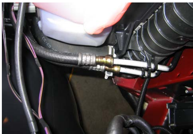
Main Water Line Clamps
