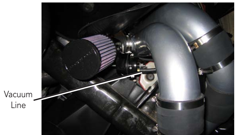
ProFlow Unit Installed
