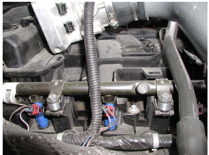
Fuel Rail Spacers Installed
