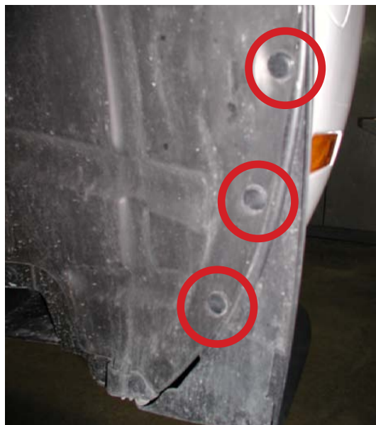
Lower Fascia Connections (Pass. Side)
