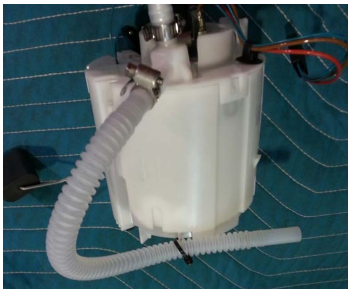
Suction Hose Attached to Basket
