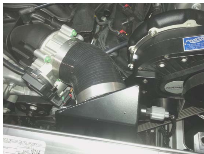
Throttle Body Tube Installed (6.4L Shown)
