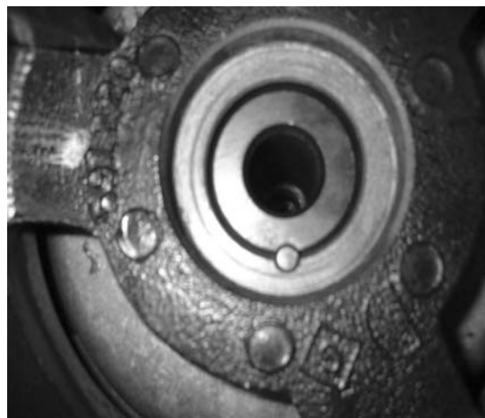
Crank Pulley Pinned to Crankshaft
