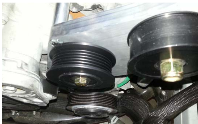
Ribbed Idler Installed
