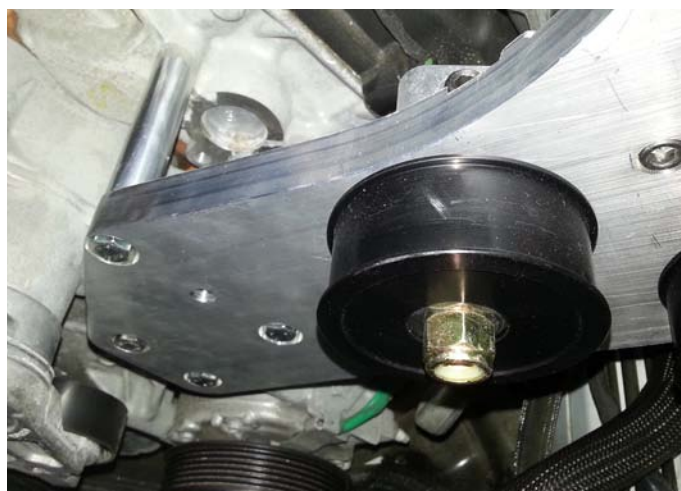
Main Bracket Installed
