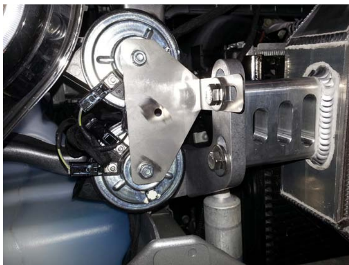
Pass. Side Intercooler & Horn Relocation
