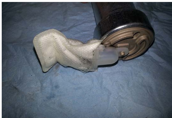
New Fuel Sock Installed
