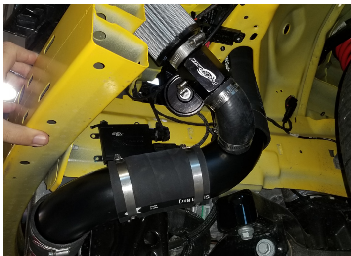
Race Intercooler Connection
