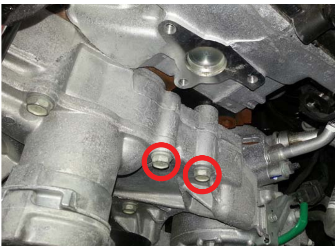
Remove Timing Cover Bolts
