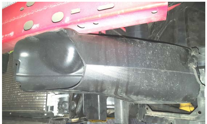
Remove Brake Duct
