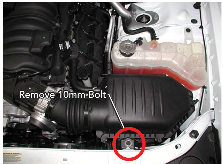
Remove Air Filter Assembly Bolt
