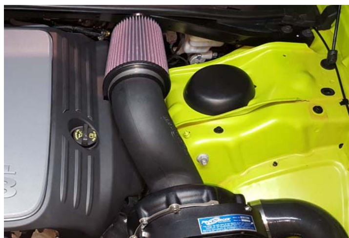
5.7L Cover Trimmed for Air Inlet
