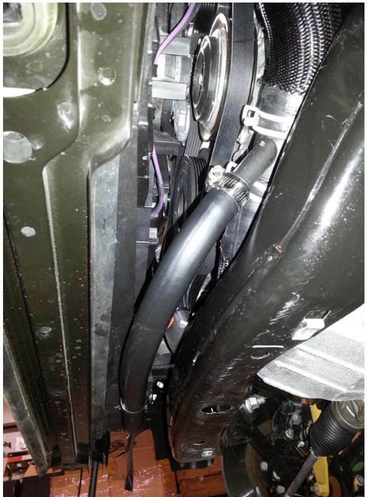
New Coolant Hose Routed (6.4L)
