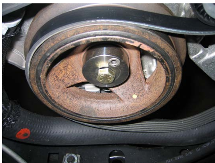
Drill Jig Installed
