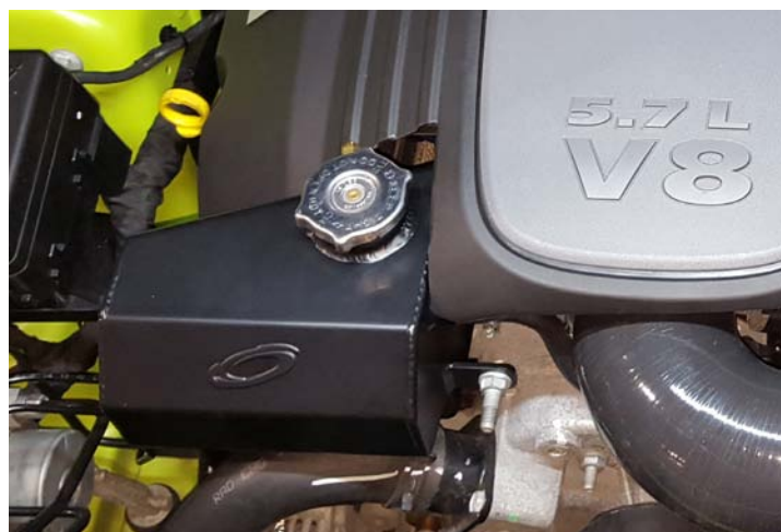
5.7L Cover Trimmed for Coolant Reservoir
