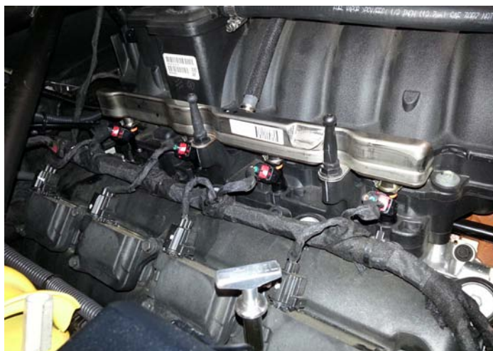
6.4L Models: Fuel Rails Installed
