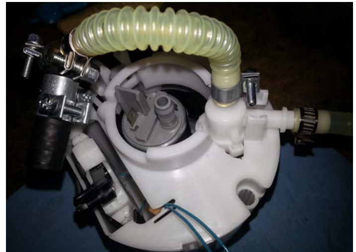
Jet Siphon Installed in Basket
