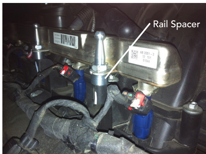
5.7L Models: Fuel Rails Installed
