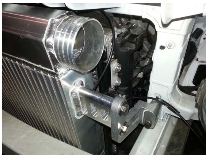
Driver's Side Intercooler Brackets
