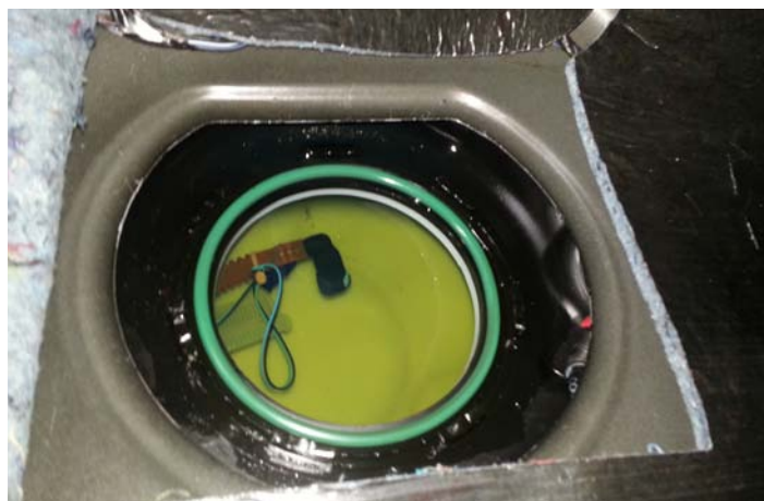
Fuel Pump Removed
