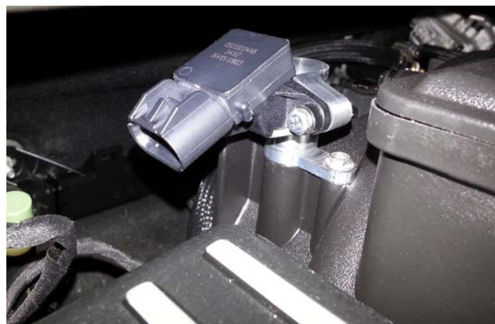
New 6.4 MAP Sensor Installed
