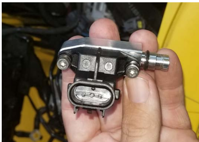
5.7 MAP Sensor Installed
