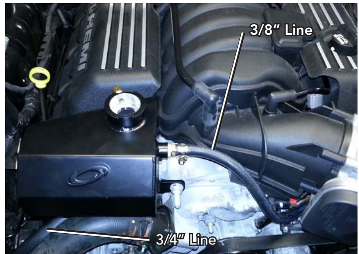
Coolant Hose Routing
