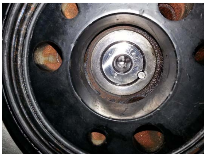
Crank Pulley Pinned to Crankshaft
