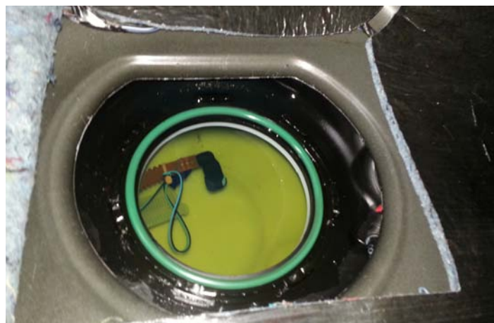
Fuel Pump Removed
