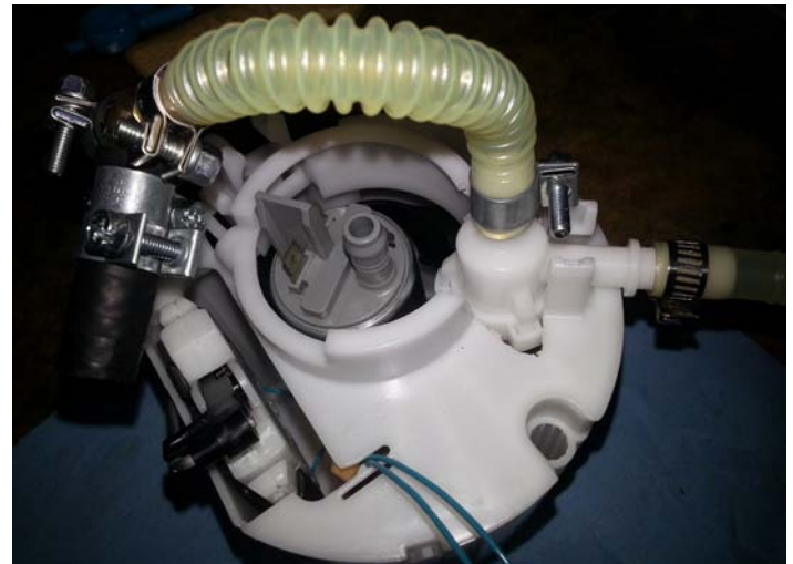
Jet Siphon Installed in Basket
