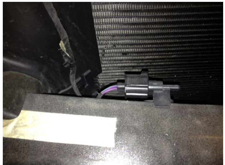
Air Temperature Sensor
