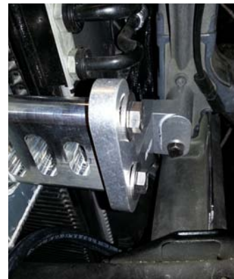
Passenger's/Driver's Intercooler Brackets
