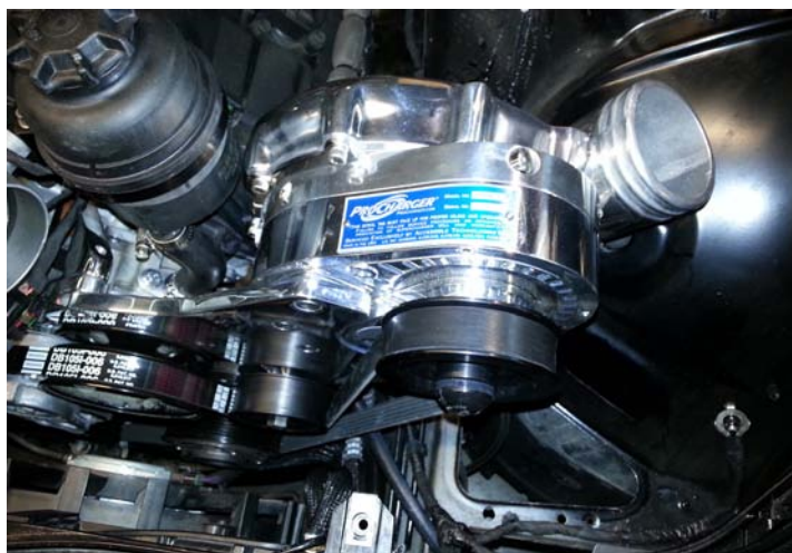
Procharger Head Unit Installed
