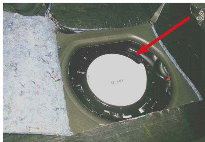
Fuel Pump Locking Ring
