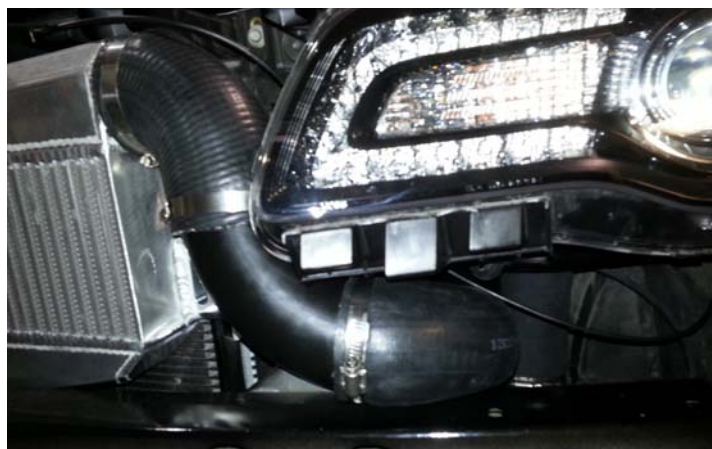
Upper Intercooler Tubing
