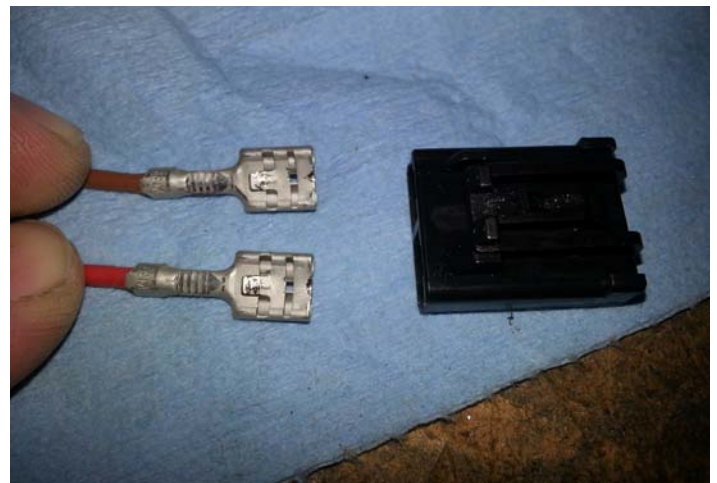
Spade Connectors Removed
