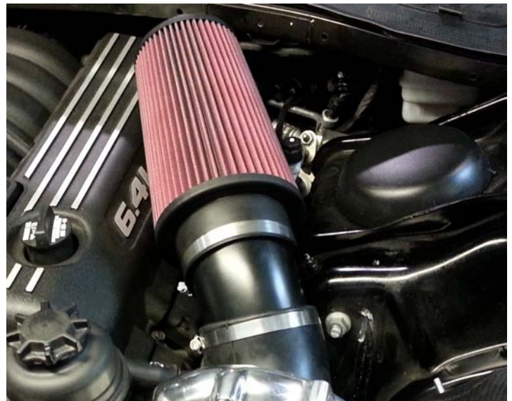
Air Inlet Assembly (No Upper Strut Brace)
