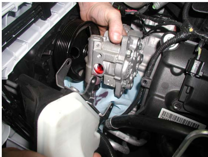
Power Steering Pump & Reservoir Separated
