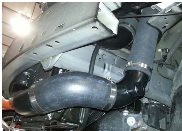
Lower Intercooler Tubing
