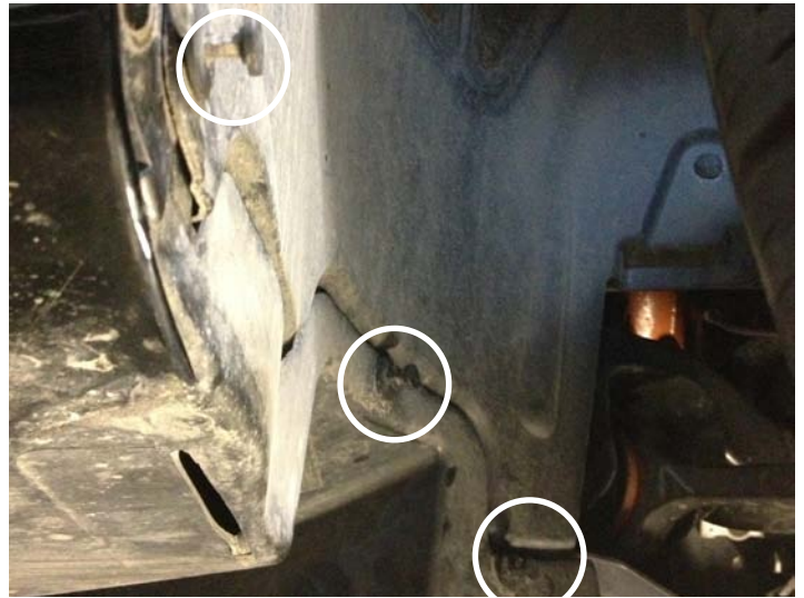
Front Fender Well Panel Fasteners
