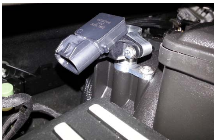
New MAP Sensor Installed
