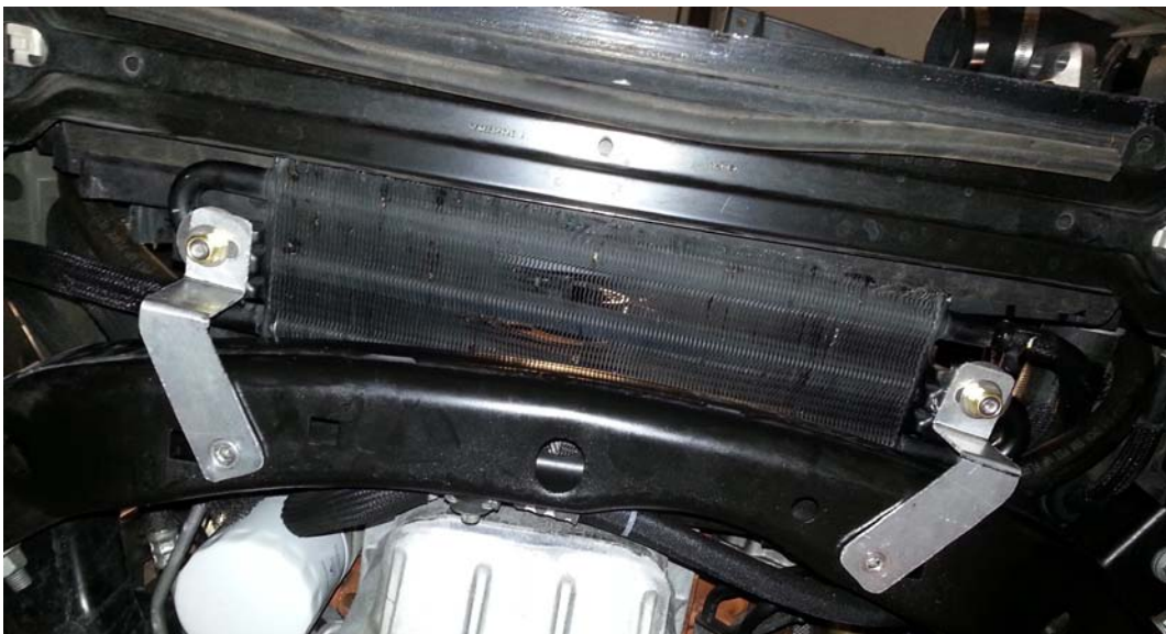
Relocated Power Steering Cooler
