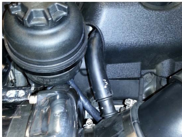
PCV Line Run To Air Inlet
