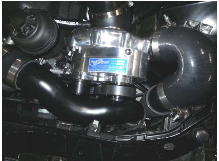
Blower Discharge Connection
