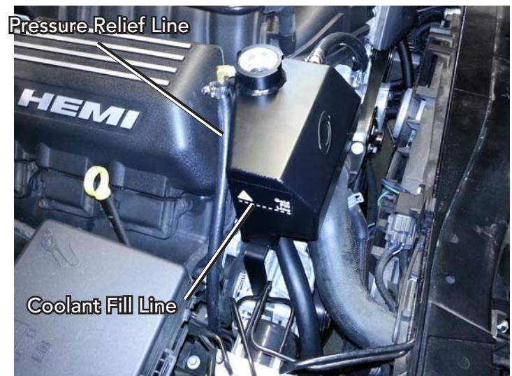
Pressure Relief Line Routing &amp; Fill Line
