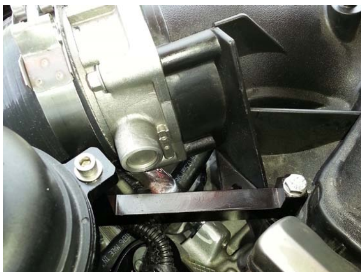
Lower Reservoir Bracket Mounting Location
