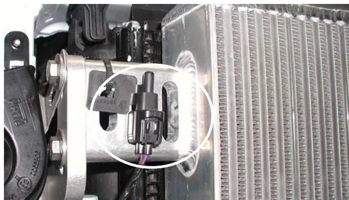
Ambient Air Temp Sensor Mounted
