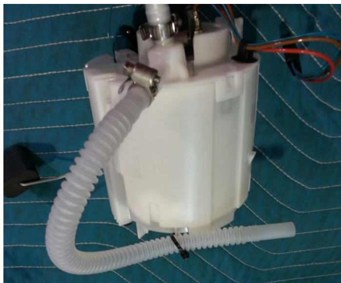
Suction Hose Attached to Basket
