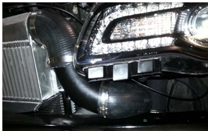
Upper Intercooler Tubing
