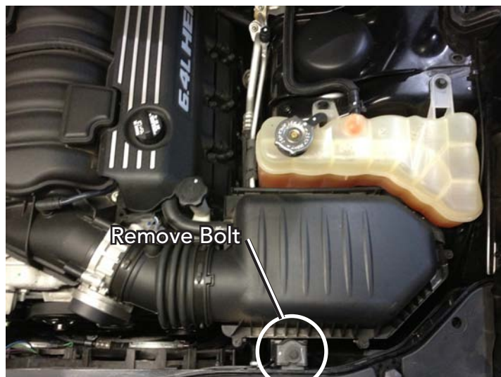
Remove Air Filter Assembly Bolt
