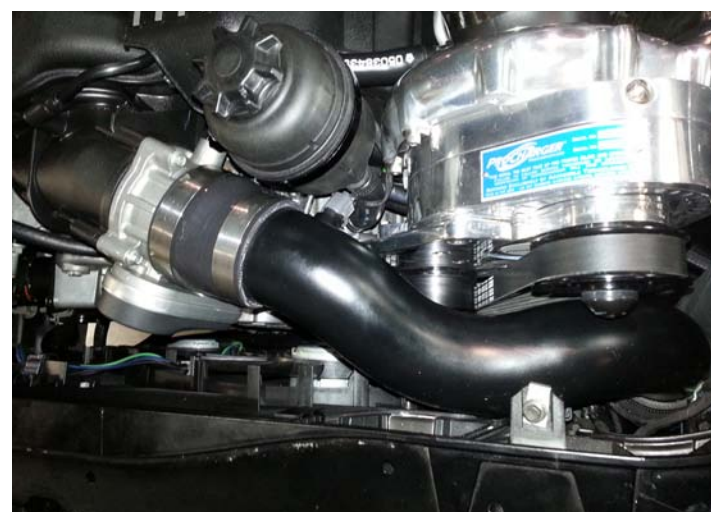
Throttle Body Tube Installed
