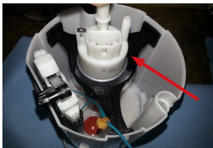
Fuel Pump Locking Tabs
