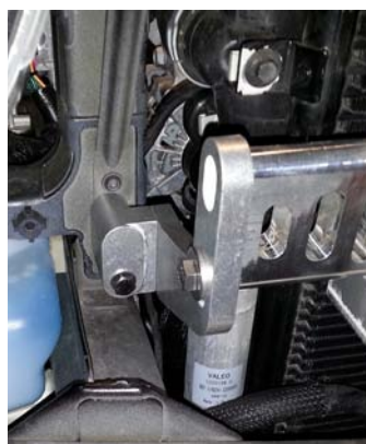
Passenger's/Driver's Intercooler Brackets
