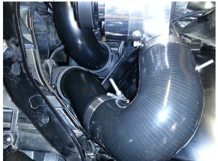
Blower Discharge Connection
