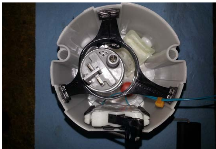
Fuel Pump Orientation
