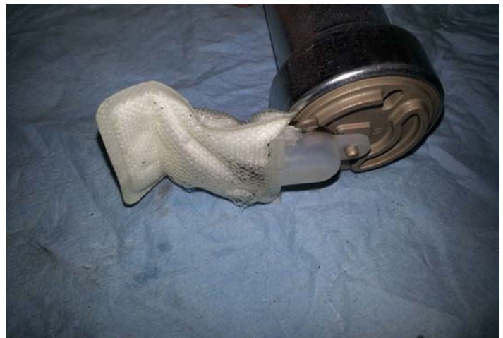
New Fuel Sock Installed
