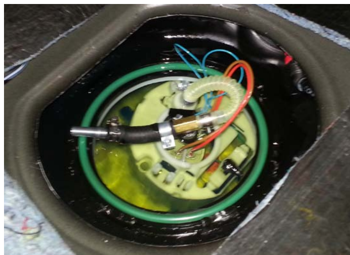
Pump Assembly Into Tank
