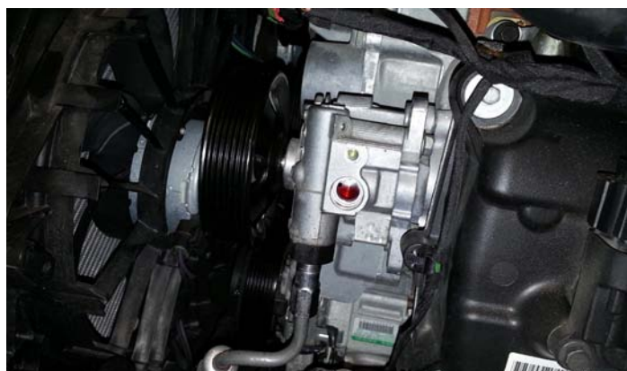
Power Steering Reservoir & Line Removed
