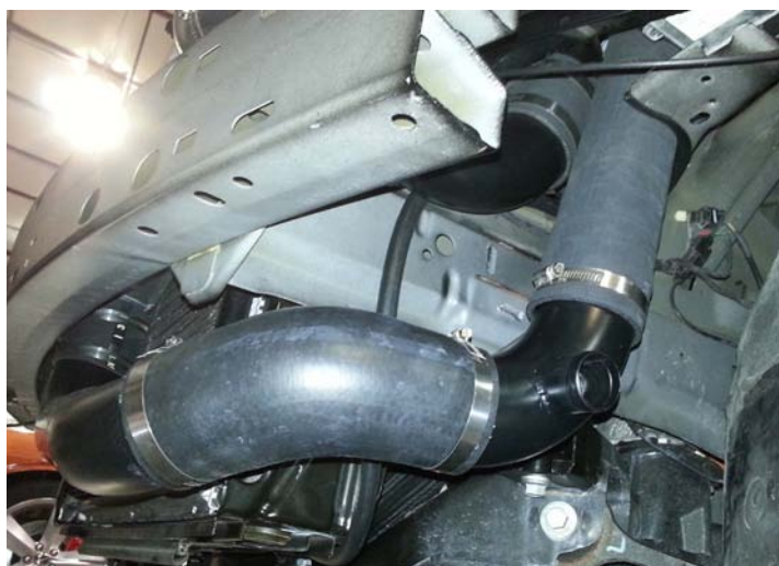
Lower Intercooler Tubing
