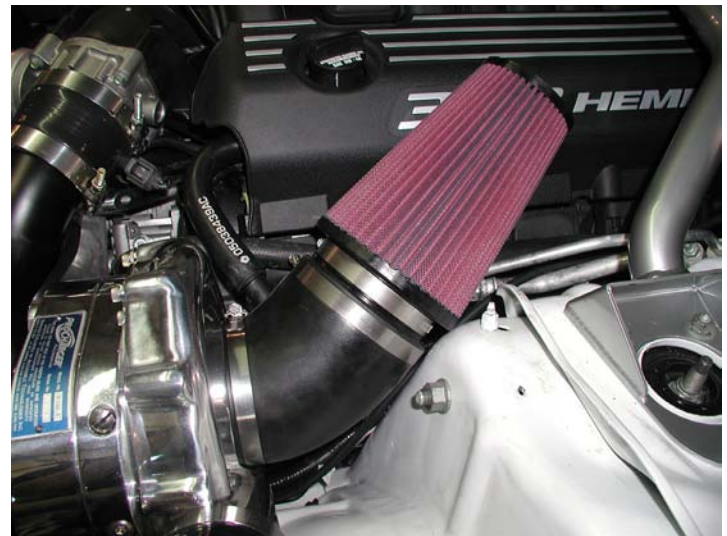
Air Inlet Assembly (With Upper Strut Brace)
