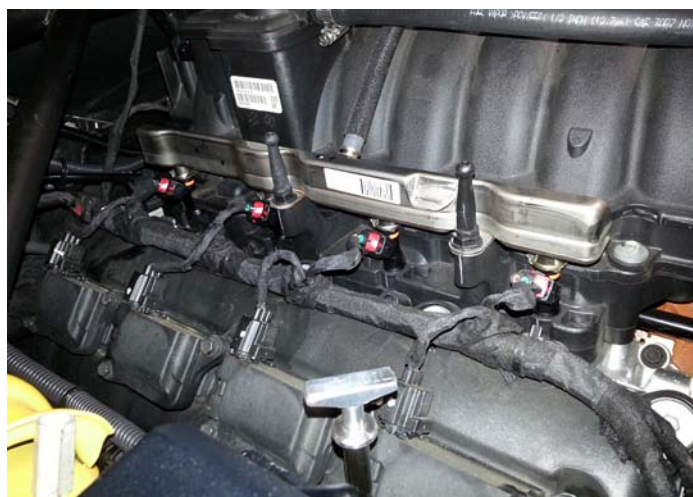
Fuel Rails Installed
