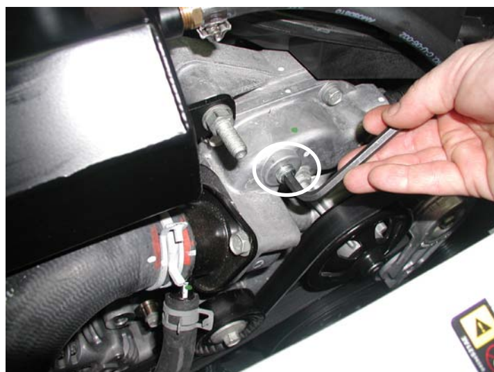
Cooling System Purge Screw
