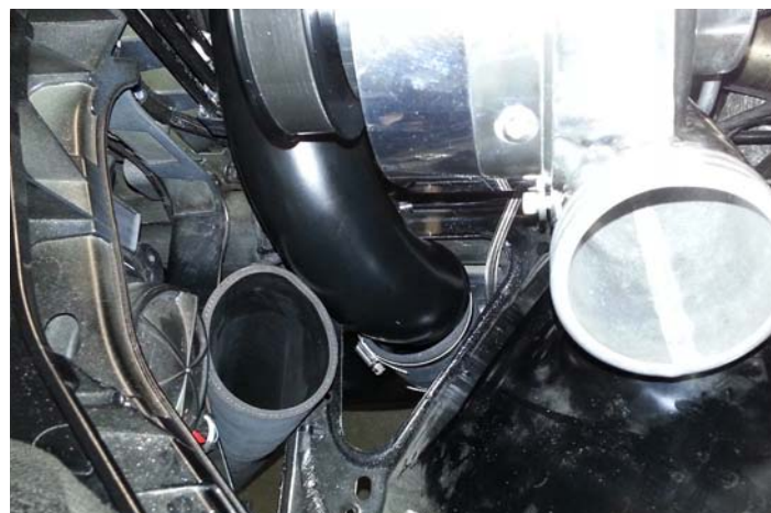
3" Rubber Tube Beneath Headlight
