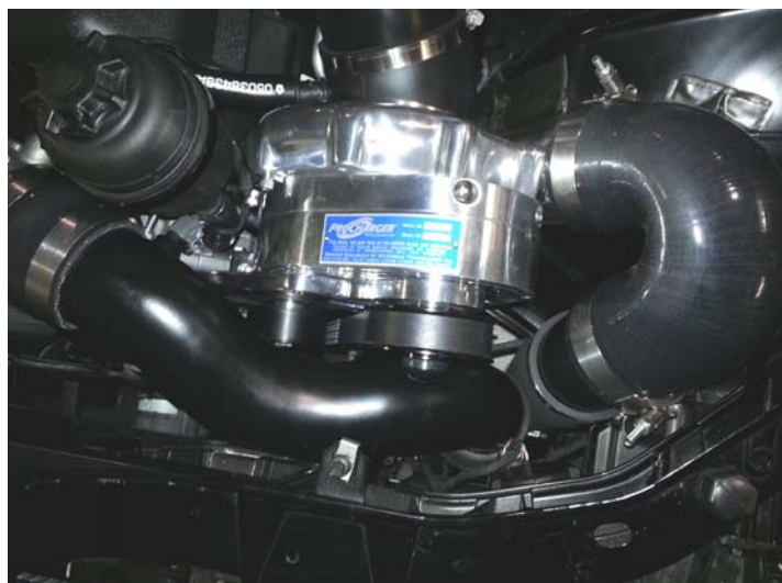
Blower Discharge Connection
