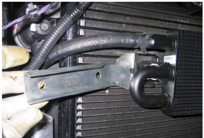
Power Steering Cooler Removal
