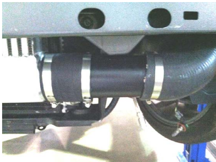
Lower Intercooler Tubing
