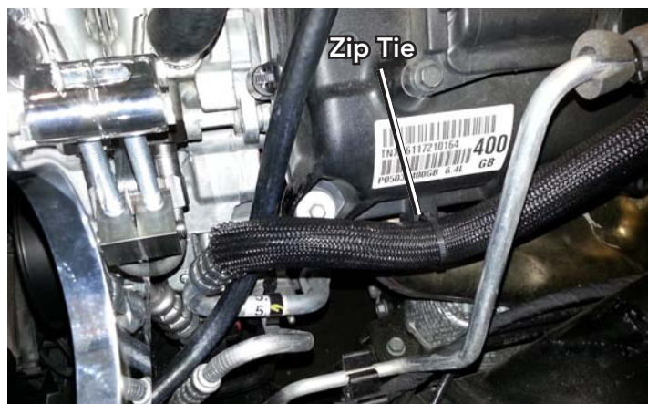
A/C Line Zip Tied to Valve Cover
