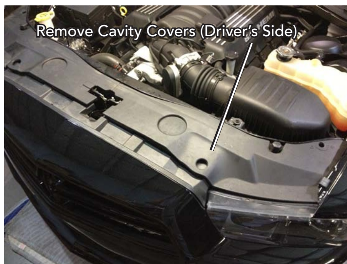
Radiator Cavity Cover(s)
