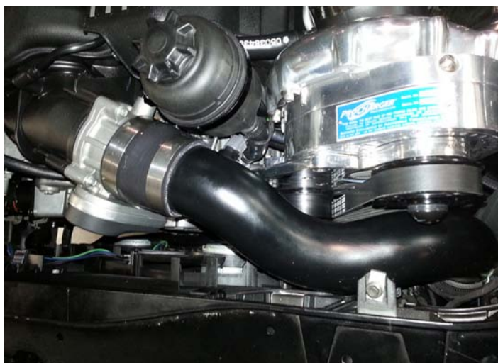
Throttle Body Tube Installed
