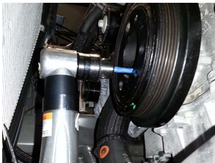
Drilling the Crank
