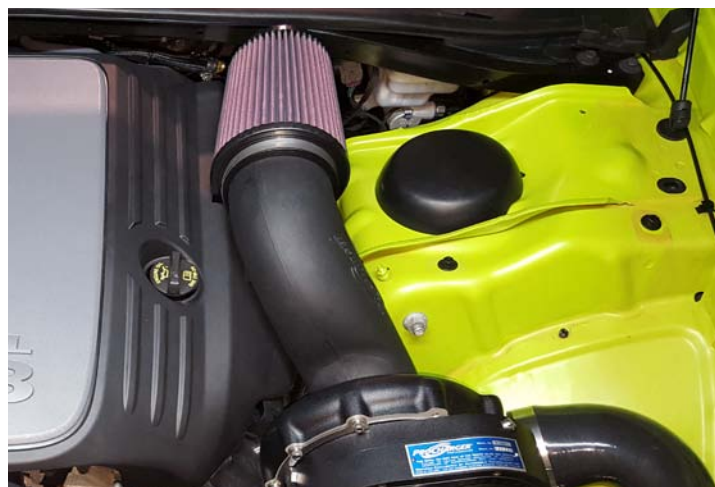
5.7L Cover Trimmed for Air Inlet
