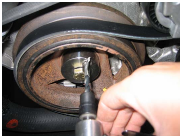
Drilling the Crank
