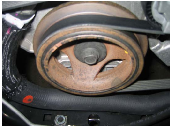
Factory Crank Pulley and Bolt
