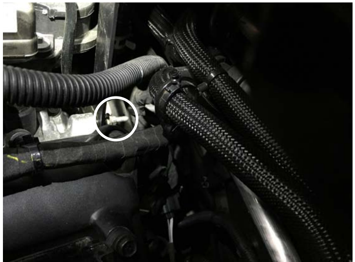
Remove Rear Braket Bolts (Drivers Side 6.4L Shown)
