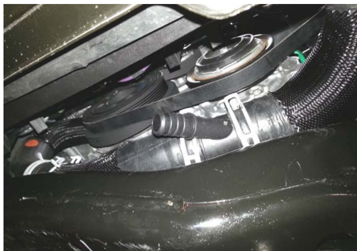
Coolant Fitting Reversed (6.4L)
