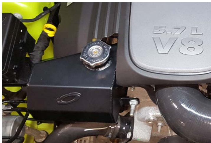
5.7L Cover Trimmed for Coolant Reservoir
