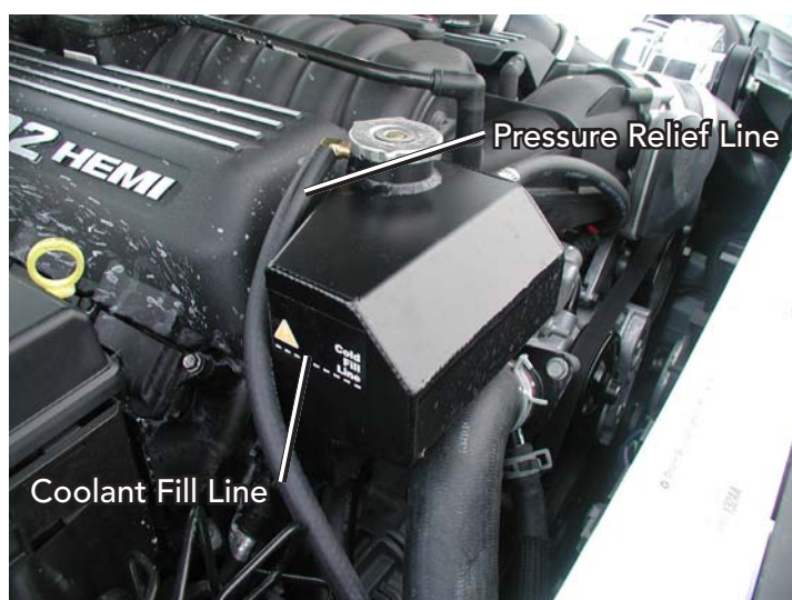
Pressure Relief Line Routing and Fill Line
