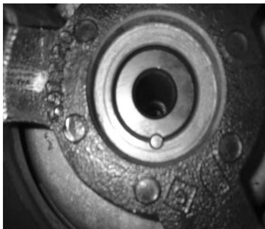
Crank Pulley Pinned to Crankshaft
