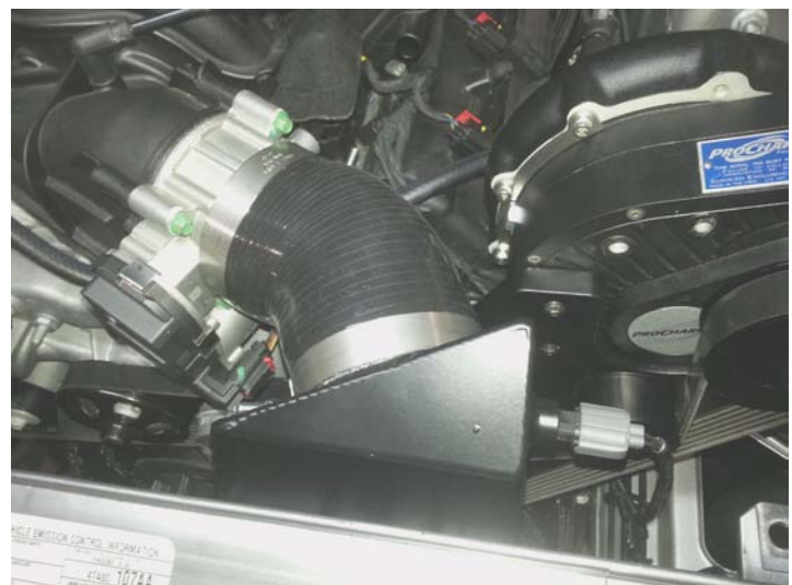
Throttle Body Tube Installed (6.4L Shown)
