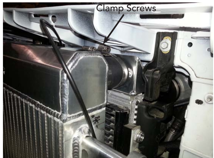
Air Plenum Connected to Intercooler
