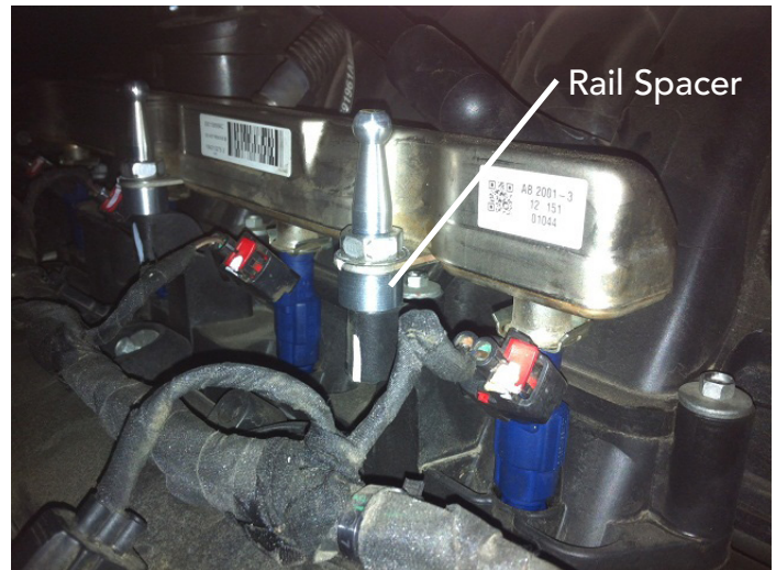
5.7L Models: Fuel Rails Installed
