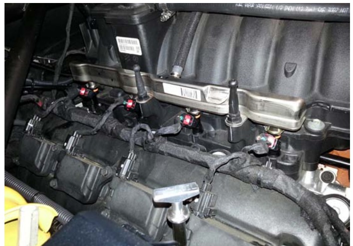
6.4L Models: Fuel Rails Installed
