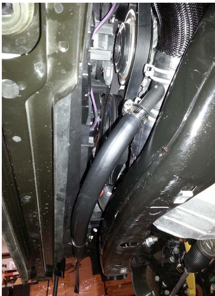
New Coolant Hose Routed (6.4L)
