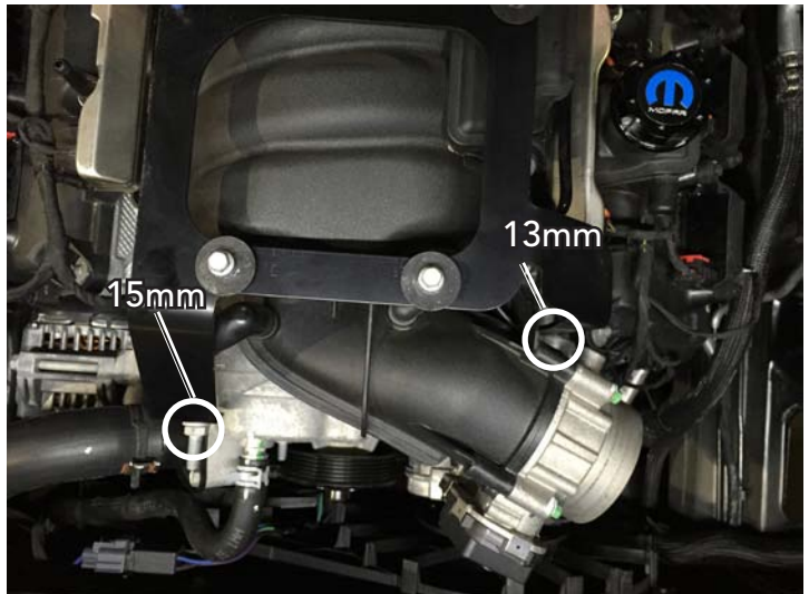
Remove Braket Bolts (6.4 shown)
