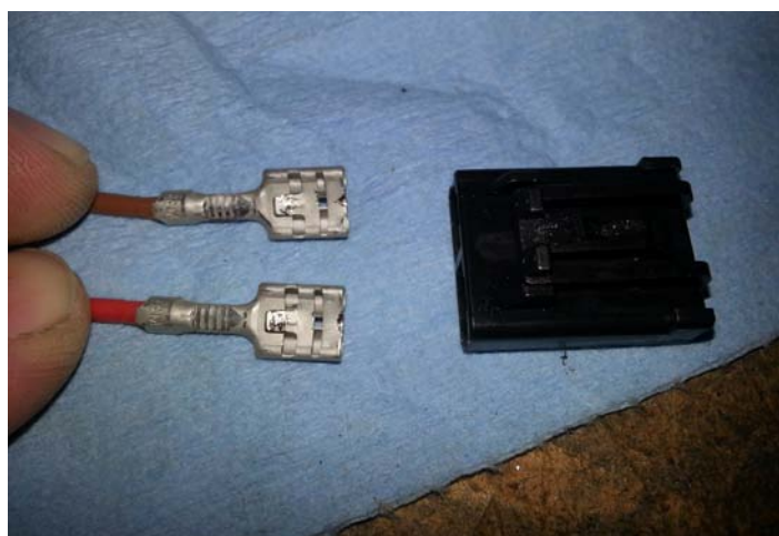
Spade Connectors Removed
