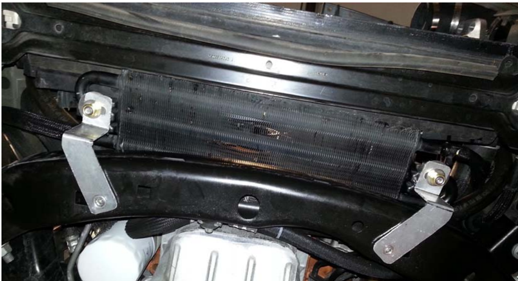
Relocated Power Steering Cooler
