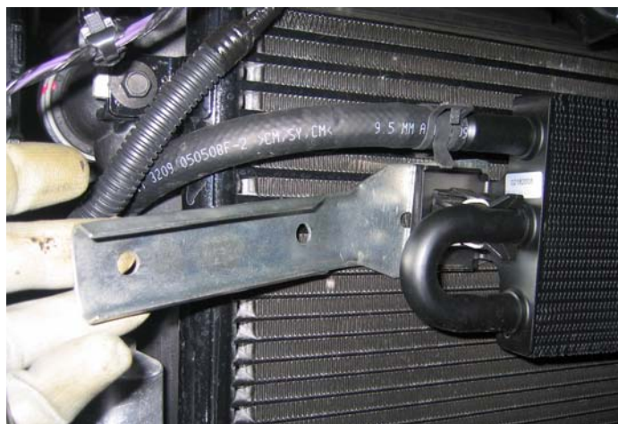
Power Steering Cooler Removal
