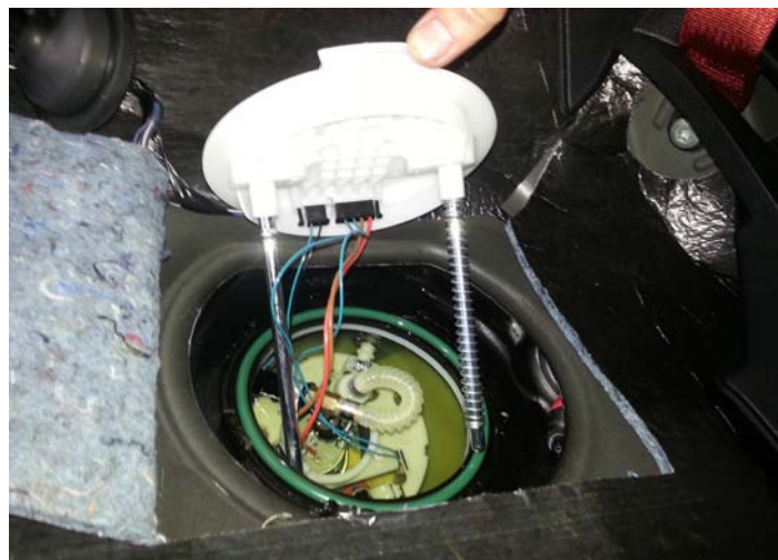
Electrical Connectors Under Pump Lid
