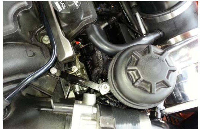
PCV Line Run To Air Inlet
