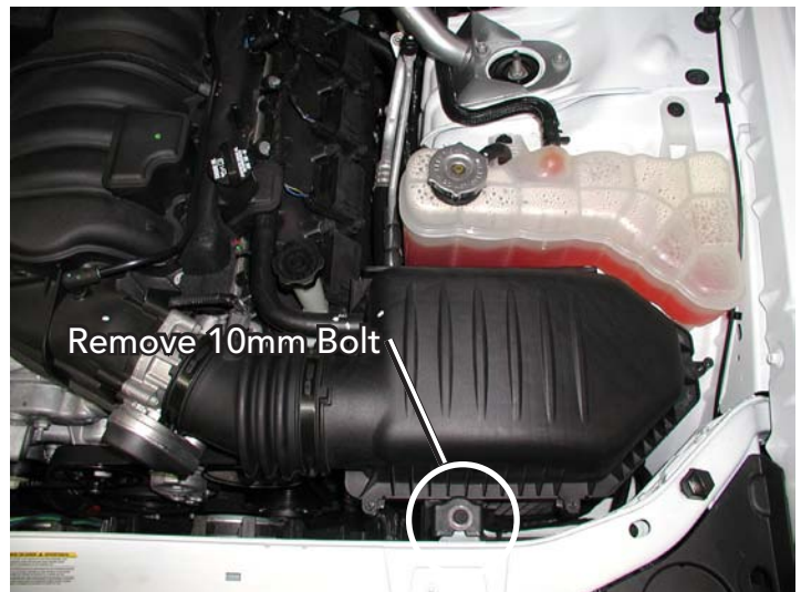
Remove Air Filter Assembly Bolt
