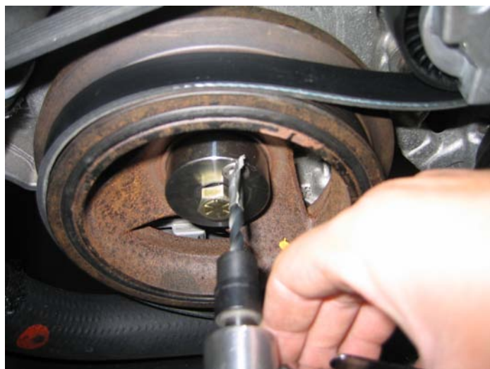
Drilling the Crank
