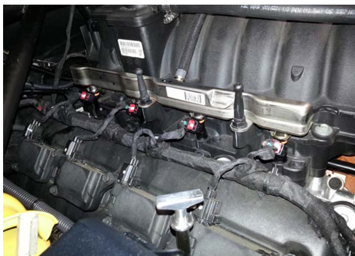
Fuel Rails Installed
