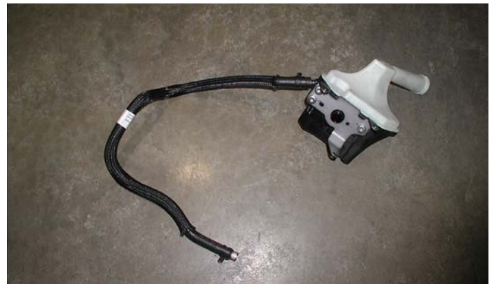
Power Steering Reservoir & Line Removed
