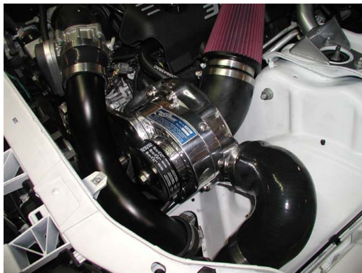
Throttle Body Tube (#315) Installed
