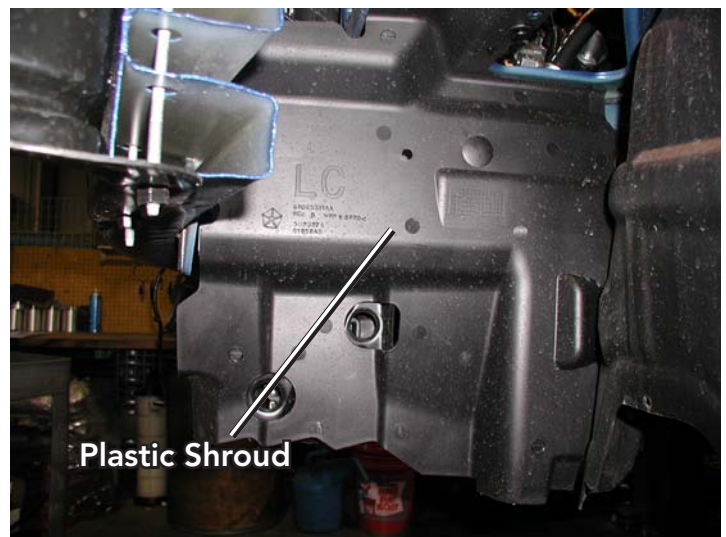
Driver's Side Plastic Shroud Removal
