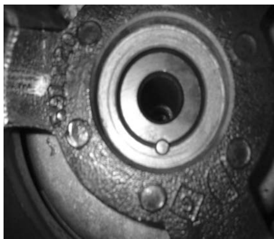
Crank Pulley Pinned to Crankshaft
