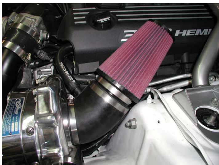
Air Inlet Assembly (With Upper Strut Brace)
