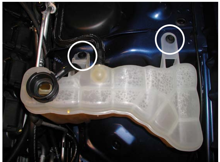
Remove Coolant Reservoir Bolts
