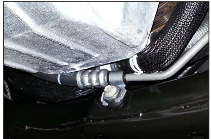
Power Steering Line Bracket's New Location
