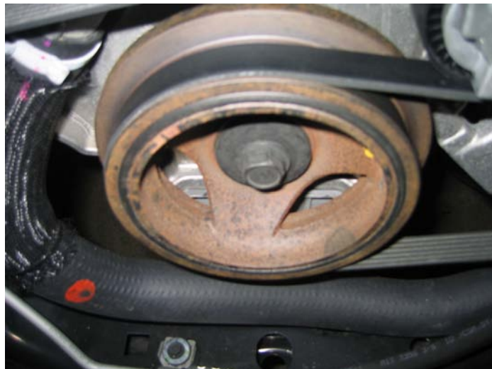
Factory Crank Pulley and Bolt
