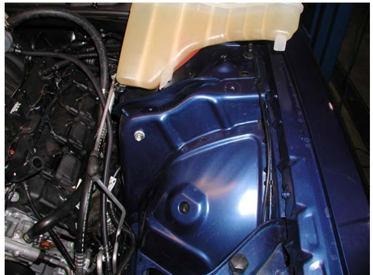
Lift Reservoir Out of Way
