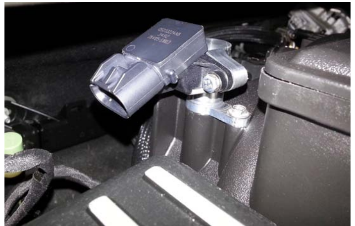
New MAP Sensor Installed
