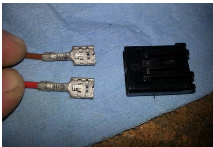
Spade Connectors Removed
