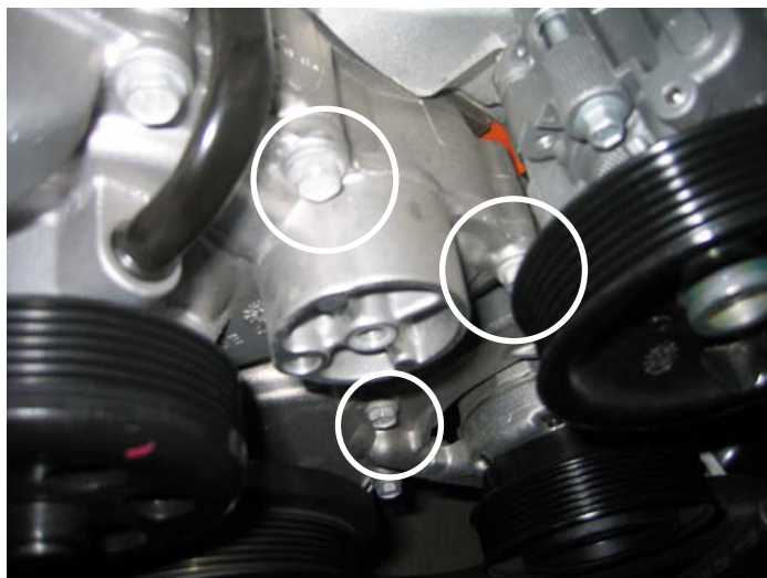
Remove 13mm Bolts For Sub-Bracket Install
