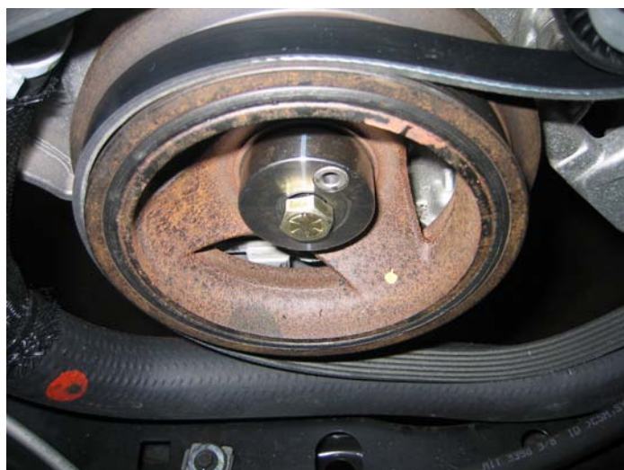
Drill Jig Installed
