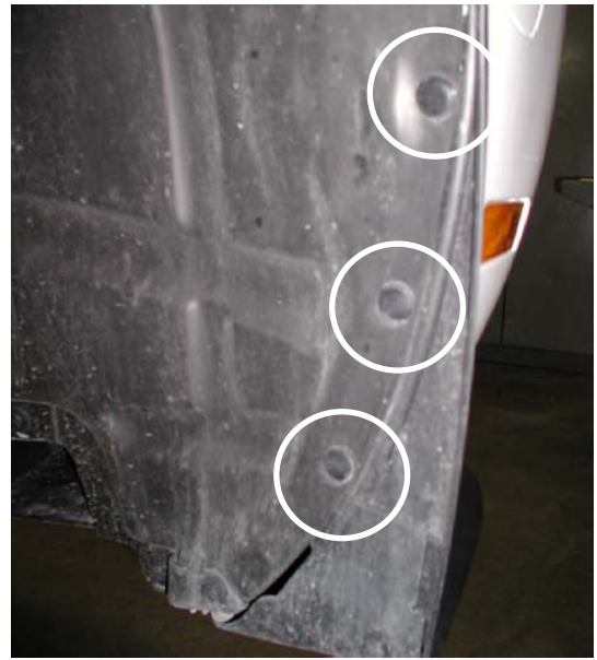
Lower Fascia Connections (Pass. Side)
