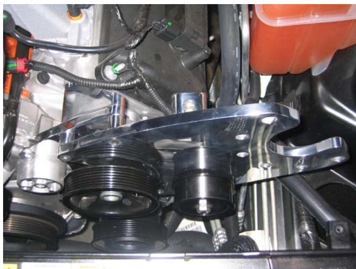
Main Bracket Installed
