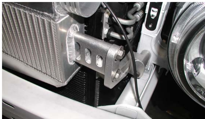
Driver's Side Intercooler Brackets
