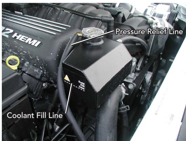
Pressure Relief Line Routing and Fill Line
