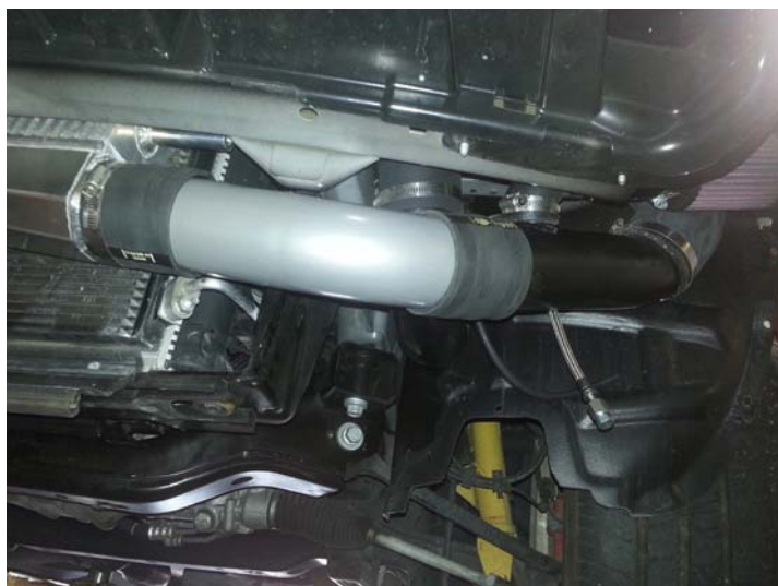
Race Intercooler Lower Tubing
