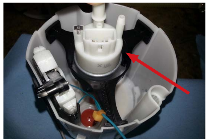
Fuel Pump Locking Tabs
