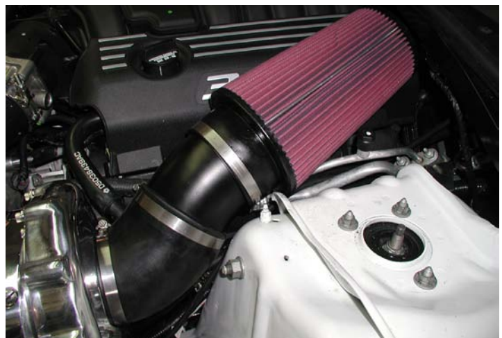
Air Inlet Assembly (No Upper Strut Brace)
