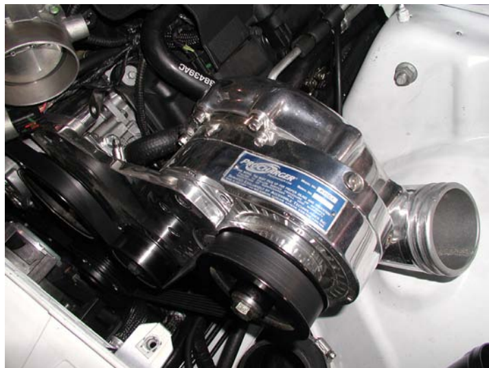
ProCharger Head Unit Installed
