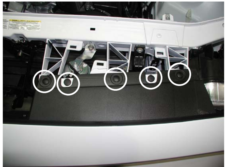
Top Fascia Connections (Driver's Side)
