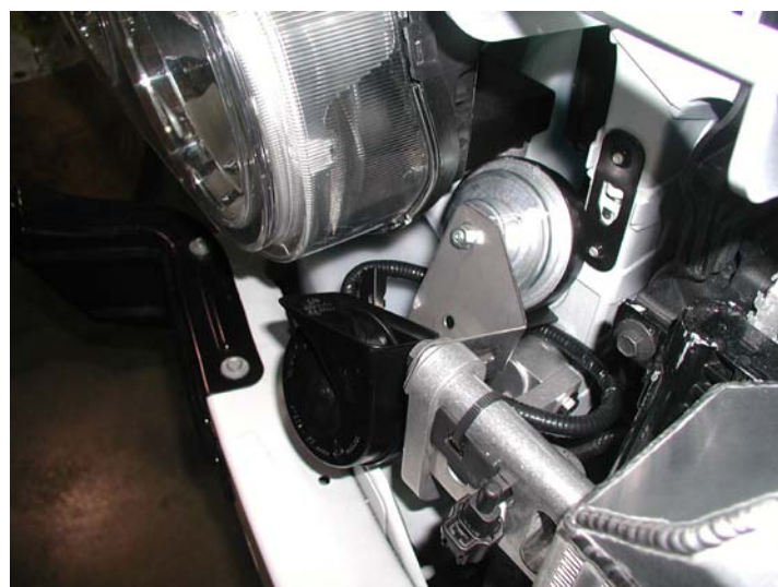
Pass. Side Intercooler & Horn Relocation
