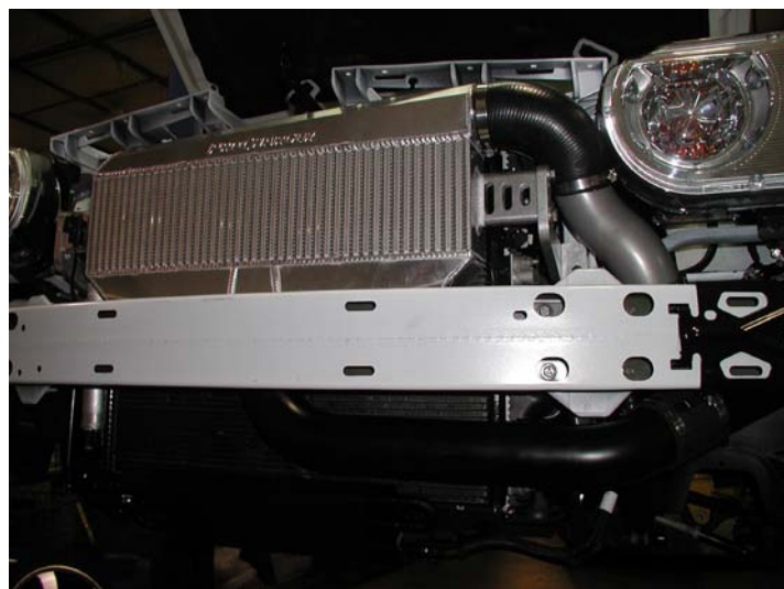
Stage 2 Intercooler and Tubing Installed
