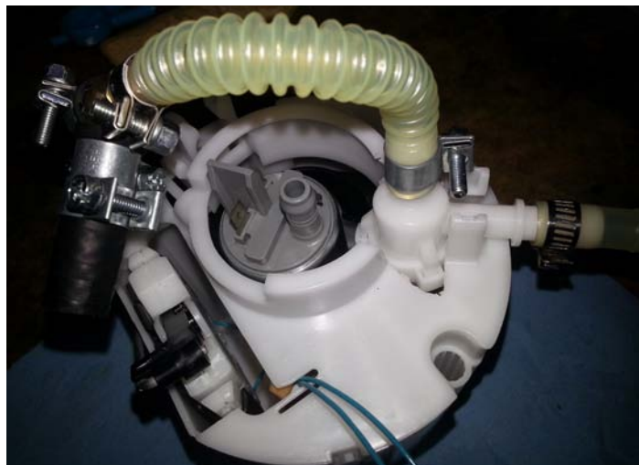
Jet Siphon Installed in Basket
