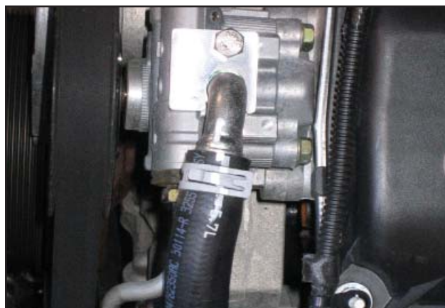
Power Steering Return Hose's New Position with Retaining Bracket
