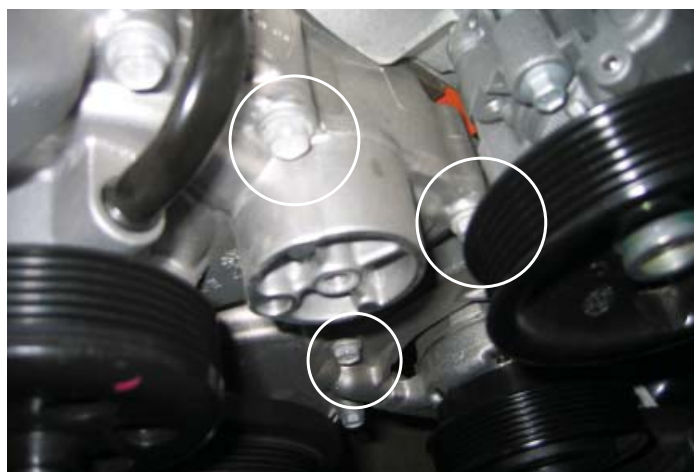
Remove 13mm Bolts For Bracket Install
