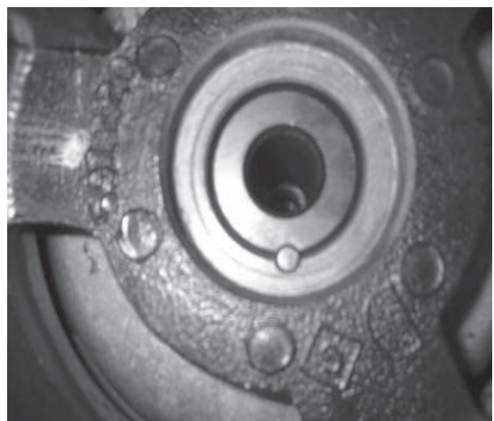
Crank Pulley Pinned to Crankshaft
