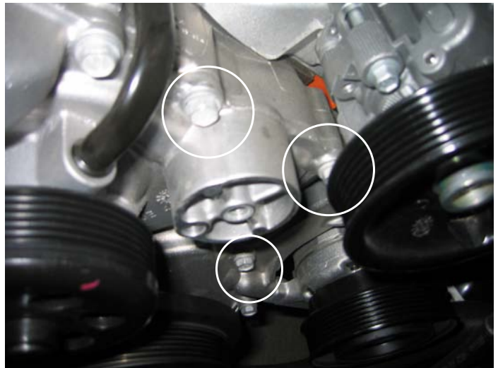
Remove 13mm Bolts For Sub-Bracket Install
