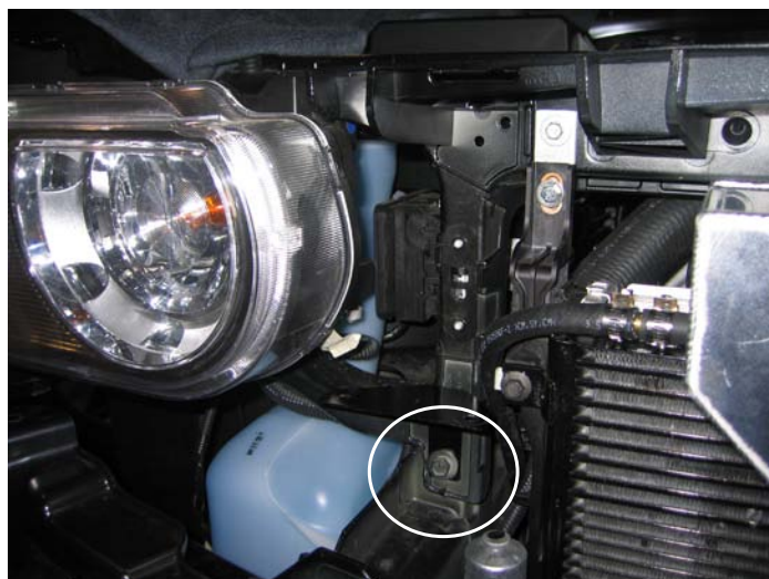
Frame Rail Bolt (For Horn Bracket Mounting)
