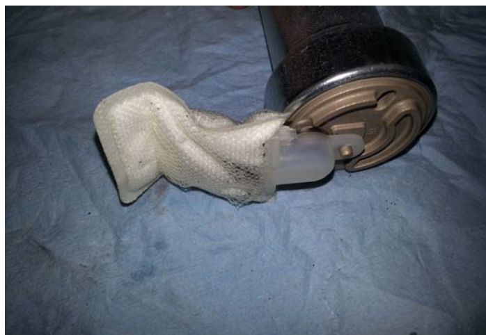
New Fuel Sock Installed
