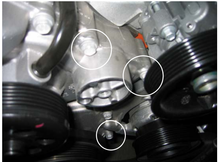
Remove 13mm Bolts For Sub-Bracket Install
