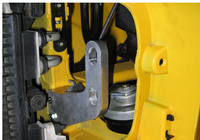
Driver's Side Intercooler Bracket Installed
