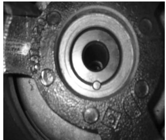
Crank Pulley Pinned to Crankshaft
