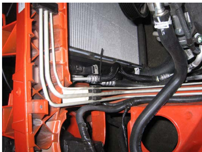
AC Lines Zip Tied Out of Way
