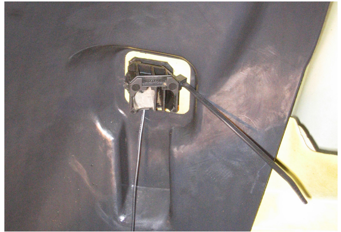
ABS Sensor Connector Zip Tied
