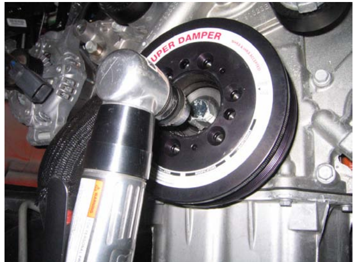
Drill Jig Installed/Drilling The Crank
