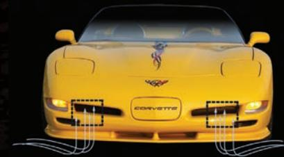
Exposing the intercooler to a constant supply of cool, incoming air is key to the heat removal process. Based on air inlet locations, ProCharger systems for C5's utilize an innovative Twin Highflow arrangement of two intercoolers.
